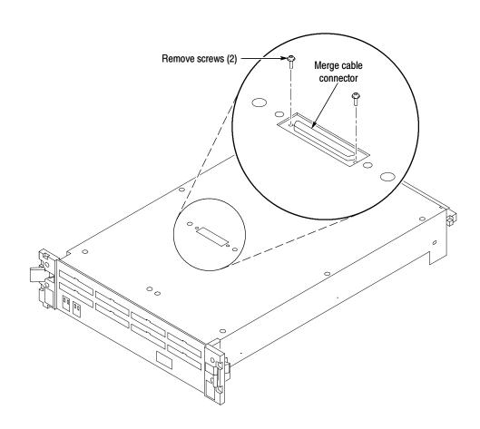
Figure 6-10: Removing the Merge cable connector from the chassis
