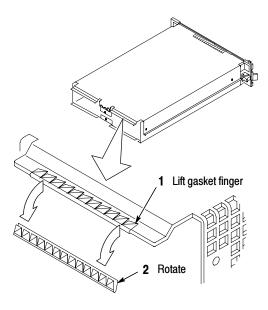
Figure 6-13: Rear EMI gasket removal
