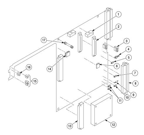
Figure 10-2: TLA700 Series LPU board exploded view
