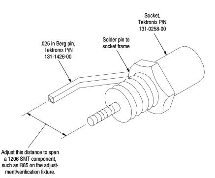
Figure 4-10: Probe tip adapter detail
