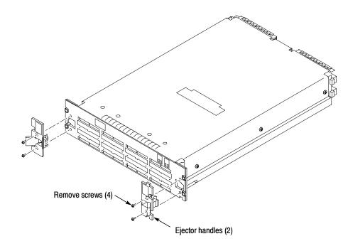
Figure 6-1: Injector/ejector handle replacement
