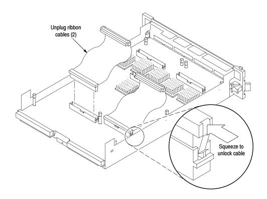
Figure 6-9: Removing the cables from the Acquisition board
