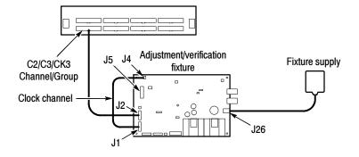
Figure 4-6: Initial FPV\_Setup\_0F test setup
