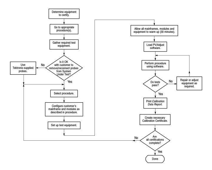
Figure 4-1: Calibration/certification procedure flow chart
