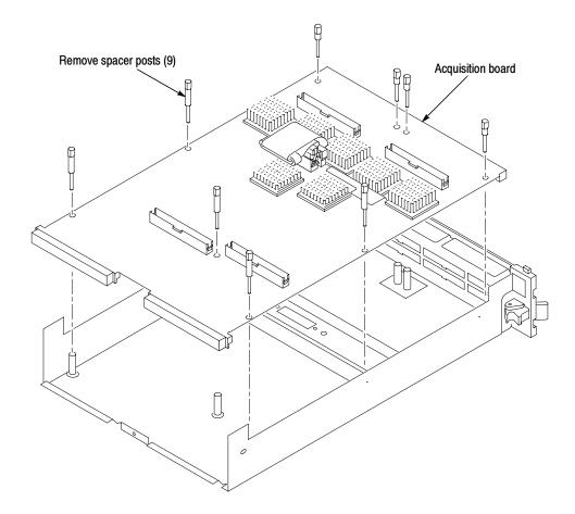
7. Remove the nine spacer posts (with a nutdriver) that secure the acquisition board to the chassis.
