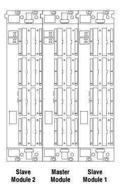
Figure 2-4: Location of modules in a three way merge
