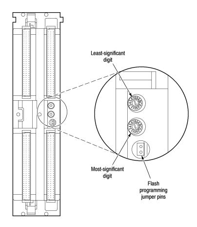
Figure 2-1: Logical address switches
