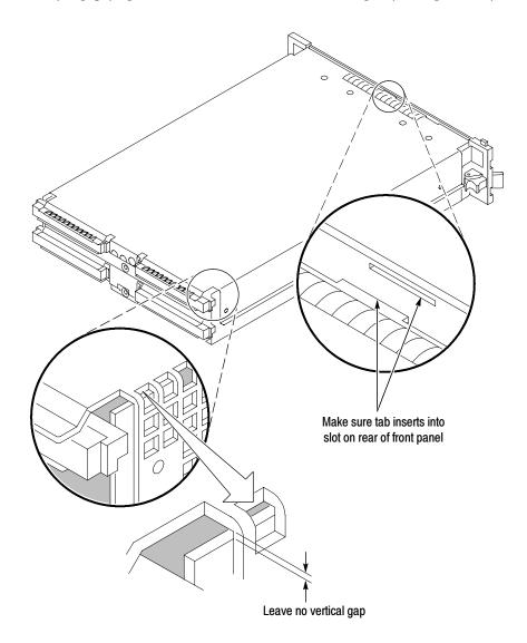
Figure 6-4: Seating the cover on the chassis
