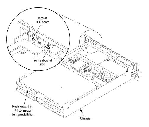
Figure 6-7: Inserting LPU board tabs into front subpanel
