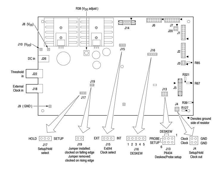
Figure 4-9: Adjustment/verification fixture detail
