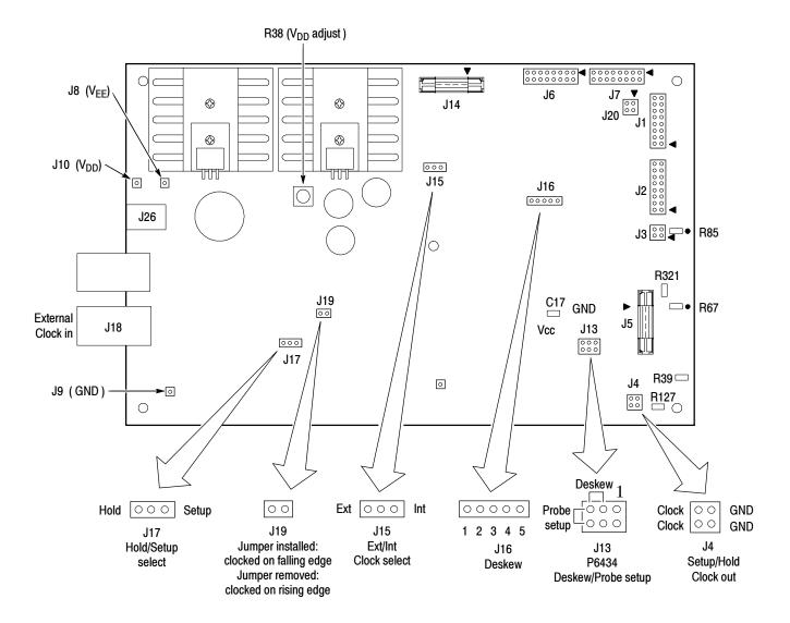
Figure 5-3: Adjustment/verification fixture circuit board layout
