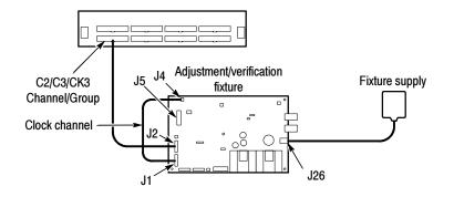
Figure 4-7: Initial FPV\_Hold\_0F test setup
