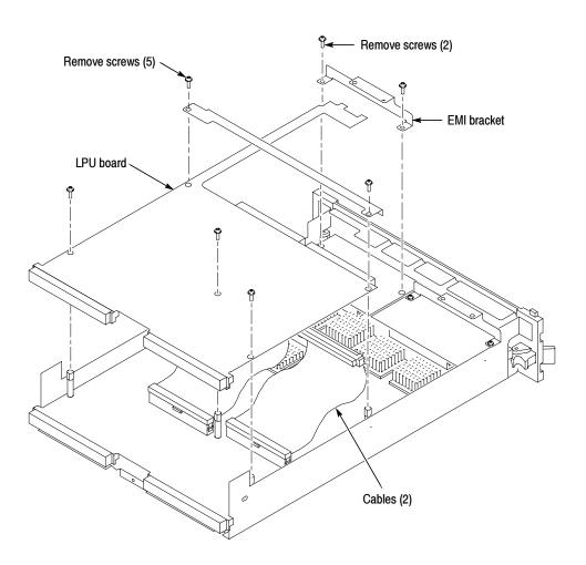
Figure 6-6: LPU board removal
