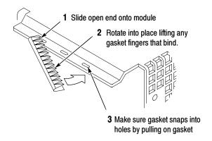
Figure 6-14: Rear EMI gasket replacement
