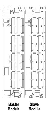
Figure 2-3: Location of modules in a two way merge
