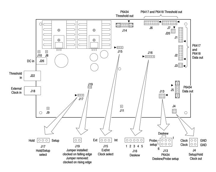
Figure 4-4: Adjustment/verification fixture connections and jumper locations
