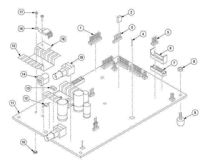
Figure 10-4: Adjustment/verification fixture exploded view
