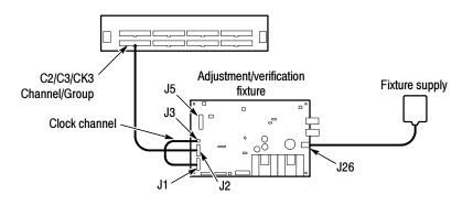
Figure 5-2: Initial deskew test setup
