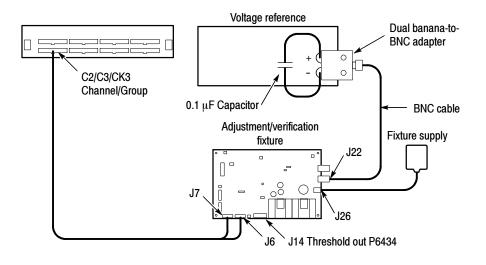
Figure 4-5: FPV\_DC\_Threshold test setup
