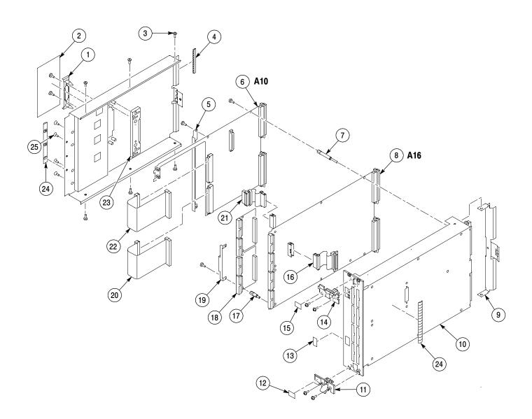
Figure 10-1: TLA700 Series Logic Analyzer Module exploded view
