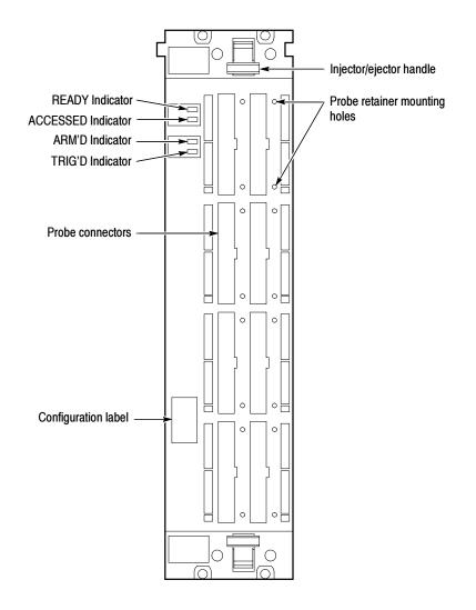
Figure 2-2: Front panel of the logic analyzer module
