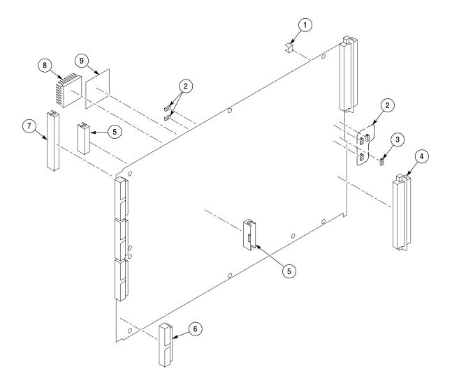
Figure 10-3: TLA700 Series Acquisition board exploded view
