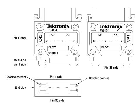
Figure 5-1: P6434 probe detail
