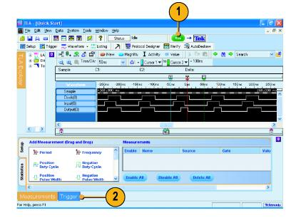
Click and drag the Channel Edge icon from the Tabbed Trigger window to the Output waveform.
