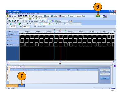
Click and drag the Glitch icon from the Tabbed Trigger window to the Output group waveform.
