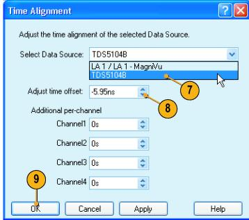
The oscilloscope data is now time-aligned with the logic analyzer data.
