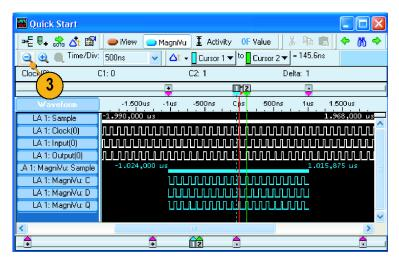
**4.** Move Cursor 1 to an area in the Waveform window outside the range of the MagniVu data.
