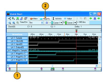
3. Click the Zoom Out button until you see the entire MagniVu timing waveforms. Note that the MagniVu timing data is 16 K bits long as compared to the Deep timing data. Deep timing lets you acquire a large amount of data; MagniVu timing lets you focus on the details of the data. MagniVu data can be up to 128 K bits long for TLA7000 series instruments or 16 K bits long for TLA5000B and TLA6000 series logic analyzers.
