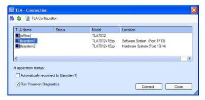
NOTE. To start the TLA Server on TLA7012, TLA6000, and TLA5000B instruments, right-click the (TLA Server) icon in the toolbar at the bottom right side of the screen and select Start TLA Server.
