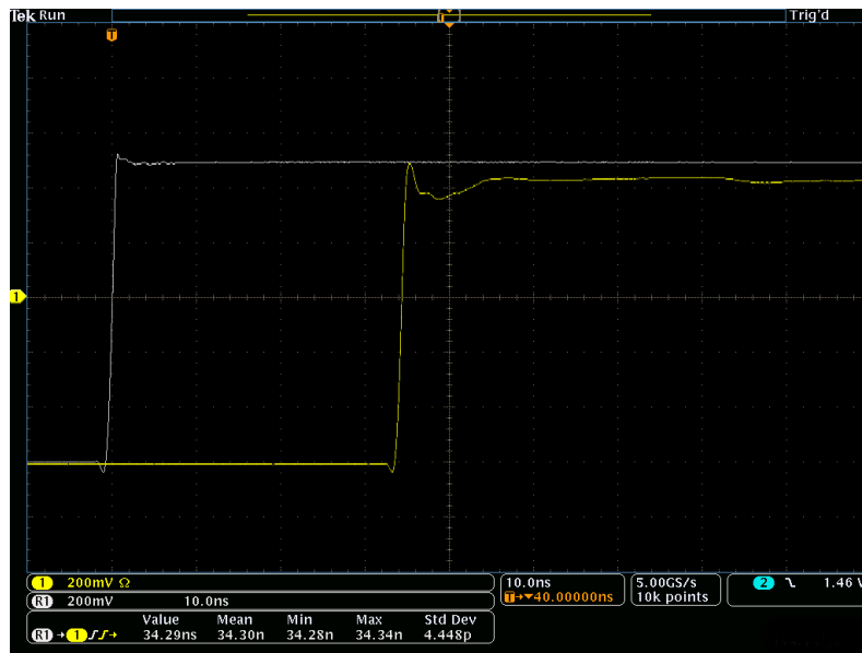
Figure 44: Propagation delay measurement
