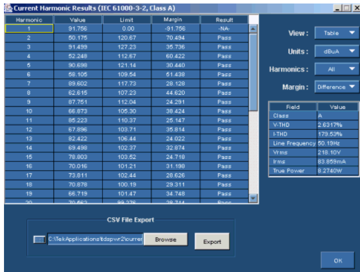
Figure 3-73: Current Harmonics IEC Standards results
