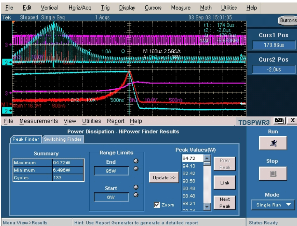
Figure 3-19: Power Dissipation results
