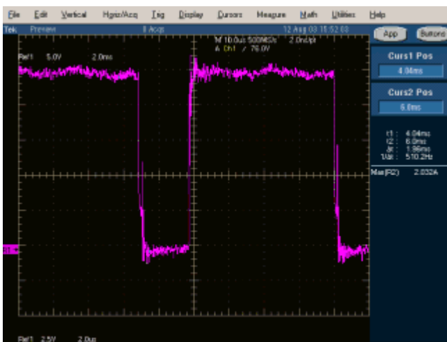
Figure 3-23: Gate signal without a glitch
