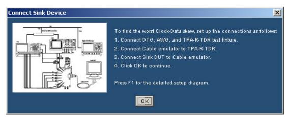
**18.** Follow the instructions in the **Connect Sink Device** dialog box. Click **OK**. The test runs, displaying a progress indicator. The **Confirm Sink Device Support** dialog box appears.
