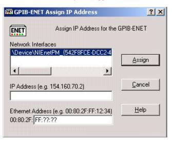
**3.** Enter the new IP Address and the Ethernet Address. Click **Assign**. A message box appears.
