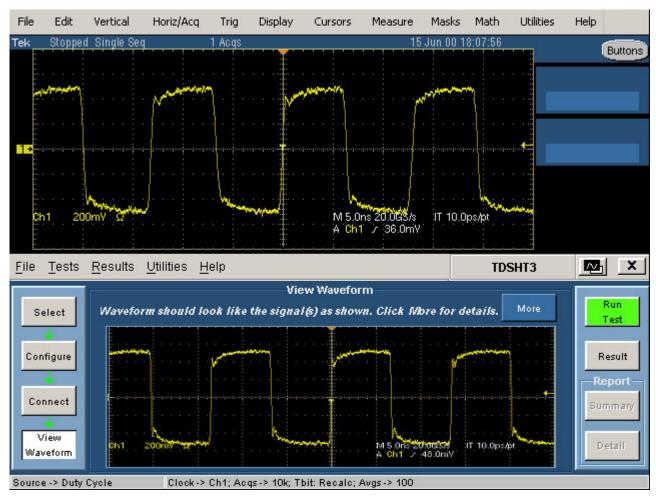
9. Click **Run Test** to perform the test. The TDSHT3 HDMI Compliance Test Software sets up the oscilloscope and the test runs, displaying a progress indicator.
