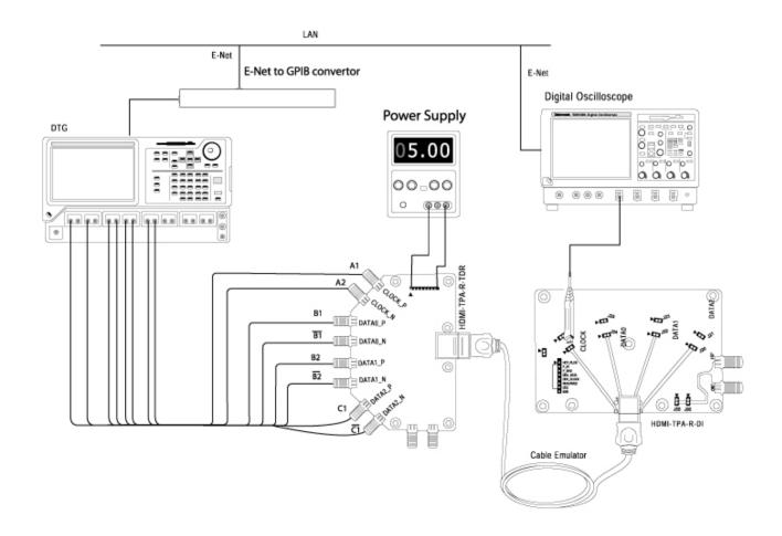
**Note**: Using the Cable Emulator/Cable is not mandatory. You can connect a TPA-P-TDR fixture directly to the DUT. If you find this inconvenient, then use the Cable Emulator/Cable to connect the DUT conveniently.
