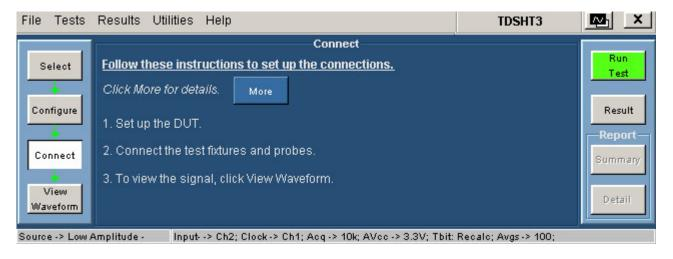
9. Ensure that your signal in the oscilloscope display is similar to the sample signal. Click **View Waveform** to display a sample of the expected signal. If the displays are not similar, go back and check your configuration and connections. The waveform shown here is for the re-calculate Tbit option. Click **Run Test** to run the test. The **Confirm** dialog box appears. Click **Continue** to continue to run the test. Go to step 11.
