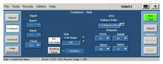
**Note**: The default configuration is to calculate the intra-pair skew of the clock channel. If you want to calculate the intra-pair skew for other data channels, then interchange the DTG physical channels of Data<X> with Clock. For example, to calculate the intra-pair skew of Data0, assign A1 to Data0 and assign B1 to Clock. Make the appropriate changes in the test connections.
