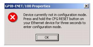
**5.** After you reset the CFG in the ENET card, click **OK** in the **GPIB-ENET/100 Properties** message box. The software will configure and another message box appears.
