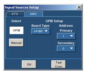
**12.** To configure and test the GPIB connection to the DTG, click **Signal Sources**. The **Signal Sources Setup** dialog box appears.
