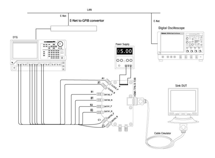
**Note**: Using the Cable Emulator/Cable is not mandatory. You can connect a TPA-P-TDR fixture directly to the DUT. If you find this inconvenient, then use the Cable Emulator/Cable to connect the DUT conveniently.
