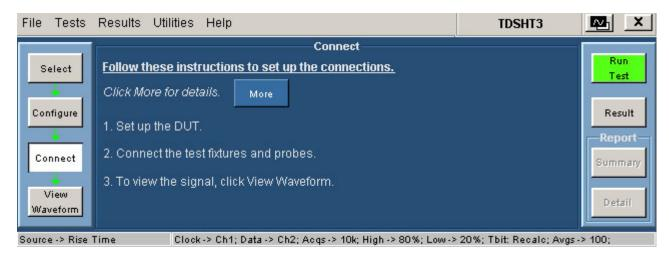
9. Ensure that your signal in the oscilloscope display is similar to the sample signal. Click **View Waveform** to display a sample of the expected signal. If the displays are not similar, go back and check your configuration and connections.
