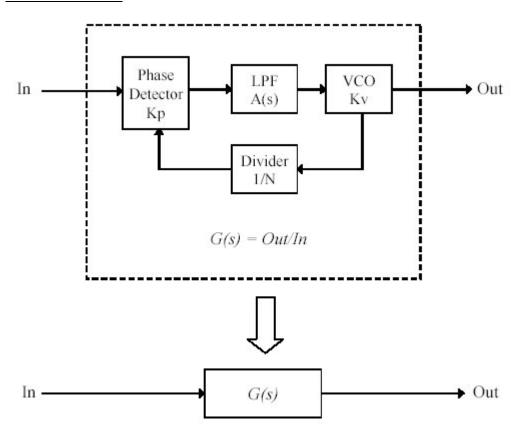
The diagram shows a simplified block diagram of generic phase-locked loop (PLL). A PLL consists of the Phase Detector (PD), Low Pass Filter (LPF), Voltage Controlled Oscillator (VCO), and Frequency Divider (FD).
