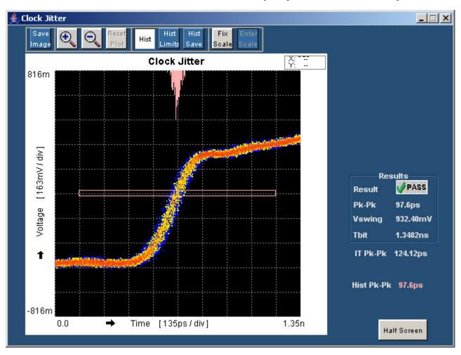
12. Click **Half Screen** to view the clock jitter plot in half screen. You can also view both the result summary of the test and the report configuration in the result pane as shown in the following diagram. For more information on result summary and report configuration, refer to the online help.
