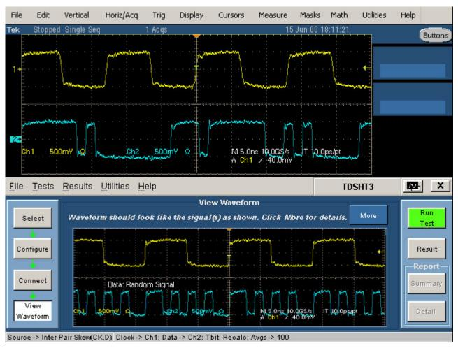
9. Click **Run Test** to perform the test. The TDSHT3 HDMI Compliance Test Software sets up the oscilloscope and the test runs, displaying a progress indicator.
