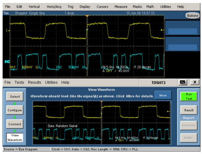
**10.** Click **Run Test** to perform the test. The TDSHT3 HDMI Compliance Test Software sets up the oscilloscope and the test runs, displaying a progress indicator.
