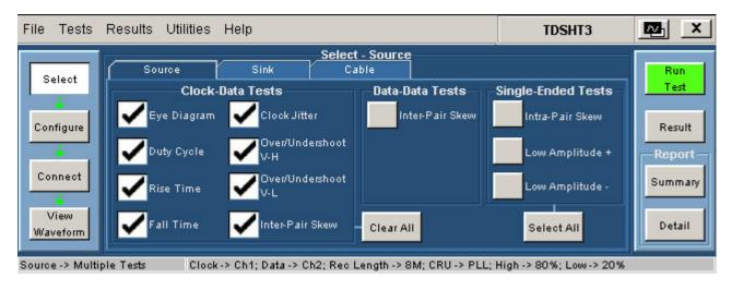
3. To change the configuration settings, click **Tests** > **Configure**. For most tests, you can use the factory default configuration. However, you can change the values by using the virtual keyboard or the general purpose knob on the oscilloscope front panel. Using the File menu, you can also restore the factory defaults or save and recall your own configuration settings.
