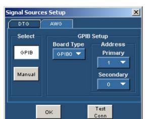
9. To configure and test the GPIB connection to the DTG, click **Signal Sources**. The **Signal Sources Setup** dialog box appears.
