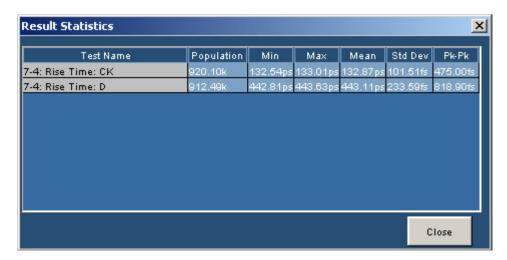
The software calculates statistics for each selected test, and logs the statistics on a cycle-by-cycle basis in a large waveform. The standard statistics are for the Maximum, Minimum, Mean, Standard Deviation, and Population.
