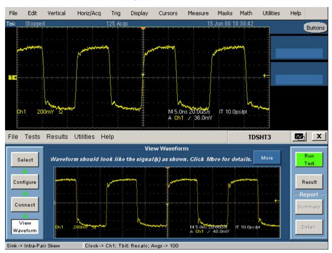
**Note**: To run the test successfully, ensure that the Bus Timing parameter is set to  $2 \mu sec$  on your GPIB board configuration. For more details, refer to the section on Remote Control Caution.
