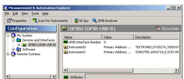
9. Open the Measurement & Automation Explorer software that was installed with the NI-488.2 software.
