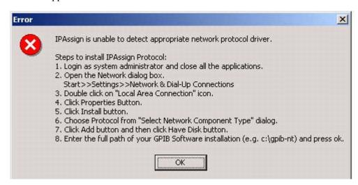
**Note**: The GPIB software installation is in the path C:\Program Files\National Instruments\NI-488.2\GPIB-ENET on the oscilloscope.
