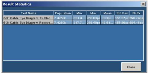
The software calculates statistics for each selected test, and logs the statistics on a cycle-by-cycle basis in a large waveform. The standard statistics are for the Maximum, Minimum, Mean, Standard Deviation, and Population.
