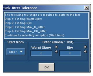
**17.** Follow the instructions in the Sink Jitter Tolerance dialog box. Click **OK**. The **Connect Sink Device** dialog box appears.
