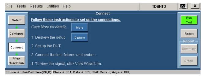
**8.** Ensure that your signal in the oscilloscope display is similar to the sample signal. Click **View Waveform** to display a sample of the expected signal. If the displays are not similar, go back and check your configuration and connections.
