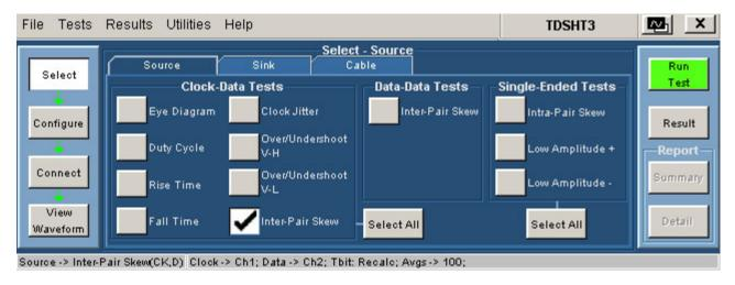
3. To change the configuration settings, click **Tests** > **Configure**. For most tests, you can use the factory default configuration. However, you can change the values by using the virtual keyboard or the general purpose knob on the oscilloscope front panel. Using the File menu, you can also restore the factory defaults or save and recall your own configuration settings.
