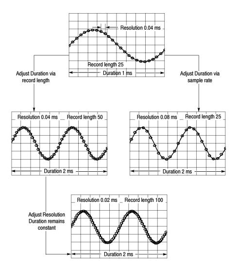
Figure 3-42: Duration and resolution control effects
