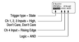
Figure 3-20: Example advanced trigger readout
