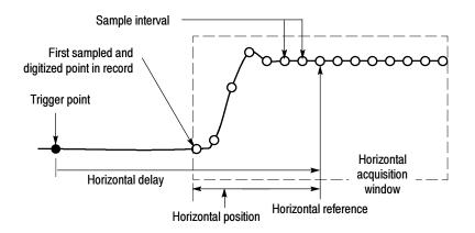
Figure 3-4: Horizontal Acquisition window definition
