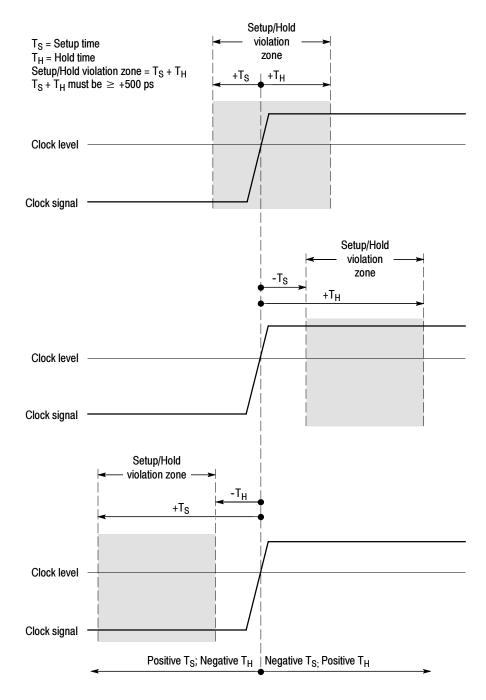
Figure 3-21: Violation zones for Setup/Hold triggering
