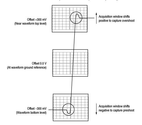
Vertical Window = 100 mV (8 divs X 10 mV /div + (+/-1 divs of position))
