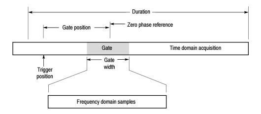
Figure 3-43: Definition of gate parameters
