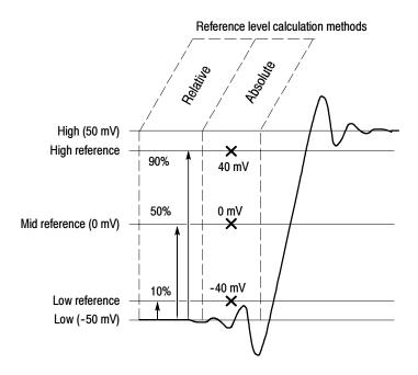
Figure 3-32: Reference-level calculation methods
