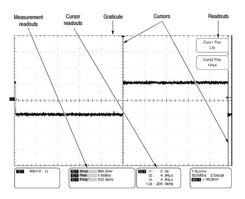
Figure 3-29: Graticule, Cursor, and Automatic measurements
