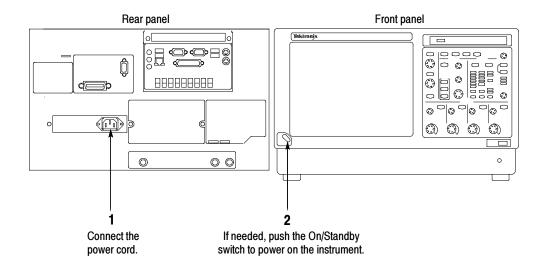
Figure 1-2: Powering on the instrument
