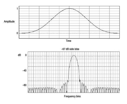
Figure 3-54: Time and frequency graphs for the Kaiser-Bessel window
