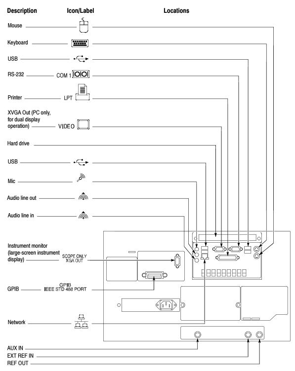
Figure 1-1: Locations of peripheral connectors on rear panel
