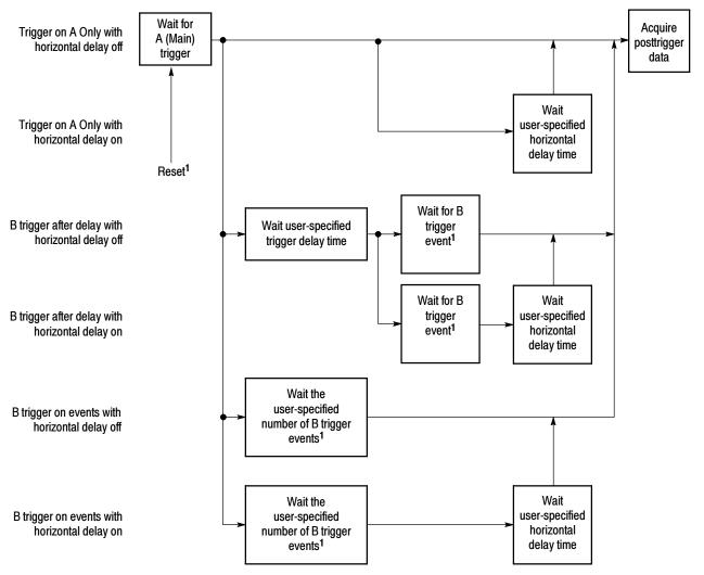
The flow diagram in Figure 3-26 summarizes all combinations of triggering and horizontal delay.
