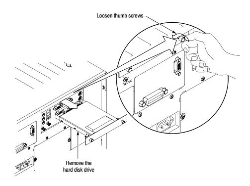
Figure 1-3: Removing the hard drive
