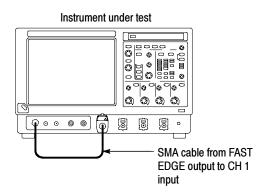
Figure 1-9: Universal test hookup for functional tests - CH 1 shown
