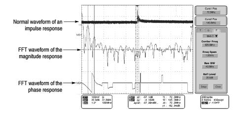
Figure 3-38: Spectral analysis of an impulse
