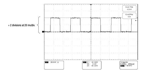
Figure 3-33: Horizontal cursors measure amplitudes
