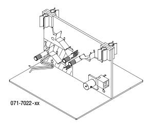
Figure 3-36: Probe calibration and deskew fixture
