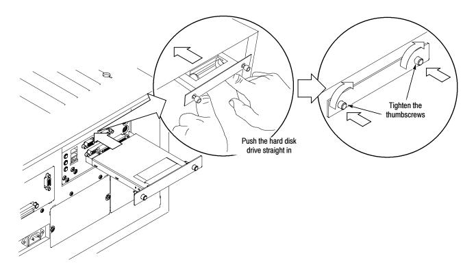
Figure 1-4: Reinstalling the hard drive
