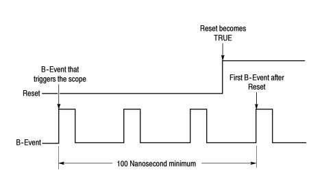
Figure 3-25: Reset trigger limitation
