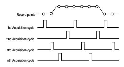
Figure 3-12: Equivalent-time sampling
