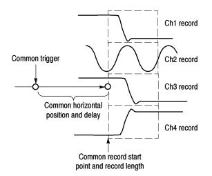
Figure 3-5: Common trigger, record length, and acquisition rate for all channels
