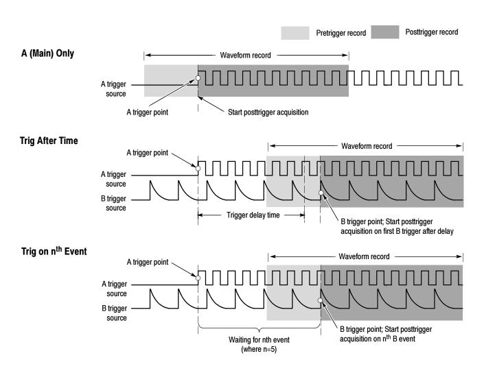
Figure 3-23: Triggering with Horizontal Delay off
