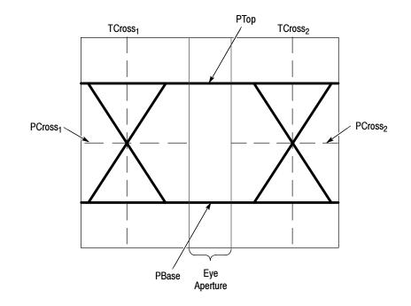
Figure C-5: Eye-diagram and optical values
