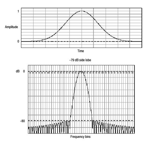
Figure 3-50: Time and frequency graphs for the Gaussian window
