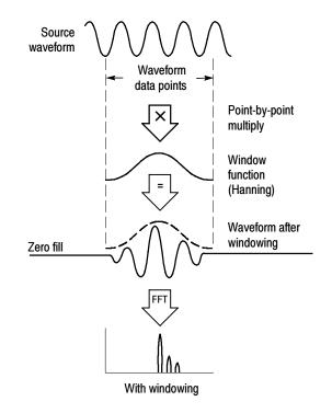
Figure 3-48: Windowing the time domain record
