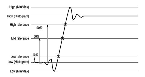
Figure A-1: Levels used to determine measurements
