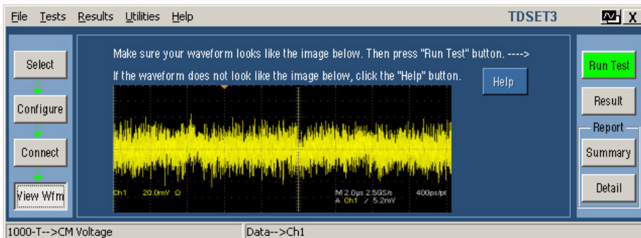
Figure 11-13: 1000BASE-T View Waveform for CM Voltage
