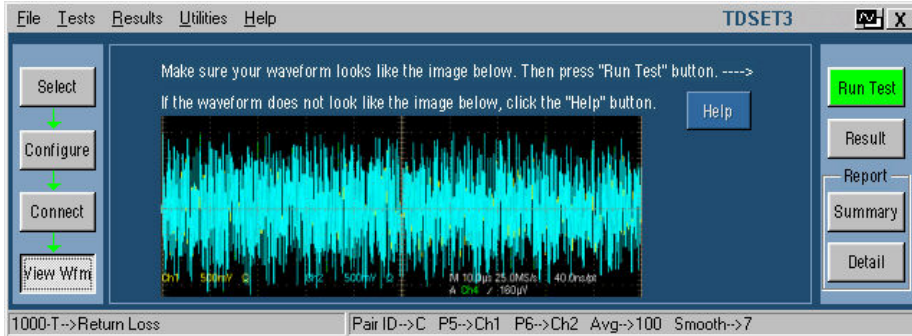
Figure 11-12: 1000BASE-T View Waveform for Return Loss
