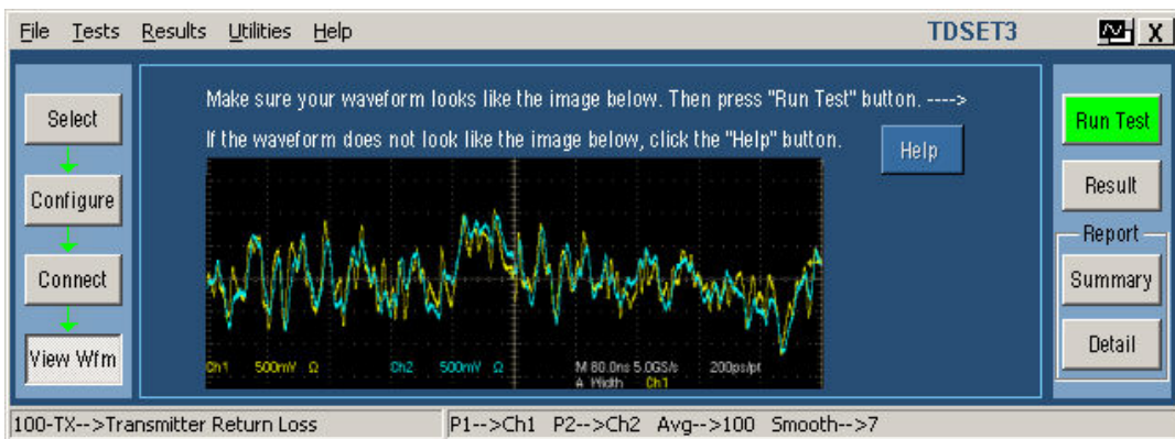
Figure 12-2: 100BASE-TX View Waveform for Return Loss Transmitter
