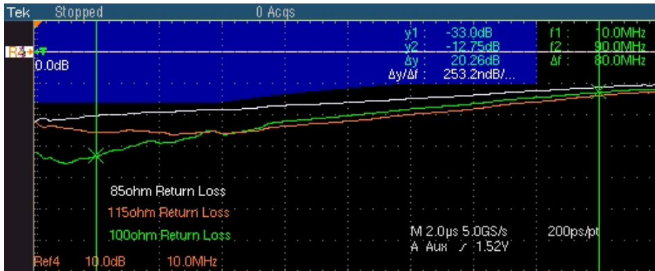
Figure 9-18: Waveform for 100BASE-TX Return Loss Transmitter
