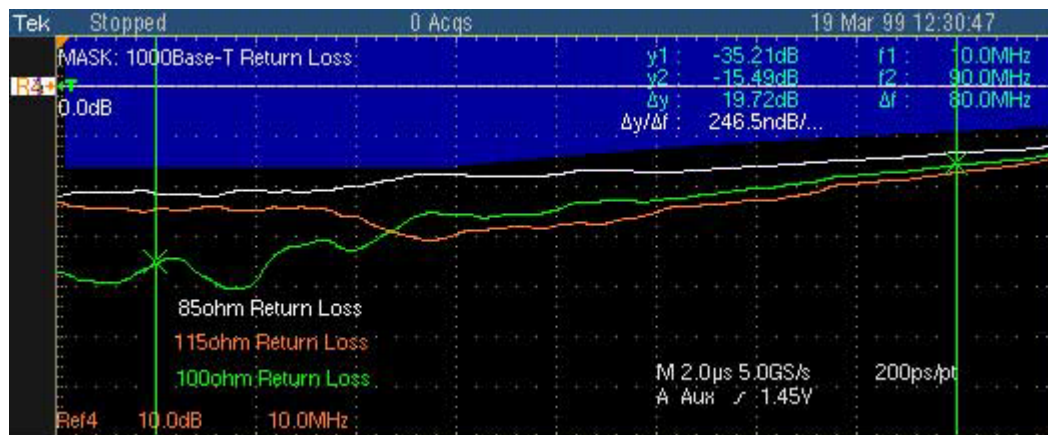
Figure 8-23: Waveform for 1000BASE-T Return Loss
