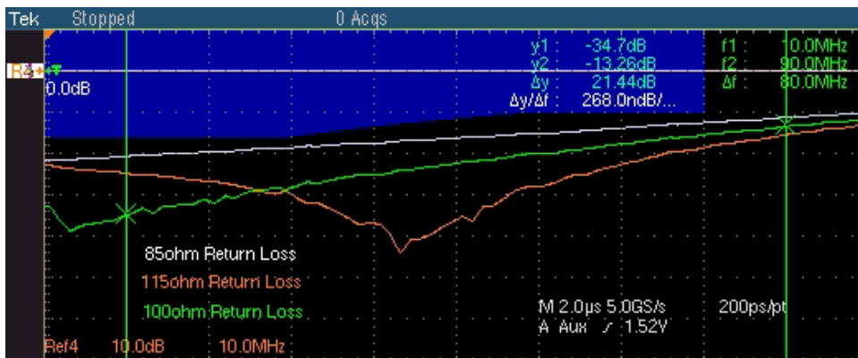
Figure 9-19: Waveform for 100BASE-TX Return Loss Receiver
