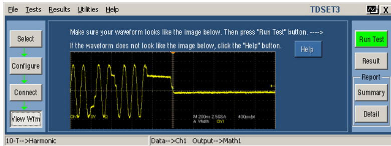
Figure 13-9: 10BASE-T View Waveform for CM Voltage
