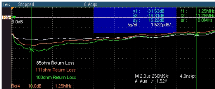
Figure 10-23: Waveform for 10BASE-T Return Loss Transmitter
