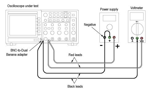
**4.** Set the power supply to the 1.8 V value shown in column A, the Approximate Test Voltage.
