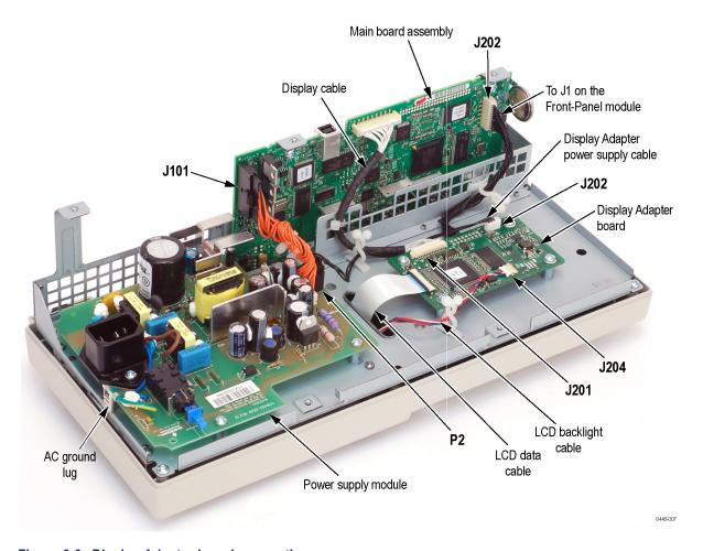
Figure 6-3: Display Adapter board connections
