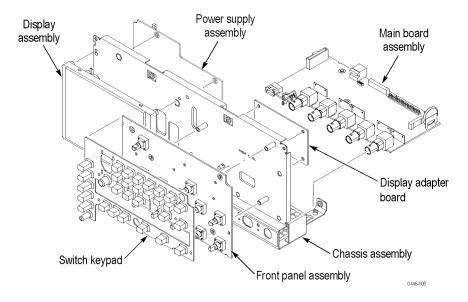
Figure 6-2: Locator for internal modules (4-channel model shown)
