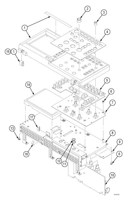
Figure 8-1: Exploded diagram, 2-channel models
