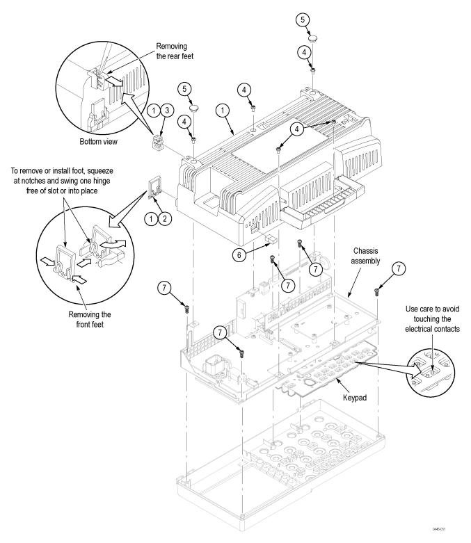
Figure 8-4: Exploded diagram, back case and trim
