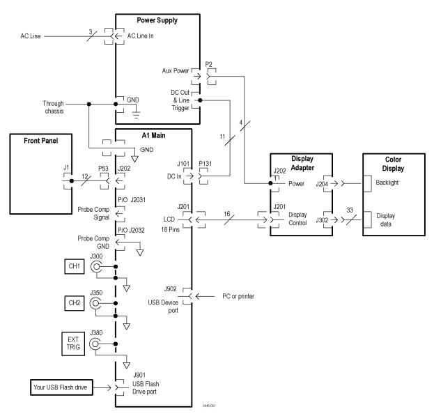
Figure 3-1: Module-level block diagram (2-channel)
