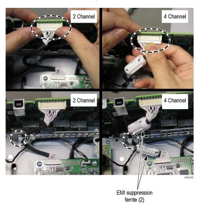
Figure 6-4: Connecting the Display cable
