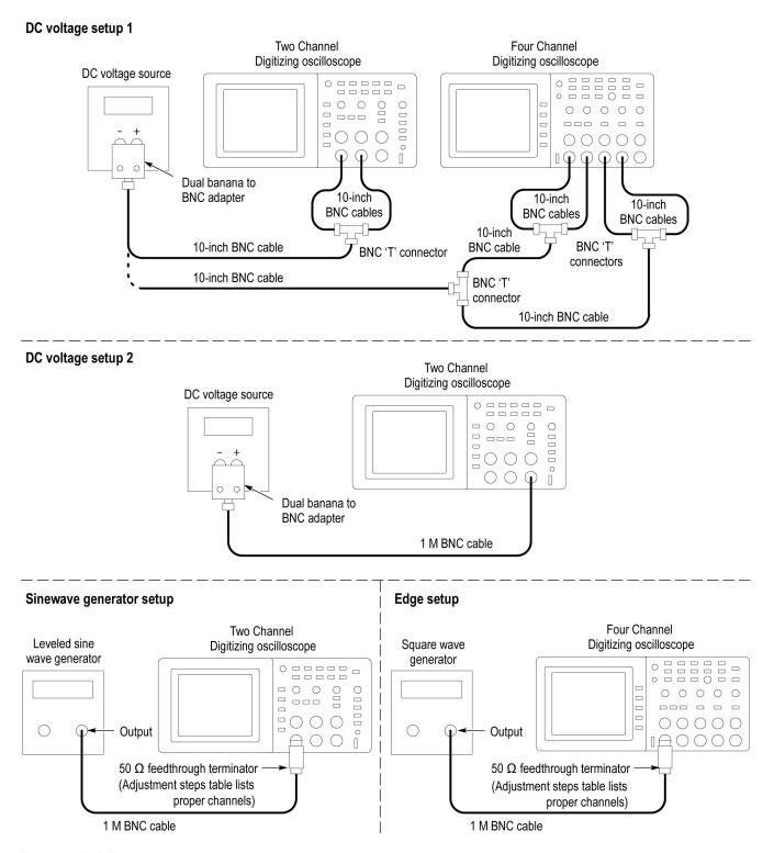
Figure 5-1: Adjustment setups
