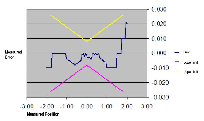
Figure 4-1: Example of a line graph for the Vertical Position Accuracy test
