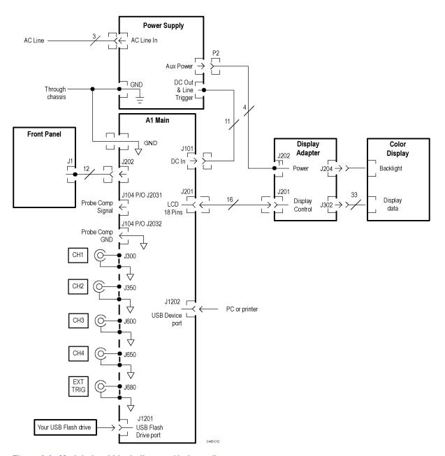
Figure 3-2: Module-level block diagram (4-channel)
