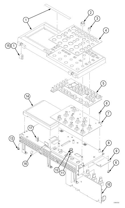
Figure 8-2: Exploded diagram, 4-channel models
