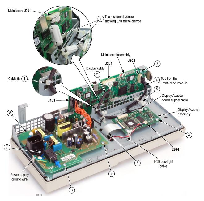
Figure 8-3: Power supply module, cables, and wires (2-ch model shown, with 4-ch model in circle)
