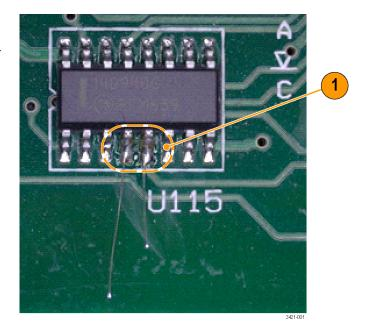
Thread tip onto wires. The two middle vias are the A(+) and B(-) inputs of the tip.
