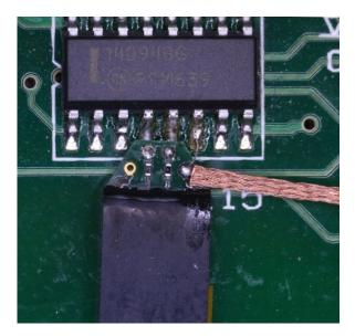
2. Use the solder-wick to remove excess solder from the input vias. Again, be careful not to place the solder-wick too close to the input resistors.
