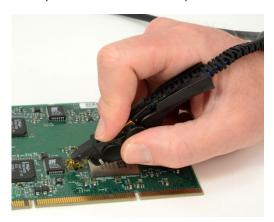
The browser is a differential only probe accessory, but can be used to measure ground referenced, single-ended circuits as well. When measuring a ground referenced signal, connect the A side (positive) input to the signal to be measured and the B side (negative) to the ground connection.
