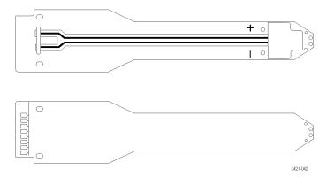
The flex circuit based solder tips are made with flex circuit material and can be bent and shaped to fit around or into spaces where it is difficult to reach a test point.
