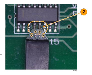
3. With the tip in position, quickly solder the wires to the vias. If the soldering iron is left too long on the tip, it may cause the 0201 input resistors to reflow and move.
