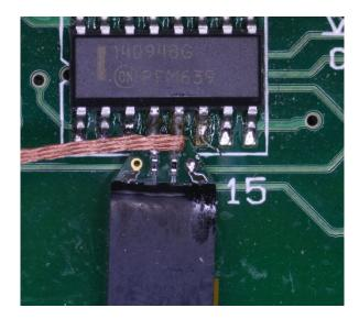
3. If the solder cannot be fully removed from the input via while attached to the test points, it is possible rock the tip side to side while reflowing the solder in the vias. Since the wires are cut flush to the board, the tip can be slowly removed from the wires using this method. Once the tip has been removed from the board, use the solderwick to clean out the vias so the tip can be reused.
