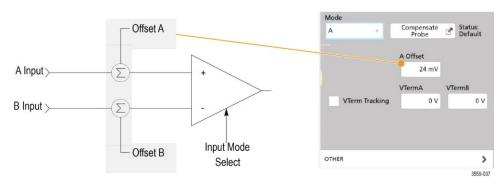
Figure 1: Simplified probe input model
