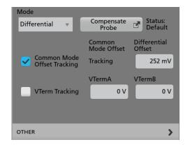
**Differential Mode Offset Tracking.** When this mode is selected Differential Mode Offset is set to tracking.
