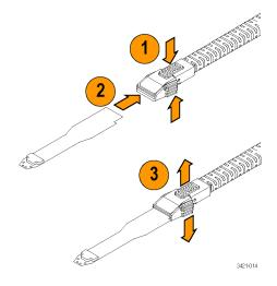
3. Once the tip is fully inserted, release the pinch and the TekFlex connector closes. When closed and properly seated, the top of connector will be flush with the probe tip housing.
