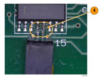
5. Attach the ground wire for TriMode input to the probe tip. First add solder to the test point and the nearest ground via on the solder tip.
