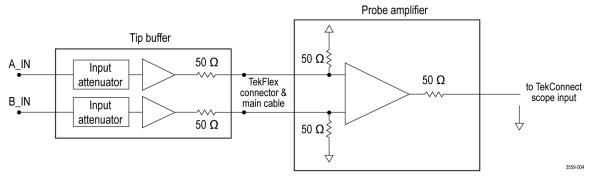
Figure 3: Simplified probe architecture diagram
