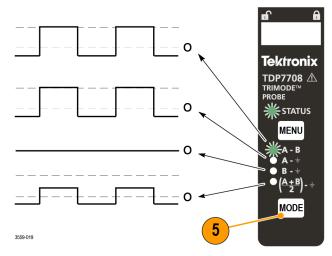
6. Change the SMA cable connection from the Deskew Fixture A input to the B input. Repeat the displayed waveform checks. The measurements should be different as follows:
