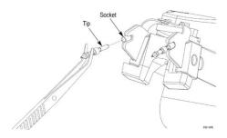
Once the old tip has been removed, retrieve a new, replacement tip from its storage vial in the accessory kit. Grip the replacement tip with the tweezers, gently push the tip into the socket on the browser's front end.
