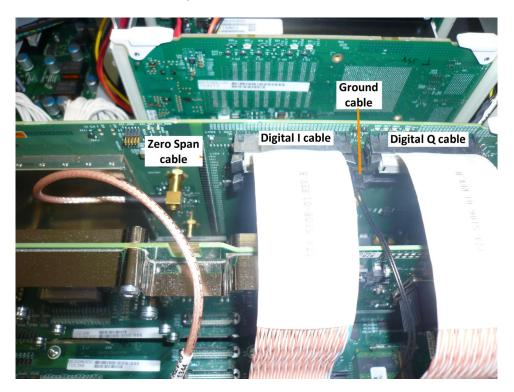
Figure 5: Option 65, 66, 6566 cables reinstalled
