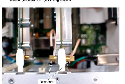
2. Disconnect the two SMB cable assemblies from the installed acquisition board (in Slot 1). (See Figure 3.)
