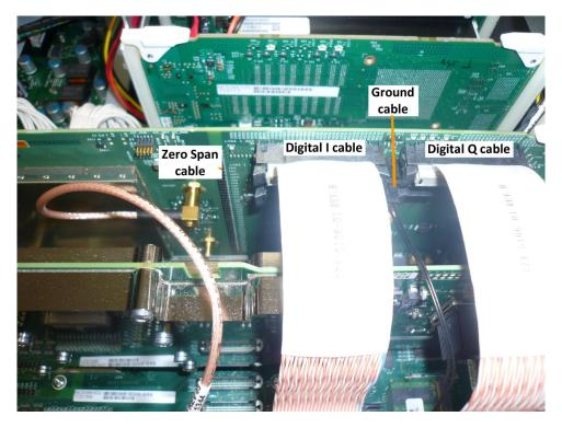
Figure 2: Disconnect Option 65, 66, 6566 cables
