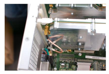
**3.** Reconnect the SMB cable to the connector on the front of the new acquisition board (the side facing the rear panel).
