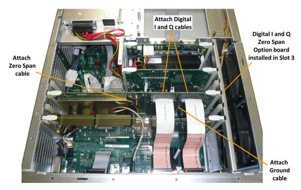
Figure 4: Installing the option board
