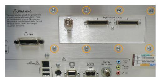
Figure 3: Installing the rear panel cover on the rear panel of the chassis
