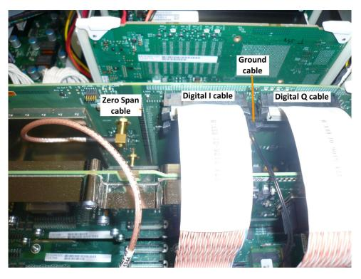
Figure 5: Connecting the output cables
