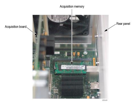
**1.** Use the ejector latches to release the existing acquisition memory module. Place the memory module into a static-shielded bag.
