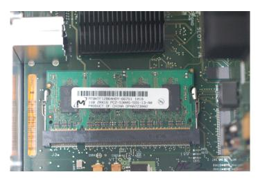
2. Insert the new memory module at an approximately 45° angle, making sure the gold "fingers" are fully seated. Then rotate the module down toward the board until the latches click into place.
