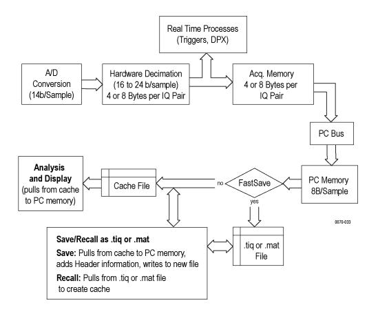
FastSave mode bypasses cache file creation and writes directly to a file. This eliminates two of three disk read or write operations. Depending on the file size, FastSave reduces the time required for data acquisition up to 65%. Using FastSave means that *only* real-time processes will be used. The instrument triggers and DPX display are not affected. All other measurements are suspended, and an information message (Disabled - FastSave is selected) is displayed in the graph area of each display.
