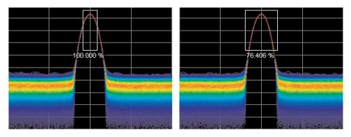
Figure 24. Density of signals defined within an area. Left: Correct measurement of a CW signal. All columns in the box include the signal. Right: Incorrect measurement area. The measurement is accurate, but probably not what you expected. Some columns in the box contain no hits, so they contribute zeros to the calculation of average density.
