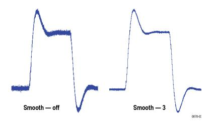
The range for the Smooth function is 2-1000. The setting resolution is 1. The knob increments this value by 1, and the arrow keys increment it in steps of 1, 2, 5, 10. When smoothing is enabled, it applies to both traces. Smooth is turned off by default.
