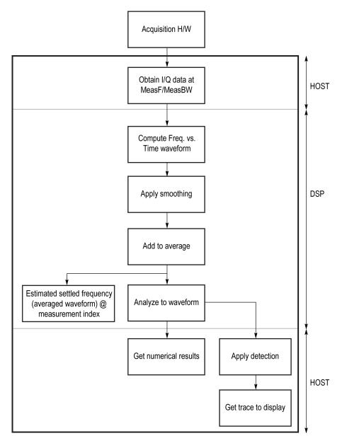
Frequency settling time flow diagram
