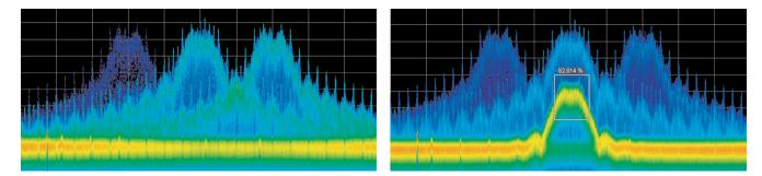
Figure 29. Example of Density Trigger. Left: A free-run DPX display showing pulses with varying frequency. Occasionally, a short pulse in the middle appears for a split instant, but it is hard to capture it with just a Run/Stop button. Right: The triggered DPX displays shows the low-amplitude pulse that was not apparent in the untriggered display. The analyzer was set to trigger whenever the average density in the user-drawn box measured 50% or higher.
