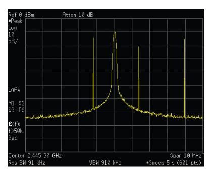
Figure 16. Swept spectrum display of the infrequent transient.
