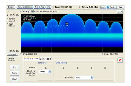
**Searching for peaks on the DPX bitmap trace.** To locate peaks on the DPX Bitmap trace, use the arrow buttons on the Marker toolbar. The left / right arrows move the selected marker to the next peak lower or higher in frequency. The up and down arrows search for peaks at the same frequency. The peaks on the DPX Bitmap trace are defined by the settings for the DPX Signal Density on the Markers > Define Markers > Define Peaks (see page 376) tab.
