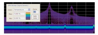
Figure 12. Adjusting to values less than 1, increases the contrast for viewing events in the top half of the selected density range.
