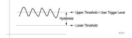
The following figure shows that a trigger is generated when the signal frequency changes sufficiently to exceed the hysteresis value (the difference between the upper and lower thresholds) and cross the lower threshold followed by crossing the upper threshold.
