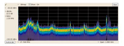
Figure 14. Off-air ambient signals over a 1 GHz span in the swept DPX display.
