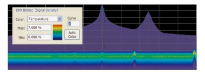
Figure 11. Over a narrow Signal Density range, the color curve is set to 1.
