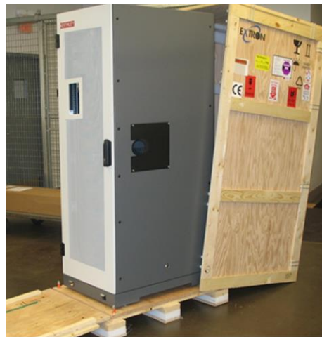
Figure 8: Sliding the outer box off the crate
