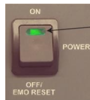
Figure 26: Indicator showing system power is still on
