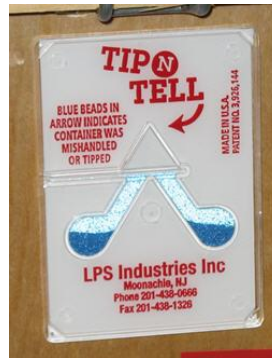
Figure 3: S540 crate tipping indicator
