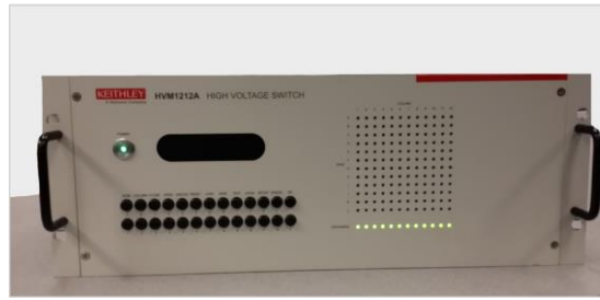
Figure 51: HVM1212A High-Voltage Matrix
