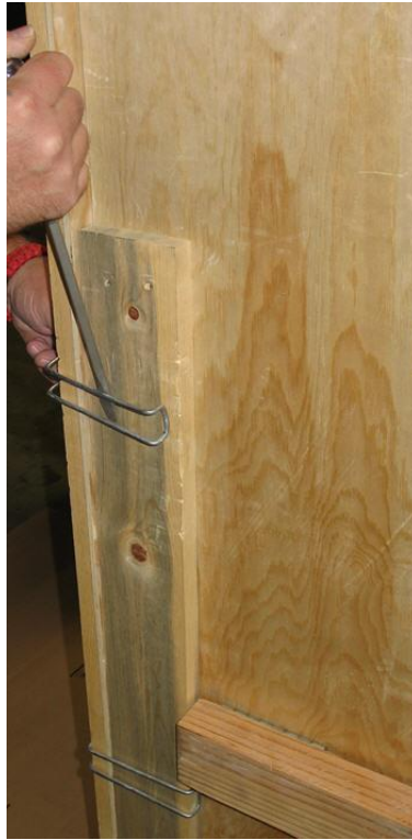
Figure 4: Removing the crate clamps
