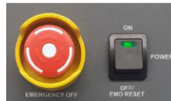
Figure 36: S540 power ON switch
