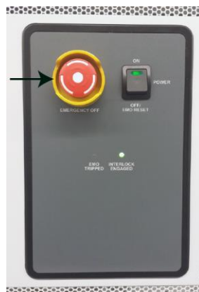
Figure 39: EMERGENCY OFF button
