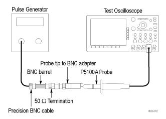
Figure 9: Setup to adjust HF response
