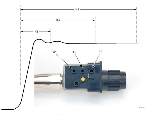
Figure 15: Areas of the waveform affected by adjustments R1, R2, and R3
