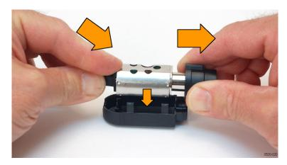
Figure 11: Align and seat the probe into the bottom cover
