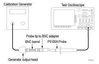
Figure 2: Setup for system accuracy check
