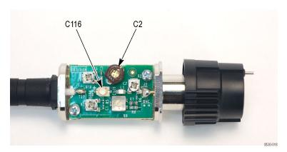
Figure 8: C2 (LF) and C116 (fine LF) adjustment locations
