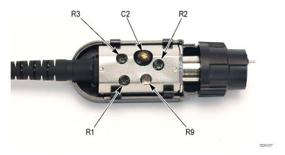
Figure 6: P5100A probe adjustment locations
