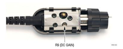
Figure 7: R9 (DC gain) adjustment location
