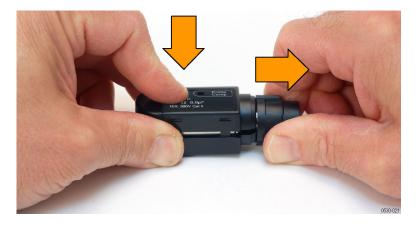
Figure 12: Install the top cover
