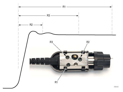
Figure 10: Areas of the waveform affected by adjustments R1, R2, and R3
