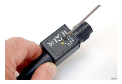
Figure 13: Depress the tab and slide back the cover
