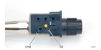
Figure 14: LF and fine LF adjustment locations
