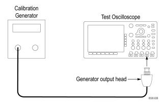
Figure 1: Setup for oscilloscope gain check
