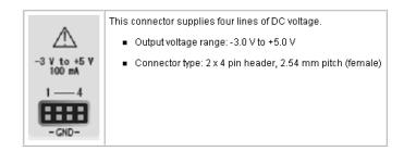
Of these four lines, only the first two DC outputs (DC1 and DC2) are used.
