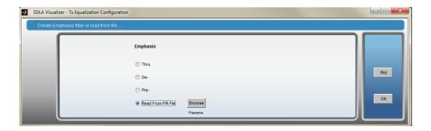
**NOTE.** The filter setup need not be an emphasis type. It may be of any type required to better simulate your system.
