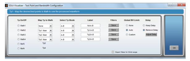
**Tp On/Off.** Controls which of the six (4 math and 2 reference) active test point waveforms are on or off. Each radio button lists the name of one of the available Math functions or a Ref memory waveform in the oscilloscope. If the button is off, then the waveform on the oscilloscope screen is turned off. If the button is on, then the waveform on the oscilloscope screen is turned on.
