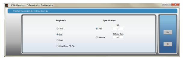
Four types of filter response are available. Each option offers the ability to either remove the effects of a component or to simulate one. The Pre/De-emphasis units are in dB. You can use the typical 3 dB setting or enter a custom dB setting. To see the results of the filter on the source signal, press **Apply** on the Main Menu to recompute the system's test point filters.
