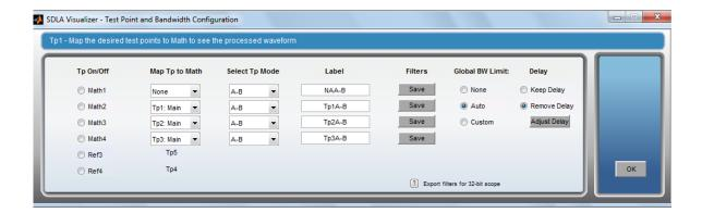
2. Under Global BW Limit, select Custom and then press Setup BW. This brings up the Bandwidth Limit Filter Design Menu.
