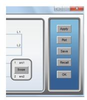
**Apply.** When you press the local **Apply** button, SDLA computes the filters for all enabled test points throughout the entire system. Unlike pressing Apply on the Main Menu, this Apply does not send the filters to the scope math function and it does not bring up DPOJET. This provides faster compute time while you dial in all the settings in the system.
