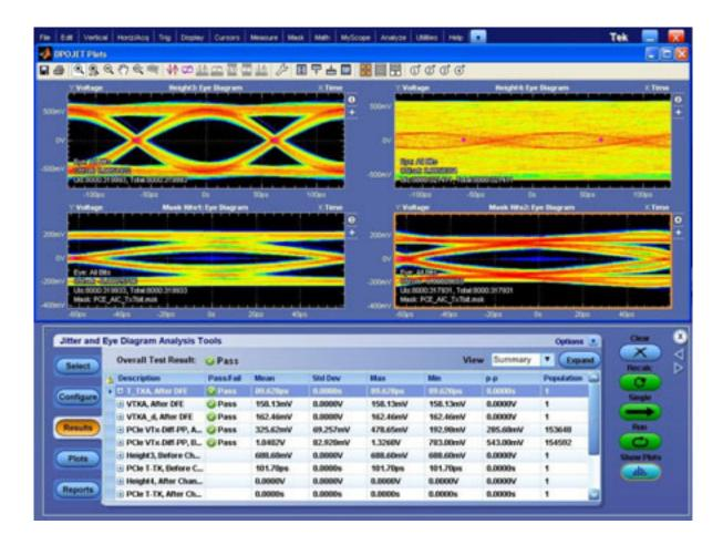
To switch between SDLA Visualizer and DPOJET, use the Alt Tab keyboard combination or the navigation buttons (< and >) on the SDLA Main Menu. Use the TekScope application minimize button to minimize the scope window to view the DPOJET and SDLA applications.
