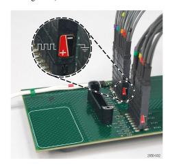
Figure 4: Differential probe connections
