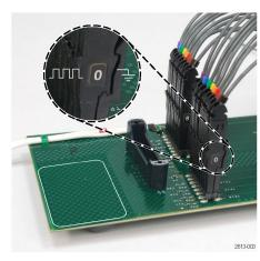
Figure 3: Single-ended probe connections
