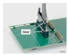
Figure 5: P6750 Probe connection
