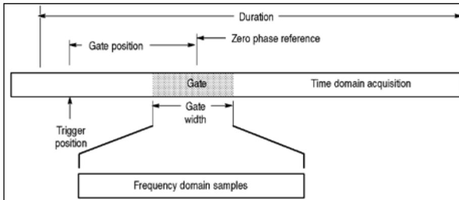
Time domain gating is inversely proportional to the resolution bandwidth of the spectral waveform. The narrower the gate, the larger the resolution bandwidth and the lower the frequency resolution. To obtain the best frequency resolution, use as wide a gate as possible.
