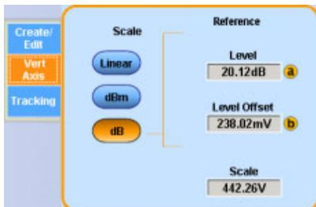
**NOTE.** The reference level offset is used to calculate the log magnitude in dB. Adjusting the reference level positions the waveform with respect to the top of the screen but does not change the position of the waveform with respect to the ground reference marker.
