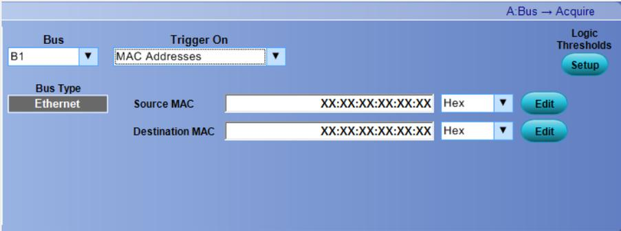
The screenshot shows a configuration window titled "A: Bus → Acquire". It has a "Bus" dropdown set to "B1" and a "Trigger On" dropdown set to "MAC Addresses". Below this, there is a "Bus Type" section with "Ethernet" selected. Two rows are visible for MAC addresses: "Source MAC" and "Destination MAC". Each row has a text input field containing "XX:XX:XX:XX:XX:XX", a "Hex" dropdown, and an "Edit" button. In the top right corner, there is a "Logic Thresholds" section with a "Setup" button.
