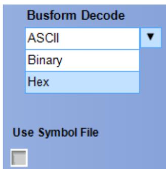
For the USB serial bus, you can display the decode of the bus in Mixed Hex, Mixed ASCII, Hex, Binary, Packet, and Details. The speed you select determines the available decodes. Select the decode from the drop down list.
