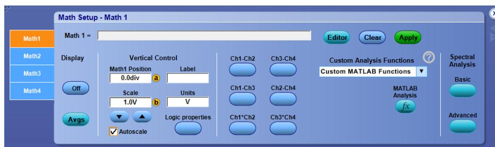
You can define up to four math waveforms. The controls for each waveform are similar, but independent of each other.
