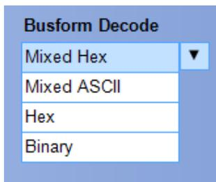
For the Ethernet serial bus, you can display the decode of the bus in Mixed Hex, Mixed ASCII, Hex, and Binary. Select the decode from the drop down list.
