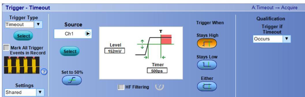
The following Trigger Timeout screen appears on MSO/DPO5000B Series instruments:
