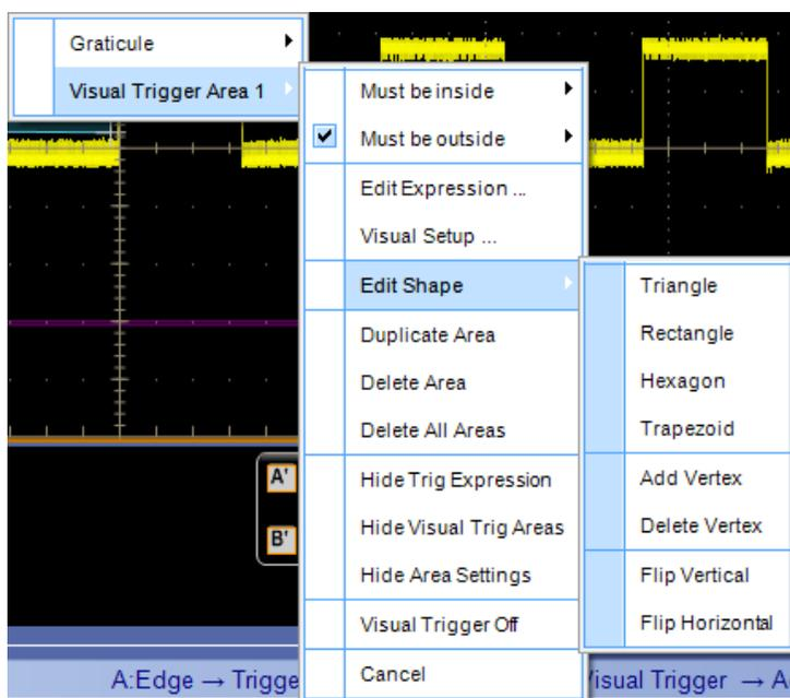
Select Edit Shape to change the shape and orientation of the visual trigger area. Selections include the following:
