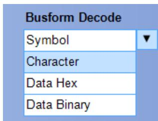
For the PCIe serial bus, you can display the decode of the bus in Symbol, Character Symbol, Character KCode, Data Hex, Data Binary, Descrambled Hex, and Descrambled Binary. Select the decode from the drop down list.
