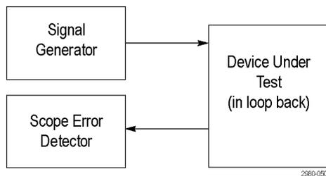
With the DUT inserted between the Signal Generator and the Serial Error Detector, all you need to do to get the Error Detector running is to press the Sync and Run buttons, because the Learn operation was completed in the previous step. If you do another Learn operation, you risk learning errors created by the DUT.
