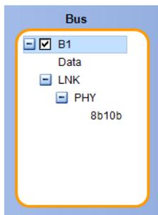
Bus views may also be added or removed from the display by clicking on the + box or - box in the display. Available views may include Transaction/transport, link/framing/packets, physical/bytes/symbols, and bit level.
