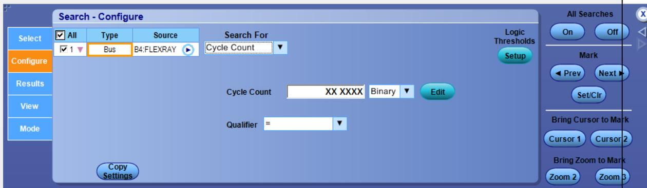
Select the Quallifier from the drop-down list. Click Edit to enter the Cycle Count value. Click Logic Thresholds to adjust the logic thresholds.
