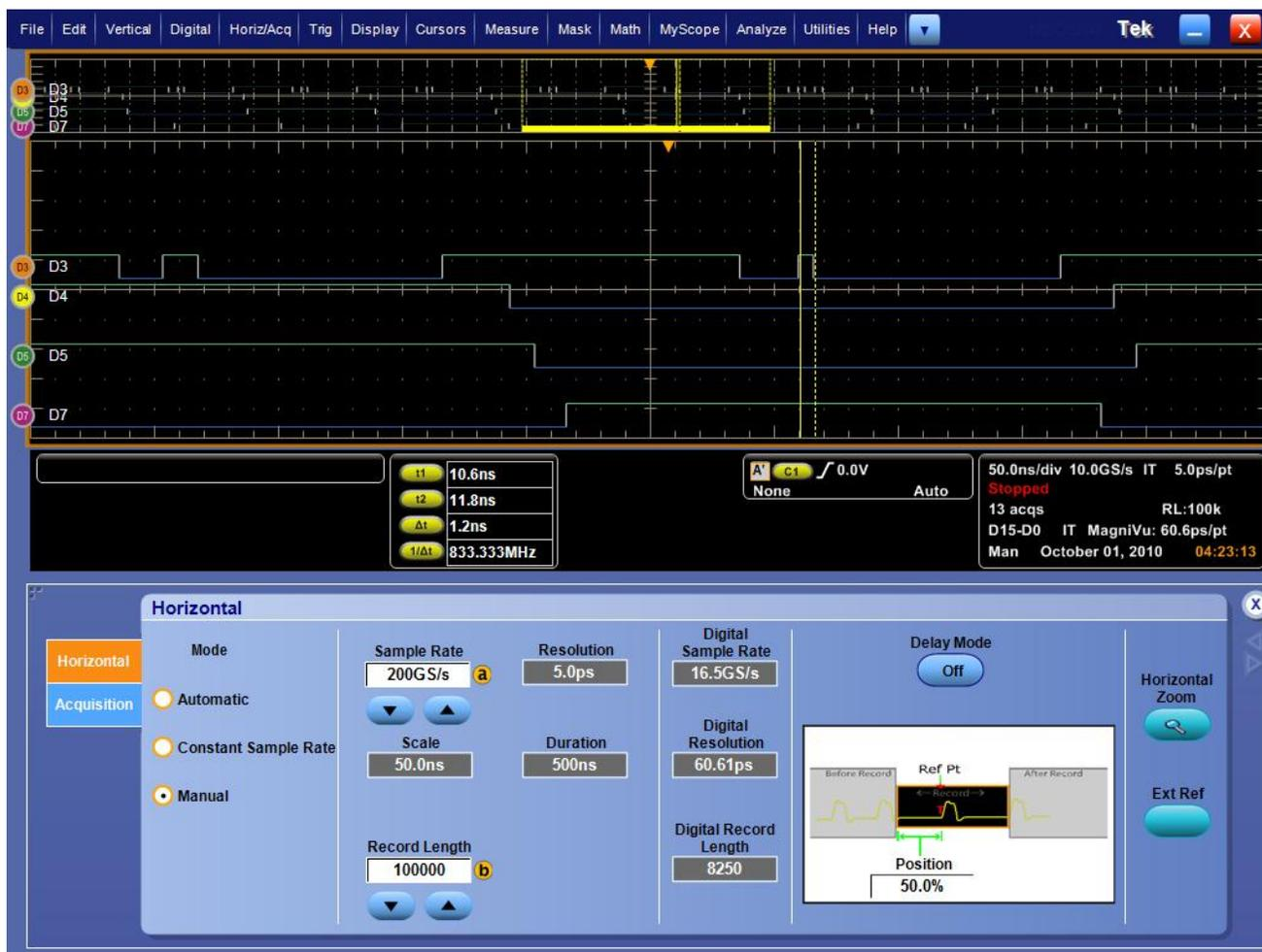
**NOTE.** The MagniVu record must always contain the trigger. If the trigger point is moved prior to the display region using Horizontal Delay, then the MagniVu record will not be available. In most of these cases, you can find the digital record by looking for the digital signal in the upper overview and panning accordingly.
