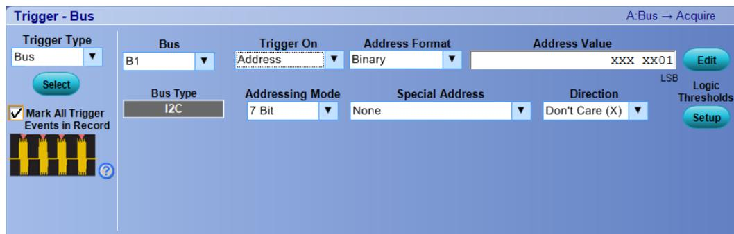
In the following example on MSO/DPO5000B Series instruments, you need to set an Address Format, Address Value (click the [Edit \(see page 942\)](#) button), Addressing Mode, Special Address, Direction, Number of Bytes, Data Format, Data Value ([Edit \(see page 942\)](#)) for the Addr+Data Trigger On type. Optionally, you can also set the component threshold levels through the Logic Thresholds Setup button.
