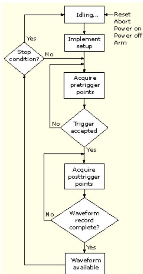
1. The instrument starts in the idle state; it enters this state at power on, upon receiving most control setting changes, or on finishing acquisition tasks.
