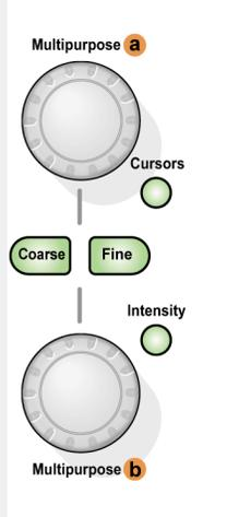
You can undo any mapping by right-clicking the multipurpose knob(s) and selecting Deassign Multipurpose Knobs, or from the Utilities menu, select the Deassign Multipurpose Knobs command. The mapping is deassigned until you perform that function again.
