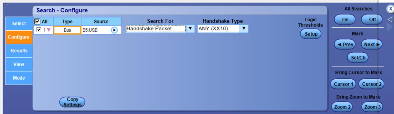
Select the Handshake Type from the drop-down list. Click Setup to adjust the logic thresholds.
