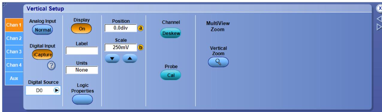
**NOTE.** Right-click on the digital source readout in the waveform window to reroute from one analog channel to any of the other three analog channels. For example, right-click on D0 captured on Ch1 and select **iCapture on Ch2** to reroute the source D0 to Ch2.
