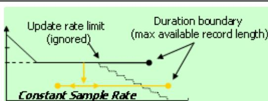
**Manual.** Use this mode to set the Sample Rate and Record Length; the horizontal scale is a dependent variable calculated from the sample rate and record length.
