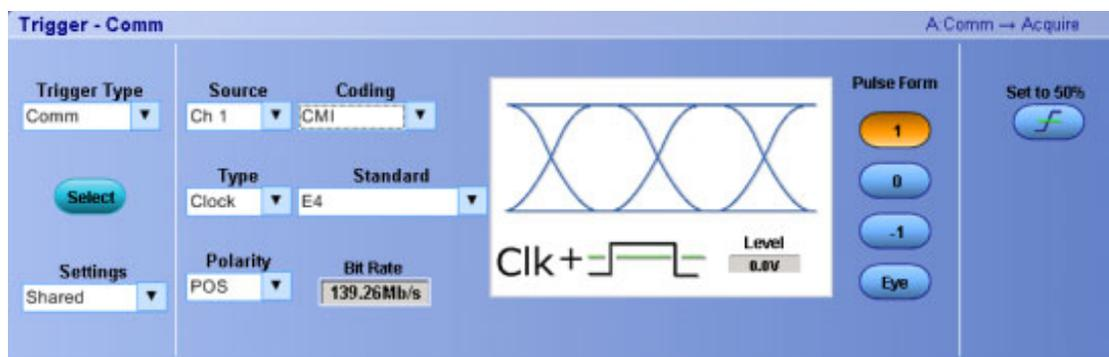
Depending on which coding format you use, you can also change the Upper, Lower, and Clock level thresholds and the pulse form using the multipurpose knobs.
