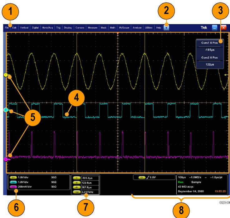
1. **Menu bar:** Access to data I/O, printing, online help, and instrument functions.
