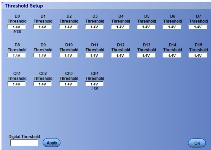
This is an example of the Threshold Setup dialog box for a 4-bit parallel bus.
