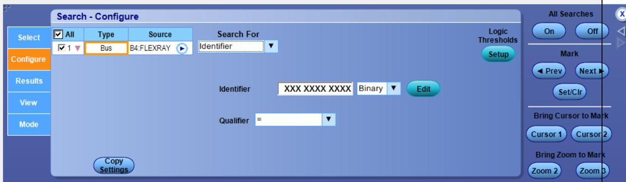
Select the Identifier from the drop-down list. Click Edit to enter the value. Click Logic Thresholds to adjust the logic thresholds.
