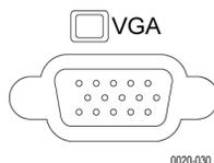
Use this VGA port to connect a monitor for extended desktop operation. For example, use the front panel to display the contents of the instrument, and use an additional monitor for Windows operation.
