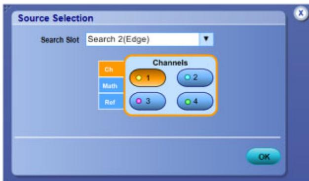
Use the dual Source Selection window to set the Clock and Data Source parameters for a Setup and Hold search.
