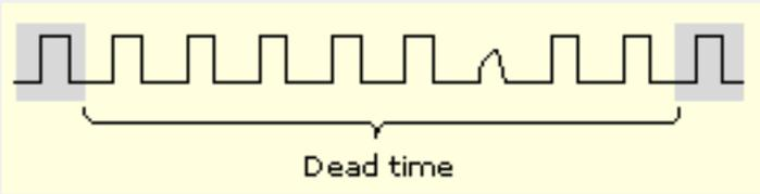
The instrument cannot acquire any new data until the previous data has been processed. If dead time is long, the instrument can miss acquiring infrequent events.
