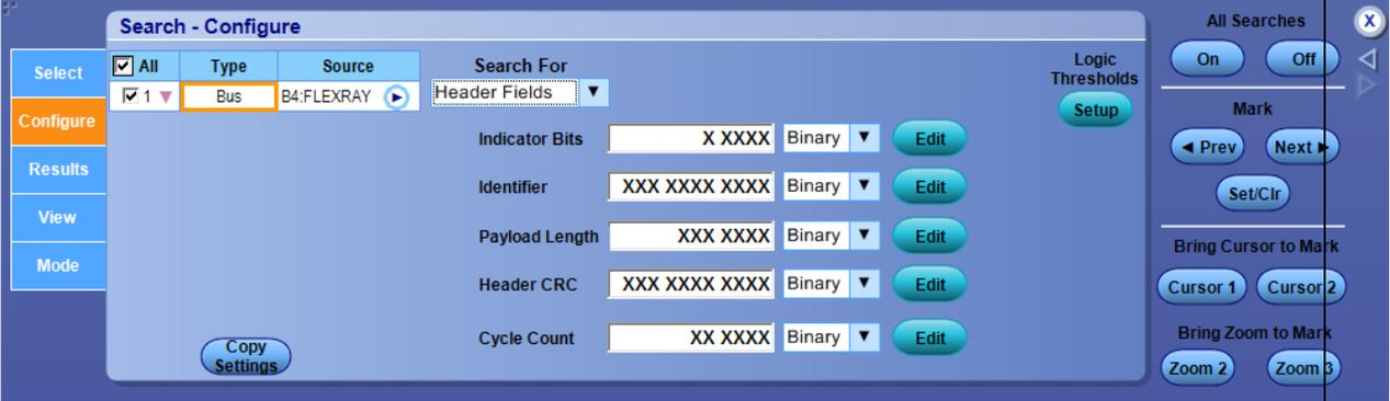
Click Edit to enter the data value. Click Logic Thresholds to adjust the logic thresholds.
