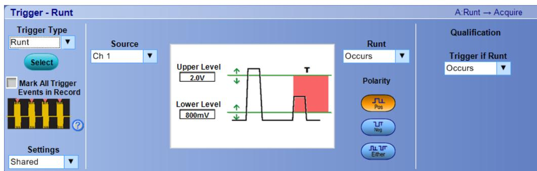
The following Trigger Runt screen appears on MSO/DPO5000B Series instruments:
