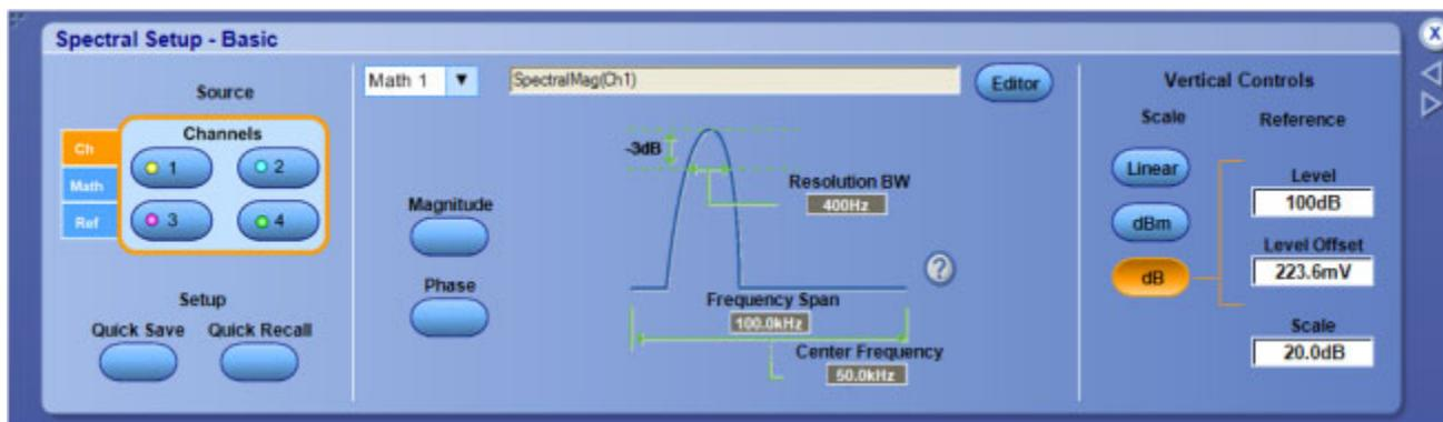
Changing the Horizontal Mode to Manual activates the Frequency Span and Resolution BW controls.
