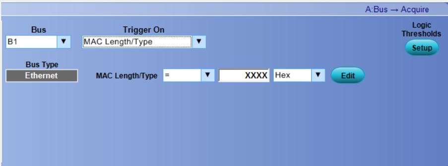
The screenshot shows a configuration window titled "A: Bus → Acquire". It has a "Bus" dropdown set to "B1" and a "Trigger On" dropdown set to "MAC Length/Type". Below this, there is a "Bus Type" section with "Ethernet" selected. A row for "MAC Length/Type" is visible, with a dropdown set to "=", a text input field containing "XXXX", a "Hex" dropdown, and an "Edit" button. In the top right corner, there is a "Logic Thresholds" section with a "Setup" button.
