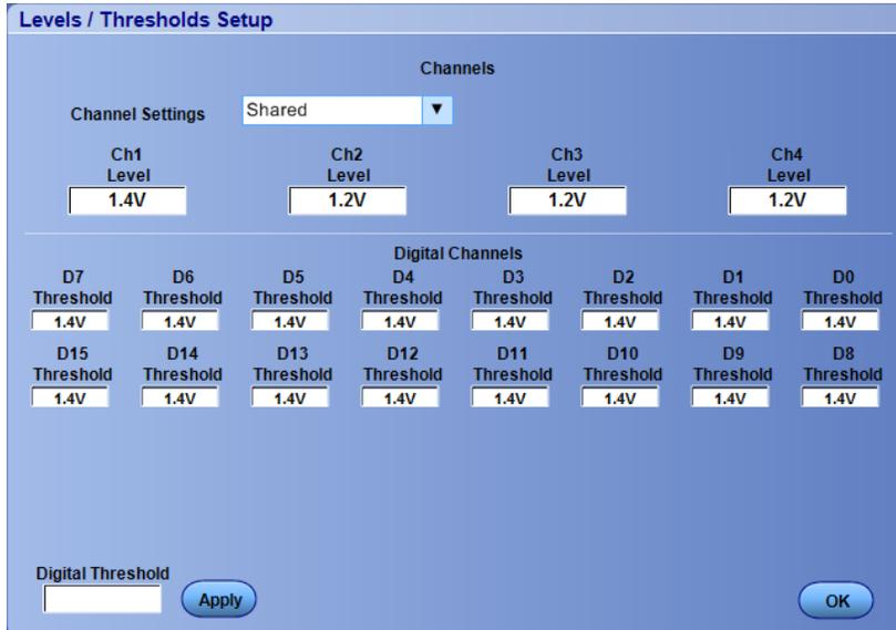
The instrument displays a different Threshold Setup dialog box for each type of bus defined: parallel or serial types.
