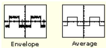
**Average.** This mode acquires and displays a waveform record that is the average result of several acquisitions. This mode reduces random noise. Use the multipurpose knobs to specify the number of waveforms that you want to average.
