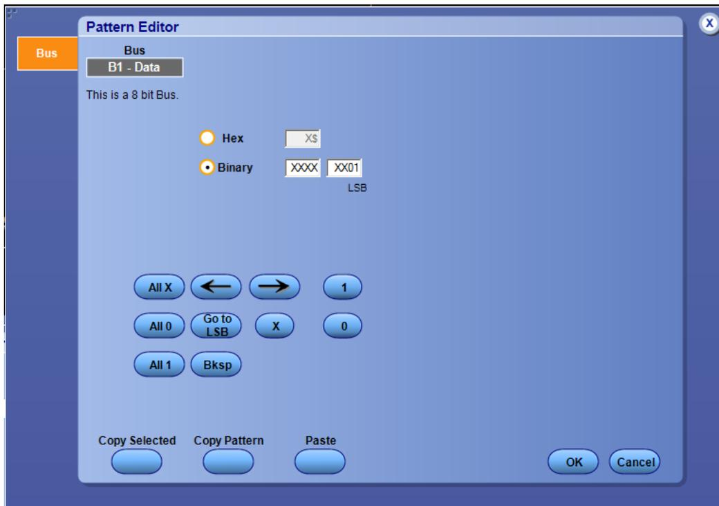
Select a bus I2C (with Trigger On set to Address or Addr+Data) or USB (with Trigger On set to Token Address Packet or Data Packet) and click the Edit button. The Bus field would display the text depending
