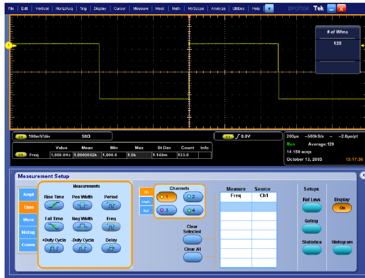
Figure 38: Measurement of probe compensator frequency
