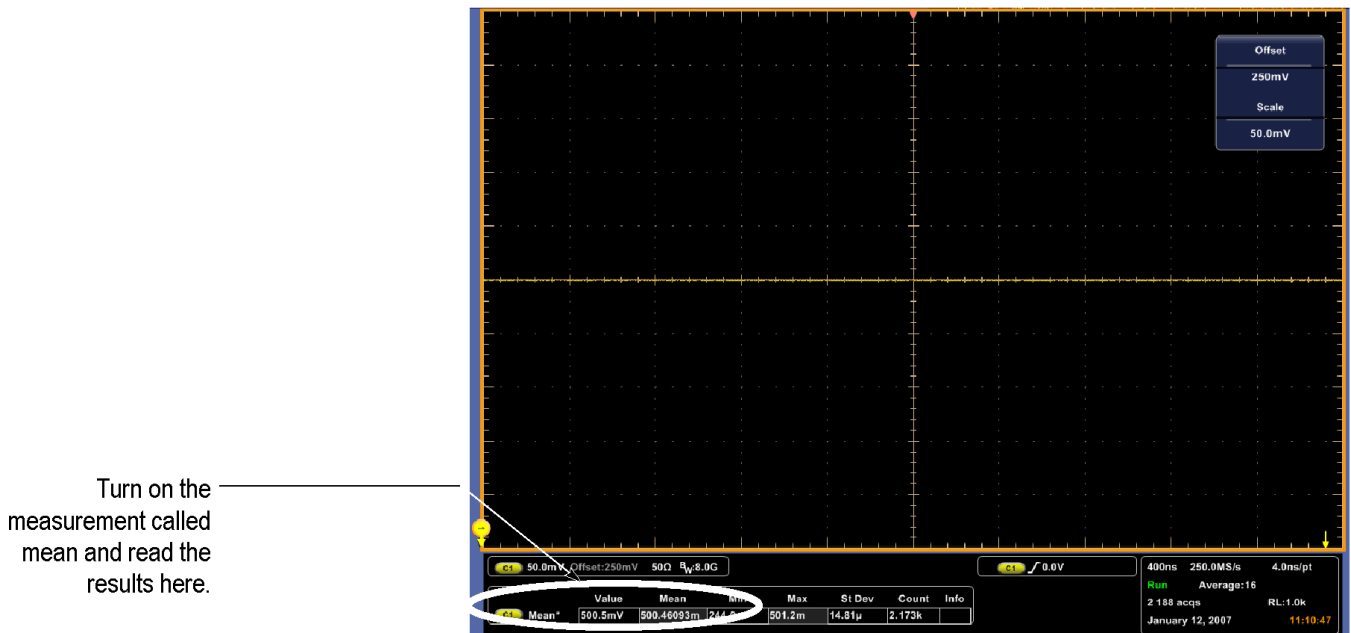
Figure 17: Measurement of offset accuracy
