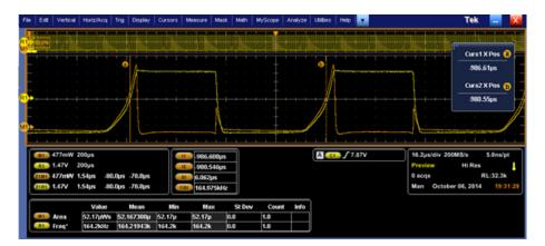
In summary, you cannot directly compare values from plot to scalar results. To compare between plot cycle and results value, you need to add all values for TON and TOFF separately. Enable dot connect, as shown below, add all yellow points which corresponds to ON region, then multiply by sample interval to get particular energy.
