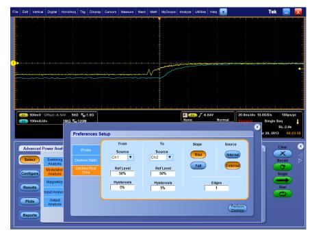
**9.** Use Ch1 as the reference point and deskew the remaining channels. The following figure shows a waveform before and after deskew.
