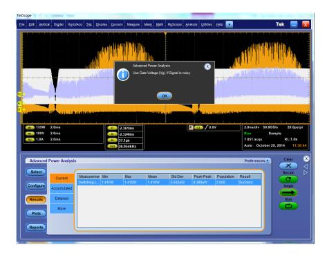
**3.** If the application detects ringing with Vg and pops up error message, then adjust REF level as described in *REF level computation for noisy VG source*.
