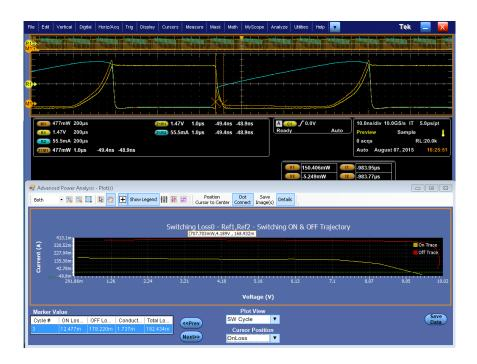
• OffLoss: The selected switching cycle Turn-off loss is zoomed and the scope cursors are placed between start and stop of Turn-off loss region. .
