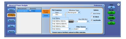
Select the Filter check box, and then select one PoE specific filter from Type drop-down and Math Filter Source. After selecting Filter, navigate to the Source configuration tab and perform the "Vert&Horiz" auto set.
