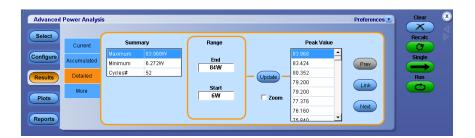
Summary results can be current and accumulated. Current shows the results for the current acquisition. Accumulated shows the statistics of all acquisitions (previous and current). Select the Accumulated tab to view the summary of the measurement.
