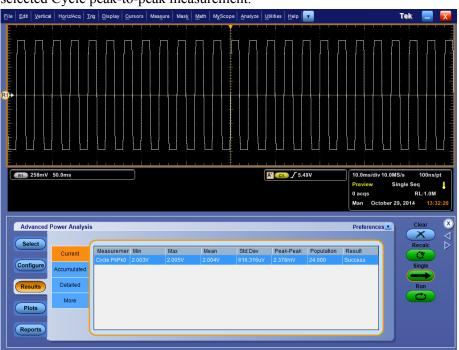
Viewing results-Cycle peak-to-peak. Click Results to view the result for the selected Cycle peak-to-peak measurement.
