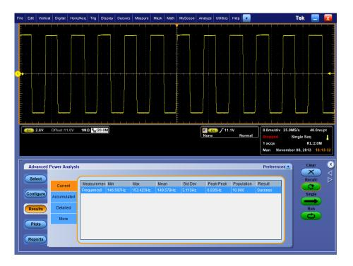
**Viewing results-Frequency.** Click Results to view the result for the selected Frequency measurement.
