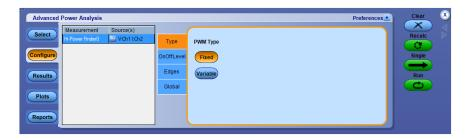
1. Click the Variable button if a switching device operates with a variable Duty Cycle with or without Discontinuous Conduction Mode. If the Variable option is selected, the voltage edge source selection in the On-Off Level tab switches to Vg (gate drive signal). If the Fixed option is selected, the application measures the switching loss for all the topologies with a constant duty cycle.
