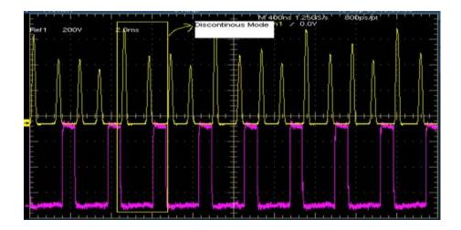
**Viewing results-Switching loss.** Do not disturb the oscilloscope settings during the post analysis of the results. Changing settings will put the oscilloscope into Preview mode. This could lead to incorrect interpretation of results.
