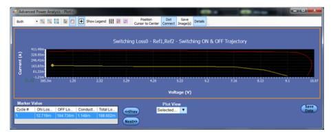
Observe that scope built-in area measurement with cursor gating turned on is  $\sim$  75.32nWs. This matches with energy of TON statistics.
