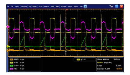
If the signal (Push Pull device) is similar to the one shown in the previous figures, configure the Ref level only at the switching portion of the voltage. The switching occurs only at the lower portion of the switch voltage. Enter the Ref value as 30% which falls midway between the lower switching portion.
