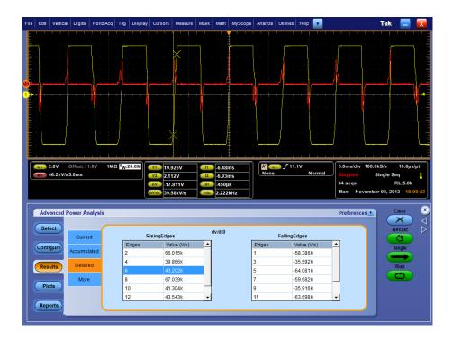
**3.** The application displays the results, which is a differential of the voltage waveform with respect to time in units of volts per microsecond.
