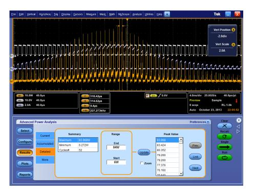
The results display the instantaneous peak power in the switching and the number of peaks in the acquired data. Select the range of interest to view the area of interest in the instantaneous peak power.
