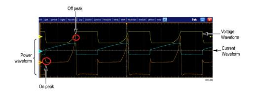
Concept to identify TOn and TOff using gate voltage for edge analysis:
