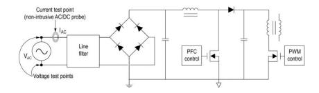
Figure 22: SMPS circuit diagram
