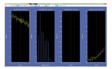
**Flow view.** The plot window arranges plots based on the size. By default plots are aligned in single row. You can adjust the size of the plot window to change the configuration to see the selected plots. For example below Flow view displays four plots arranged in single row (4\*1). Flow view is useful to view one plot at a time.
