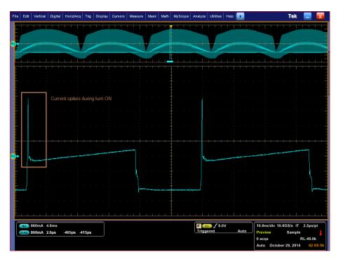
Figure 23: Current spikes during turn ON
