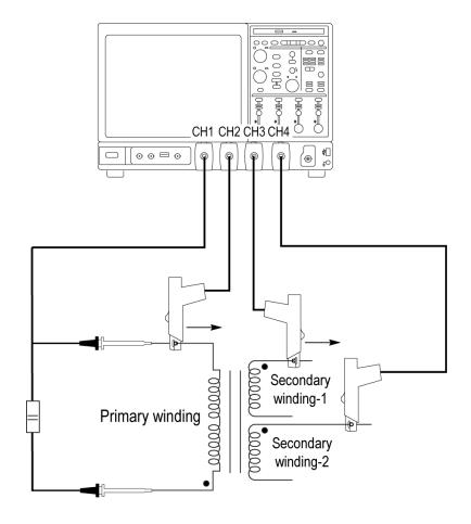
voltage probe should be connected so that the voltage is read as positive when the current rises.
