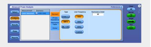
**NOTE.** Source Autoset takes input from Line Frequency and Harmonic Order. To set the minimum acquisition of sixty cycles of line frequency, run the source autoset Vert & Horiz.
