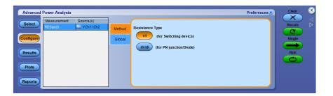
2. There are two methods, first method is V/I, which is a ratio of instantaneous voltage and current samples. This is suitable for switching devices. The second method is dV/dI, which is ratio of rate of change of voltage and current. This is suitable for PN junctions and diodes.
