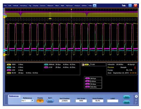
Figure 42: VDS, IDS and VG overlapped
