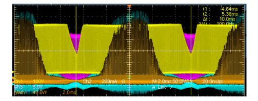
It is recommended to use gate voltage as edge source in case of PFC topology for post-processing. The switch voltage can vary in duty cycle and operating frequency as shown in the following image. The switch voltage can operate in
