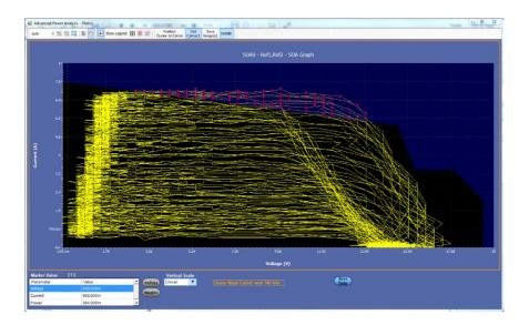
SOA Plot gives information about current vs voltage waveforms and mask. When user selects the point on SOA plot, it creates the list of points nearby region and updates the Marker value Table. It also zoom the region on scope, where this points present in time domain. User can travels through Marker Value Table points in various cycles. It allows to analyze waveform region on oscilloscope, where waveform violates the mask coordinates.
