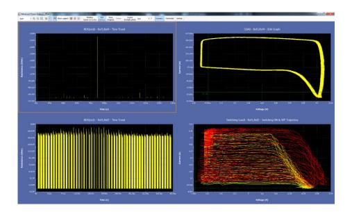
**NOTE.** A maximum of four plots can be added, and they are displayed in a single window. Double-clicking the plot will toggle between full screen and compact size. See Plot components and features for additional details.
