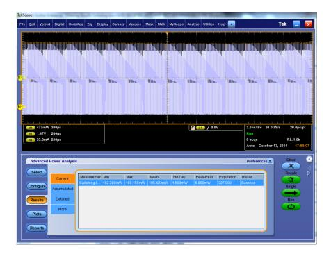
Select Analyze > Advanced Power Analysis > Results, from the oscilloscope menu bar, and then press Detailed for detailed results. Detailed result shows TON, TOFF and Conduction loss and energy statistics.
