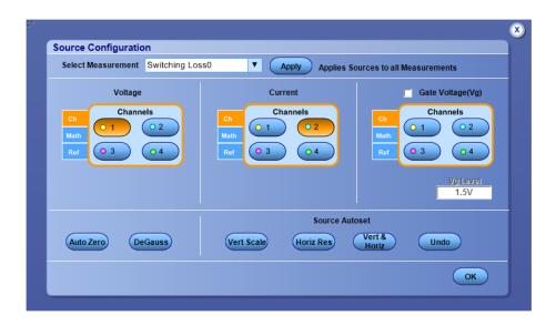
**NOTE.** Autoset accounts for the deskew value. If the deskew value is less than the sample interval set by autoset, then the deskew value is rounded to 0.0 s by the oscilloscope. This can be seen in the Vertical >Deskew menu. In this situation, it is recommended that you use a higher sample rate.
