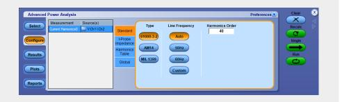
**NOTE.** Source Autoset takes input from Line Frequency and Harmonic Order. To set the minimum acquisition of ten cycles of line frequency, run the source autoset Vert & Horiz.
