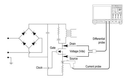
Figure 19: Equipment connection setup for Hi-Power finder
