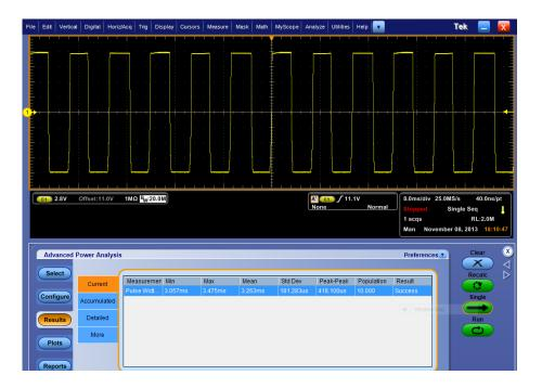
**Viewing plots-Pulse width.** Click Plots and select Time Trend to view the plots for the selected Pulse Width measurement.
