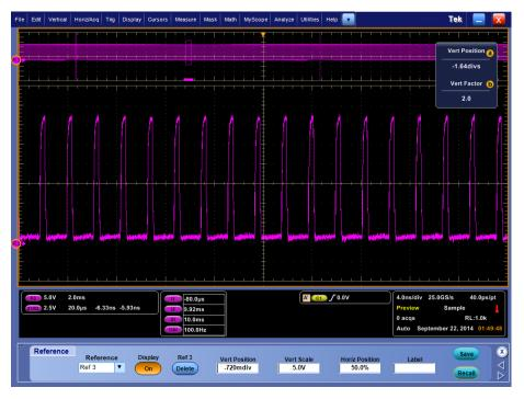
Figure 41: Zoom-in of the (VG)Gate Voltage
