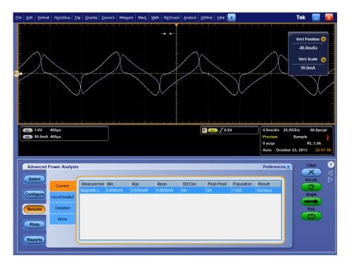
6. Press Run to measure and display the result shown below:
