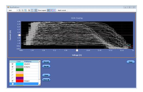
The X-axis represents the voltage values in volts and the Y-axis represents the current in amperes.
