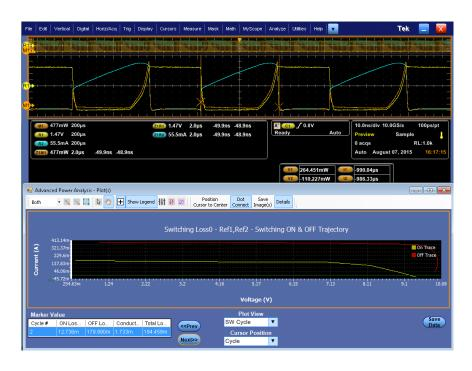
OnLoss: The selected switching cycle Turn-on loss is zoomed and the scope cursors are placed between start and stop of Turn-on loss region.
