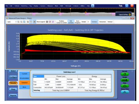
Figure 27: Measurement results and switching loss plot
