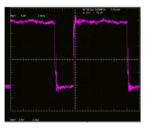
If you select the Vg option button in the Edge Finder tab, the gate voltage should be a clean pulse without any glitch or ringing as shown in the previous figure. The gate voltage is used to identify the edges, TOn or TOff portions. When a glitch occurs, the application displays incorrect results. This type of signal can result in multiple edges (wrong edges) within a switching cycle.
