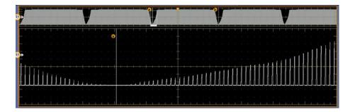
Switching waveforms with cursors near zero crossing
