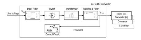
Figure 21: SMPS block diagram
