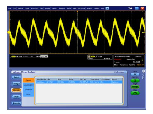
**Viewing results-Switching ripple.** Click Results to view the result for the selected Switching Ripple measurement.
