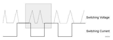
Figure 32: Discontinuous switching mode
