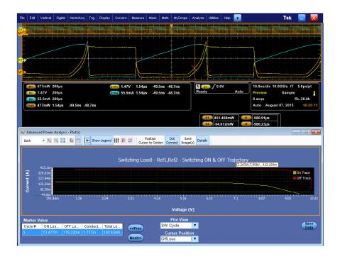
ConductionLoss: The selected switching cycle conduction Loss is zoomed and the scope cursors are placed between stop of Turn-on and start of Turn-off.
