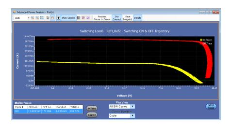
The Plot View allows you to view the plots for all cycle and single cycle based table values.
