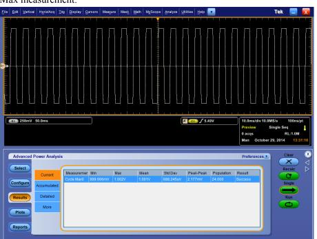
**Viewing results-cycle max.** Click Results to view the result for the selected Cycle Max measurement.
