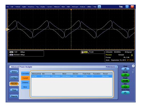
**Viewing results - I vs**  $\int$ **V.** Click Results to view the result for the selected I vs  $\int$ V measurement.
