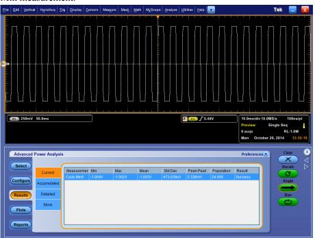
**Viewing result-cycle min.** Click Results to view the result for the selected Cycle Min measurement.
