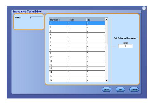
Use the Impedance table to set the transfer impedance of the probe at each harmonic frequency. The table editor displays the Harmonic Number from 1-40 for IEC standard and 1-50 or 1-100 (based on the configuration parameter selected) for MIL standard, the Impedance ratio and the Impedance ratio in decibels.
