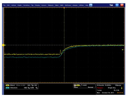
Figure 2: Waveform after deskew
