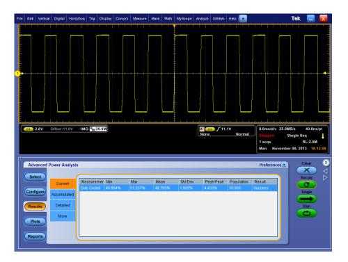
**Viewing plots-Duty cycle.** Click Plots and select Time Trend to view the plots for the selected Duty Cycle measurement.
