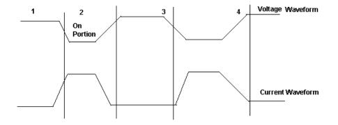
Total Switching Loss=Ton Loss+Toff Loss+Conduction Loss.
