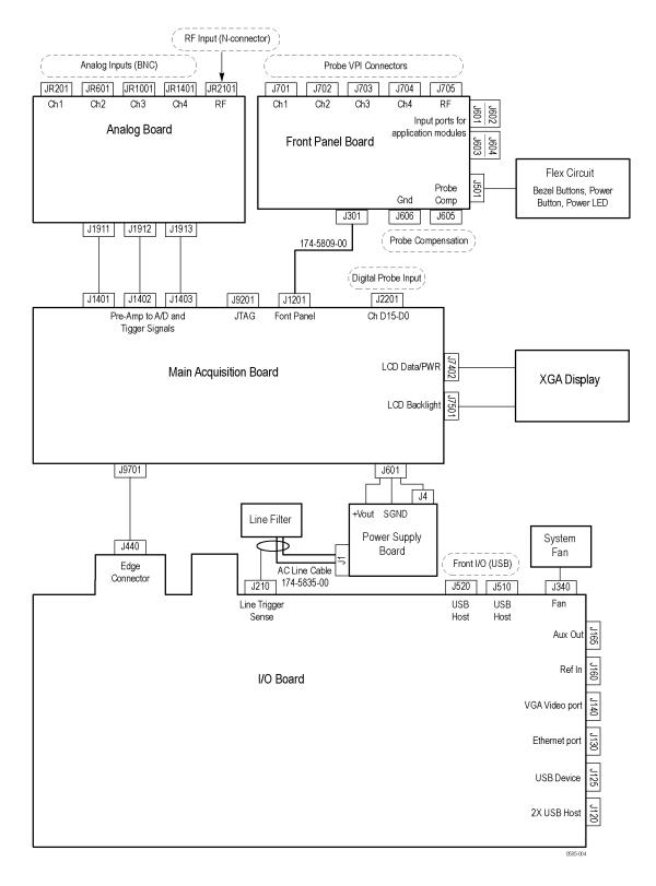
Figure 1: MDO4000 Series block diagram
