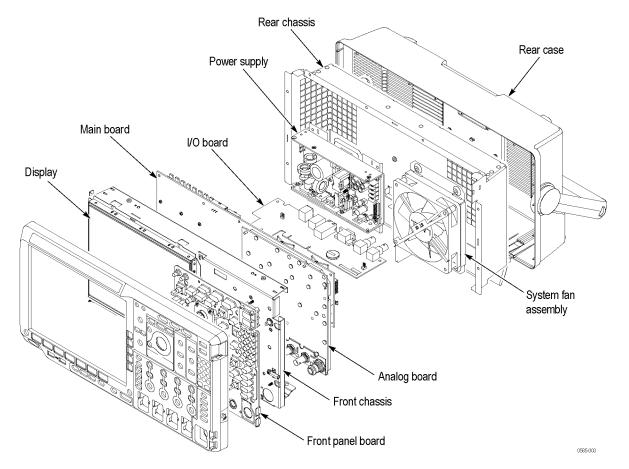
Figure 3: Module locator
