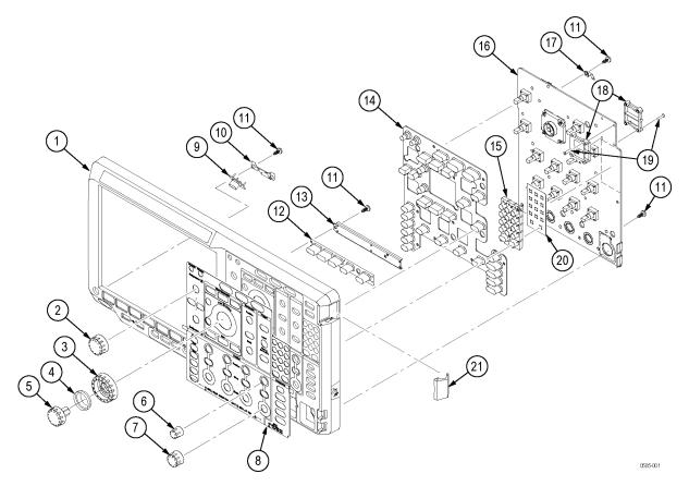
Figure 7: Exploded view, Front Panel assembly
