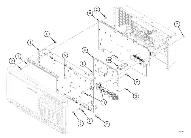
Figure 8: Display, analog board, and main board assembly
