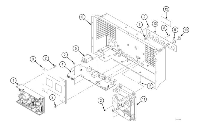
Figure 9: Rear chassis and connecting modules
