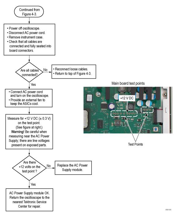
Figure 5: AC power supply troubleshooting procedure
