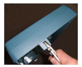
Figure 2: Removing tabs from the front protective cover
