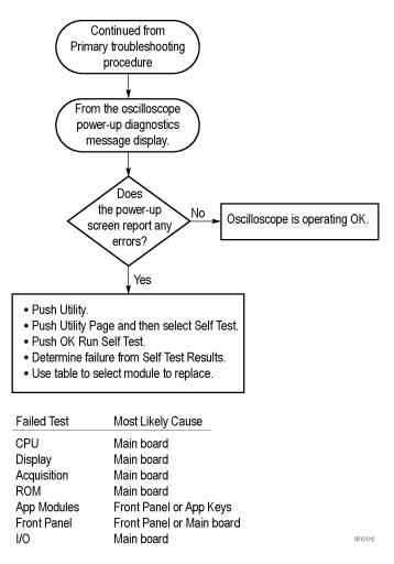
Figure 6: Module isolation troubleshooting procedure
