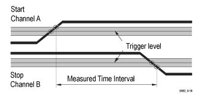
The hysteresis band is about 20 mV at 1x attenuation, and 200 mV at 10x attenuation
