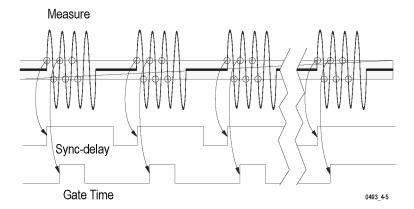
After the set measurement time has started, the instrument synchronizes the start of the measurement with the second trigger event in the burst. This means that the measurement does not start erroneously during the Burst Off duration or while inside the burst.
