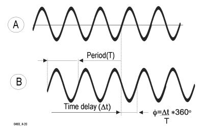
The traditional method to measure phase delay with a timer/instrument is a two-step process consisting of two consecutive measurements; a period measurement followed immediately by a time interval measurement. The phase delay is then mathematically calculated as:
