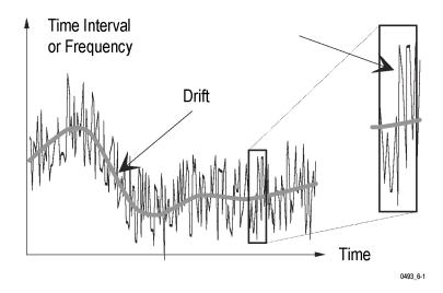
To measure the slower variation, calculate the Max, Min, or Mean values on a long series of averaged samples. Averaging eliminates the jitter in each sample and the long measuring time and large number of samples means that the measurement can record very slow variations. The maximum pacing time is 500 s, the maximum measuring time for each sample is 1000 s, and the maximum number of samples is  $2*10^9$ .
