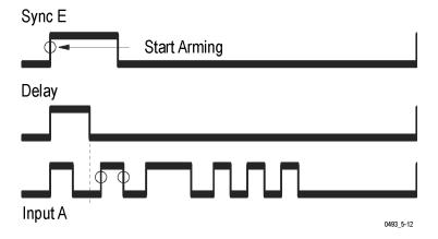
Use the same procedure as in the preceding example but set a suitable **Start Arm Delay** so that delay expires in the gap between the first and second pulse.
