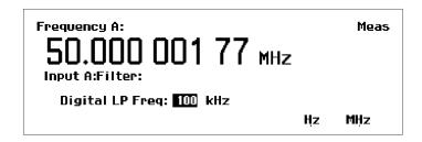
You should be aware of a few limitations with using the digital filter feature effectively and unambiguously. First you must have a rough idea of the frequency to be measured. A cutoff frequency that is too low might give a perfectly stable reading that is too low. In such a case, triggering occurs only on every 2nd, 3rd, or 4th cycle. A cutoff frequency that is too high (>2 times the input frequency) also leads to a stable reading. Here one noise pulse is counted for each half-cycle.
