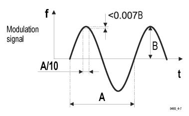
Figure 8: Error when determining fmax
