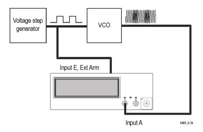
Figure 11: Setup for transient profiling of a VCO.
