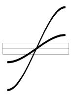
Wrong counts caused by trigger errors are much more common. To avoid incorrect counting caused by spurious signals, reduce input signal amplitudes. This is particularly true when measuring on high impedance circuitry and when using  $1 \text{ M}\Omega$  input impedance. Under these conditions, the cables easily pick up noise.
