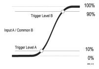
The instrument calculates and sets the trigger levels. Rise and fall time can be measured on both Input A and Input B.
