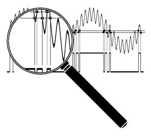
A wider trigger hysteresis provides correct triggering and mesurements on variable-level and noisy signals.
