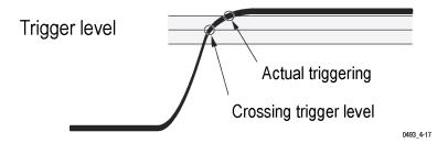
**Overdrive.** When the input signal crosses the hysteresis band with only a marginal overdrive, triggering may take some 100 ps longer than usual. The specified worst case 500 ps systematic trigger error includes this error. To avoid this error, make sure that the input signal or trigger level has adequate overdrive.
