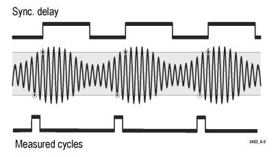
The **PRF** readout shows the modulating frequency even though the main frequency reading may be unstable.
