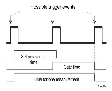
**RF signals (FCA3003, FCA3020, FCA3103, FCA3120).** The C-input prescaler divides the input frequency before it is counted by the normal digital counting logic. The division factor is called *prescaler factor* and can have different values depending on the prescaler type. The 3 GHz prescaler is designed for a prescaling factor of 16. This means that an input C frequency of, for example, 1.024 GHz is transformed to 64 MHz.
