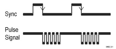
You can delay the start arming point with respect to the arming signal. Use this function when the external arming signal does not coincide with the part of the signal in which you are interested. The time delay range is 20 ns to 2 s with a setting resolution of 10 ns.
