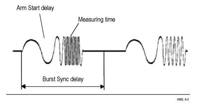
Figure 6: Three time values must be set to measure the correct part of a burst
