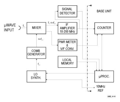
Figure 5: Microwave acquisition in the MCA3000 Series.
