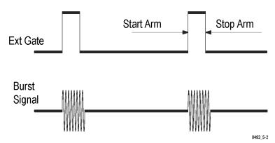
The available Arm Stop parameters are Channel, Slope, and Delay.
