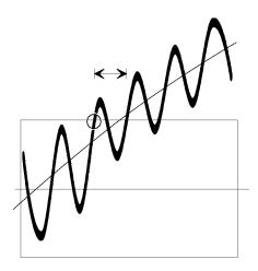
To reduce trigger uncertainty, the signal needs to cross the hysteresis band as fast as possible (high slew rate). A high amplitude signal passes the trigger hysteresis band faster than a low amplitude signal. For low frequency measurements where the trigger uncertainty is of importance, do not attenuate the signal too much, and set a high instrument sensitivity level.
