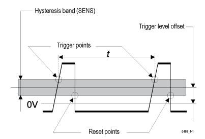
Frequencies above 100 Hz are best measured using the *Default Setup*. (See page 85, *Default Instrument Settings*.) Then **Freq A** is selected automatically. Other important automatic settings are **AC Coupling**, **Auto Trig** and **Meas Time 200 ms**. The default settings provide a successful starting point for frequency measurements.
