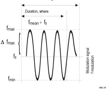
Figure 7: Frequency modulation
