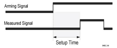
The setup time is different when using arming delay. The following figure shows the time from the expired time delay until the measurement is armed (-60 to +40 ns, for a total of 100 ns delay resolution). The figure shows that a start trigger signal may be detected although it appears 60 nanoseconds before the programmed time delay has expired. The start trigger signal must come 40 nanoseconds after the programmed time delay expires to guarantee correct start of the measurement.
