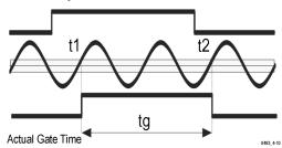
In the same way, the instrument synchronizes the stop of the actual gate time with the input signal, after the set measurement time has elapsed. The multi-register counting technique allows you to simultaneously measure the actual gate time (tg) and the number of cycles (n) that occurred during this gate time.
