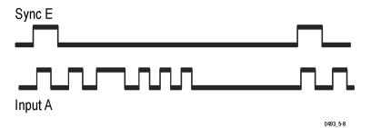
The task is to synchronize the start of the measurement (start trigger) to the leading edge of the first pulse. Depending on the signal timing, this can be easy, difficult, or very difficult.
