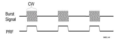
Both the CW frequency, the PRF, and the number of cycles in a burst are measured without external arming signals and with or without selectable start arming delay. (See page 73, *Arming*.)
