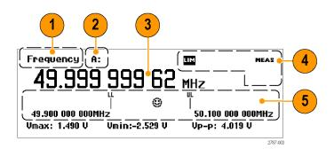
Push the Value button to display a high-resolution numeric readout of the current measurement.
