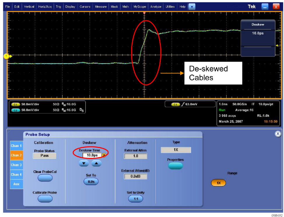
Figure 17: Cable skew adjusted
