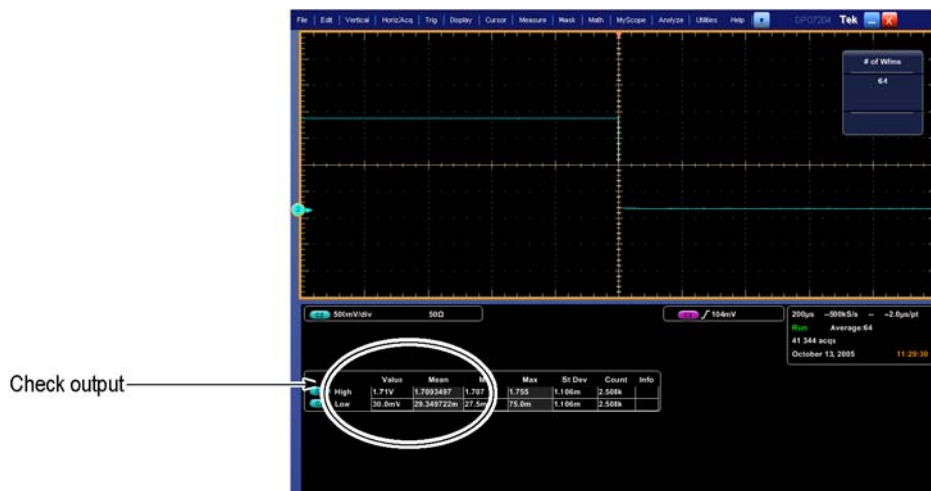
Figure 3-28: Measurement of trigger out limits
