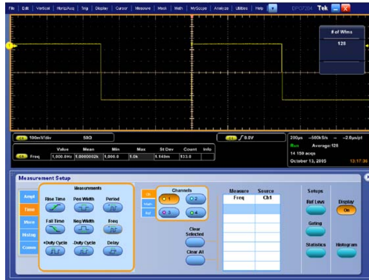
Figure 3-30: Measurement of probe compensator frequency
