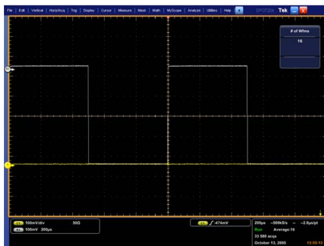
Figure 3-32: Measurement of probe compensator amplitude
