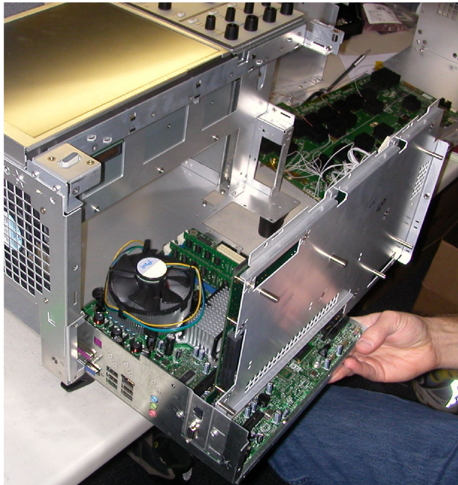
Figure 4-3: Removing the \mu ATX/Power Interface assembly
