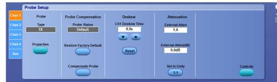
For information on the Probe Setup controls, click the buttons.
