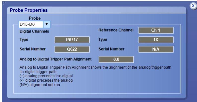
The instrument displays the following information in the Analog to Digital Trigger Path Alignment field:
