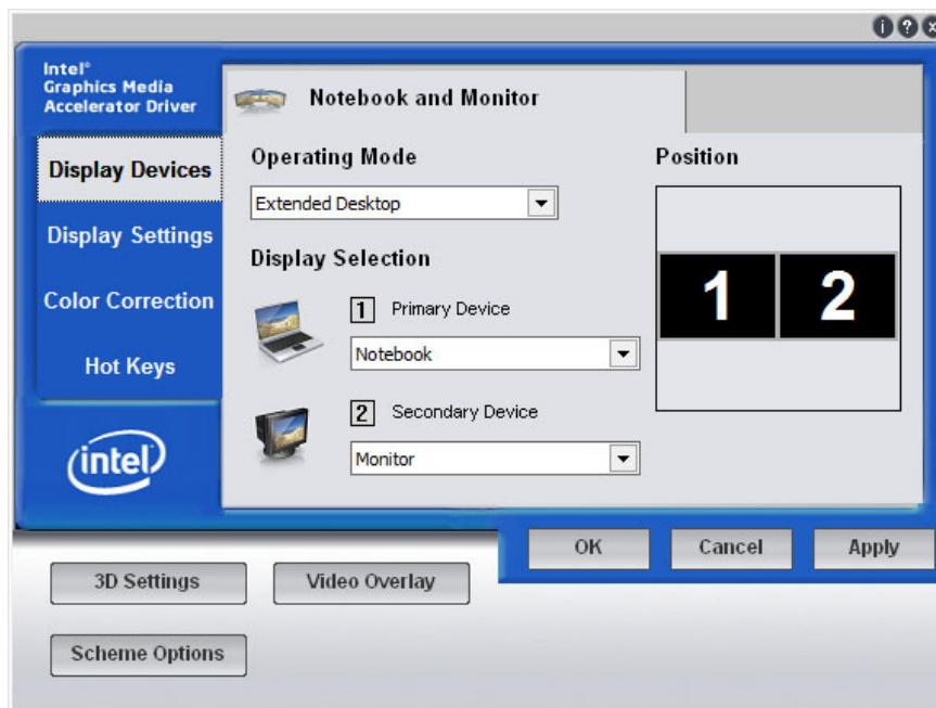
**NOTE.** Do not change the display settings for the internal monitor. The display settings must be 1024 x 768 pixels and colors must be set to 32-bit color. Ensure that the second monitor is also set to 32-bit color. If you use other instrument display settings, the video port may not work properly. However, you can use a resolution setting other than 640 x 480 on the second monitor.
