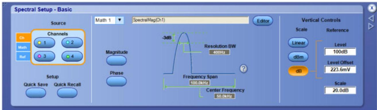
Changing the Horizontal Mode to Manual activates the Frequency Span and Resolution BW controls.
