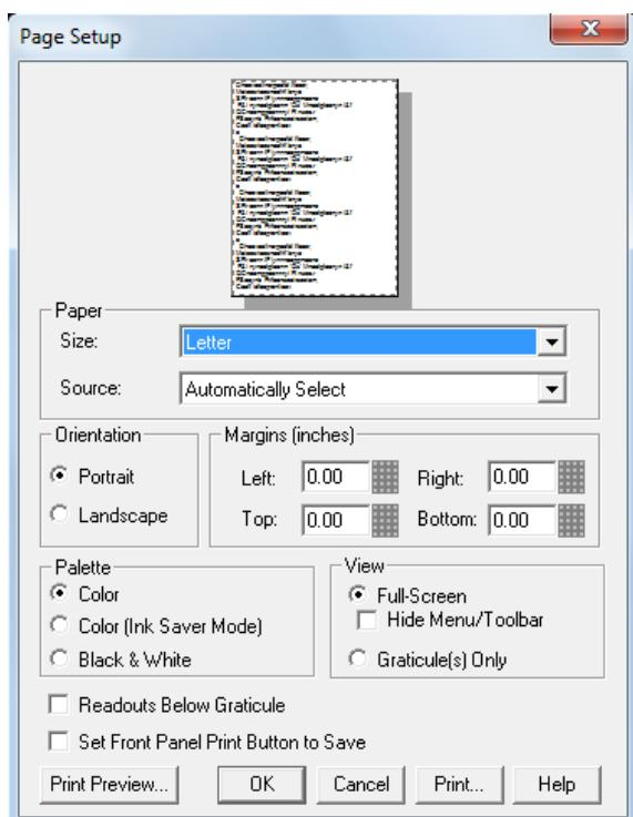
The Paper settings are dependent on the type of printer connected to the instrument. A reduced preview image appears at the top of the window. To view a larger image, click Print Preview at the bottom of the window.
