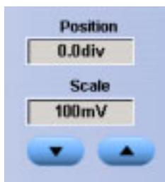
**TIP.** You can also use the dedicated Position and Scale knobs on the front panel to control the position and scale of the selected waveform.
