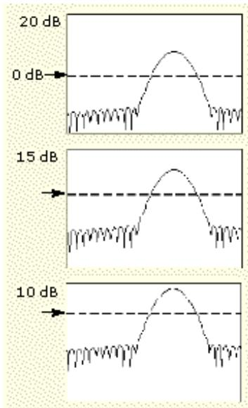
This sets the vertical position of the displayed spectrum. Its value is the magnitude at the top of the display screen. When this control is adjusted, the spectral waveform along with its zero reference marker move vertically on the screen as shown. This control does not change the spectral data.
