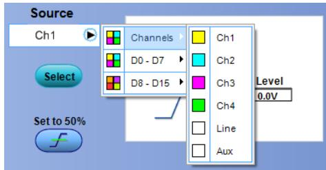
To trigger on an input channel, select a channel.
