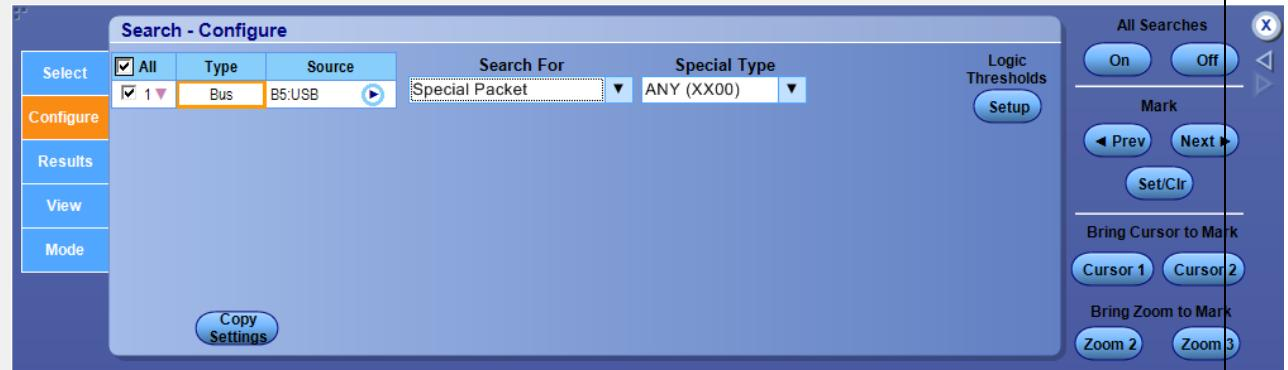
Select the Special Type from the drop-down list. Click Setup to adjust the logic thresholds.
