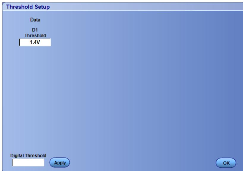
This is an example of the Threshold Setup dialog box for an USB serial bus.
