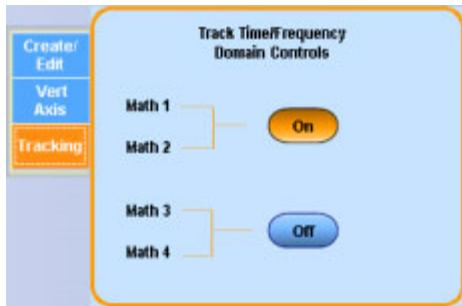
When you lock the spectral controls together, any changes you make to one math waveform are also made to the other math waveform.
