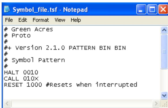
You can create symbol names from ASCII with up to 220 characters. The numeric values must reflect the base specified by the File Radix field. An X represents a “don't care” value. The number of bits represented by each character depends on the radix. For a HEX value, each character represents 4 bits. For an OCT value, each character represents 3 bits. For a BIN value, each character represents 1 bit.
