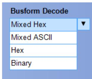
For the Ethernet serial bus, you can display the decode of the bus in Mixed Hex, Mixed ASCII, Hex, and Binary. Select the decode form the drop down list.
