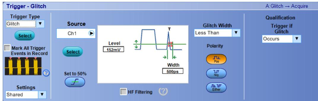
The following Trigger Glitch screen appears on MSO/DPO5000B Series instruments:
