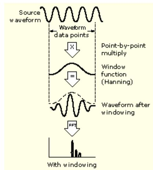
The window functions affect the ability to resolve frequency in the output spectrum and can affect the accuracy of the magnitude and phase measurements. The previous figure shows how the time domain record is processed.
