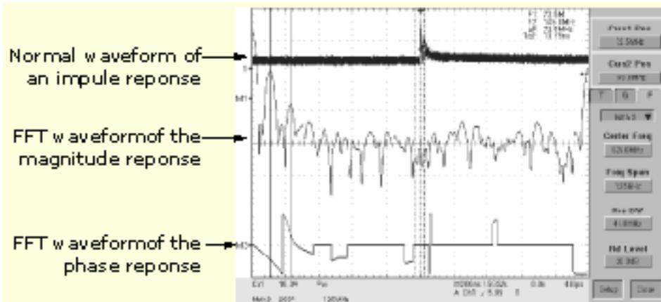
This instrument supports mathematical combination and functional transformations of waveforms it acquires. The next figure shows this concept:
