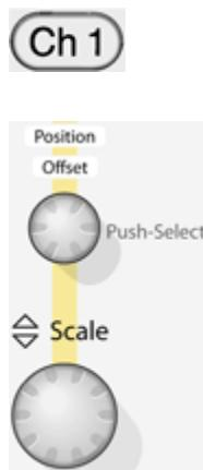
Use the dedicated channel (Ch <1–4>) buttons to turn channel displays on and off. The channel button is lighted when the selected channel is on.
