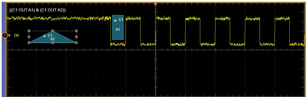
Use the Visual Trigger control window to control which triggered waveforms are displayed.
