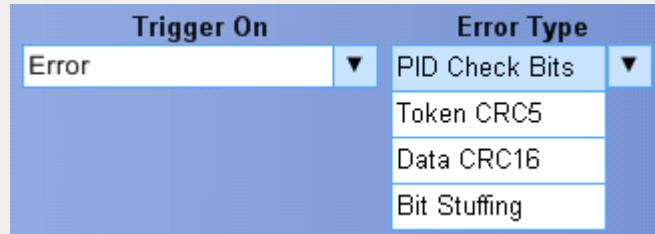
**NOTE.** The Bit Stuffing error type option is not available on high speed bus.
