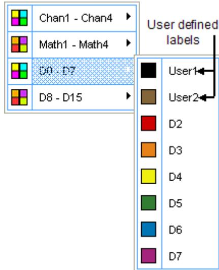
**NOTE.** You have the option to add user-defined labels for the analog, reference, bus, and digital sources. Digital sources are only available on MSO models.
