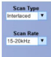
The Scan Rate enables you to trigger on nonbroadcast video signals that have unique scan rates. Select the scan rate range that includes your signal: 15-20 kHz, 20-25 kHz, 25-35 kHz, 35-50 kHz, or 50-65 kHz.
