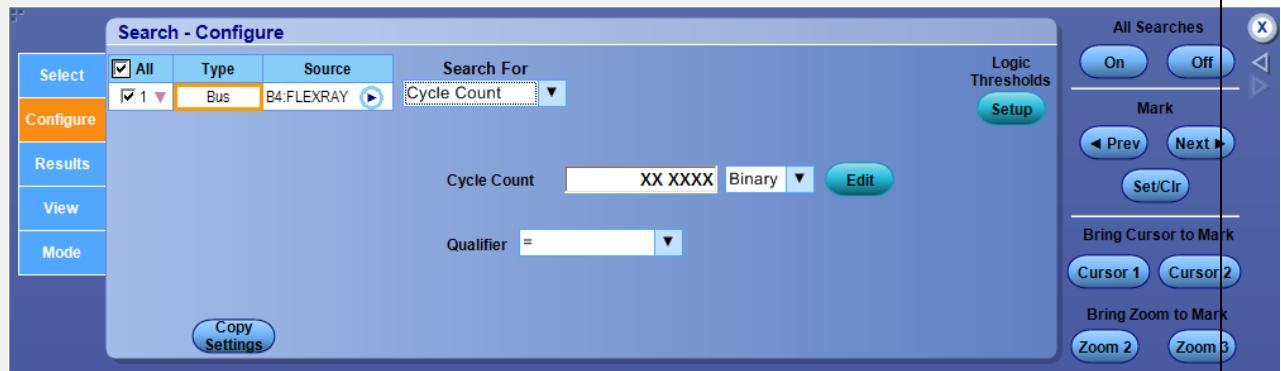
Select the Qualifier from the drop-down list. Click Edit to enter the Cycle Count value. Click Logic Thresholds to adjust the logic thresholds.
