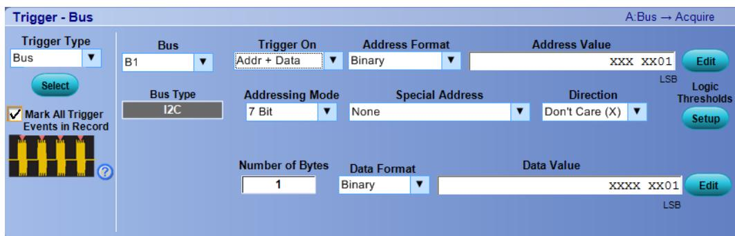
In DPO7000C and MSO7000C/DX Series instruments, when you trigger on an Address for I2C serial bus, there are some predefined patterns termed as Special Addresses. Use this information to debug your serial bus. The following table lists the predefined patterns along with their names.
