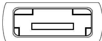
Use the eSATA port as an external interface for SATA support devices.
