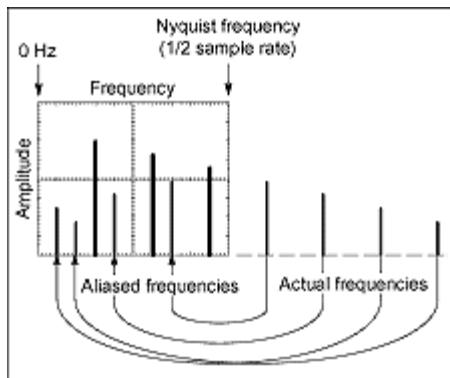
If you have a variable-frequency signal source, another way to observe aliasing is to adjust the frequency slowly while watching the spectral display. If some of the harmonics are aliased, you will see the harmonics decreasing in frequency when they should be increasing or vice versa.
