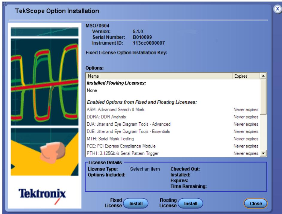
2. Enter the option installation key (provided by Tektronix) in the Options dialog box.
