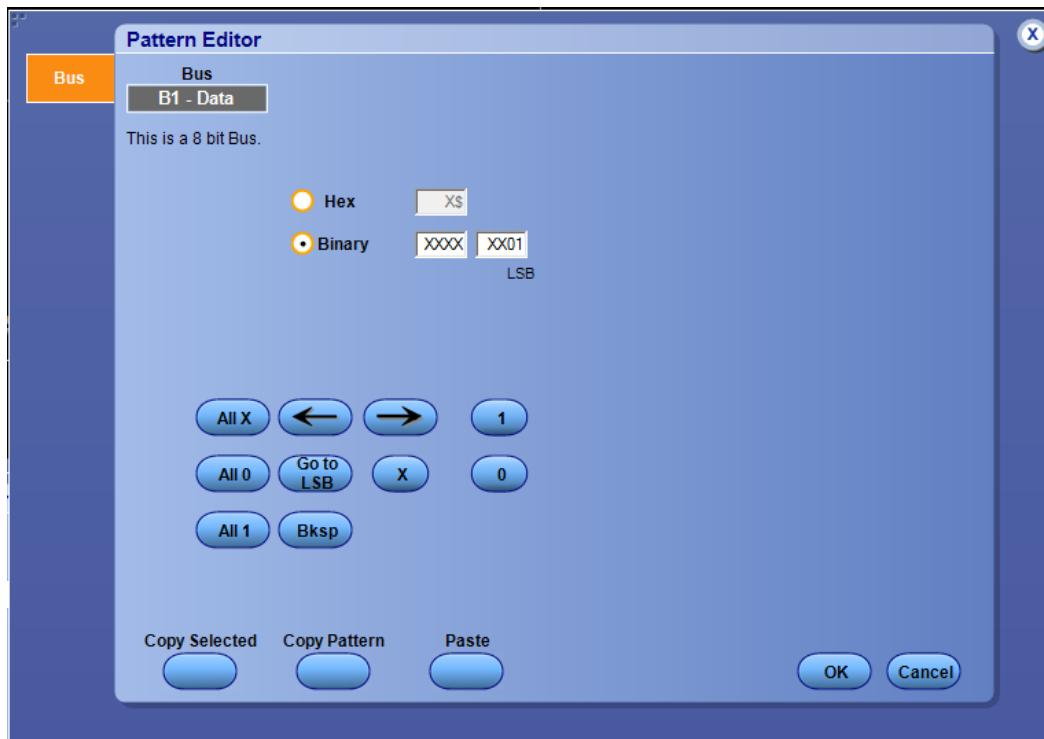
Select a bus I2C (with Trigger On set to Address or Addr+Data) or USB (with Trigger On set to Token Address Packet or Data Packet) and click the Edit button. The Bus field would display the text depending on the type of bus selected (address, data, hub, or port).
