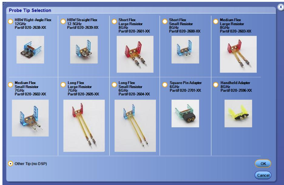
Here is an example of Probe Tip for Tektronix Trimode probe.
