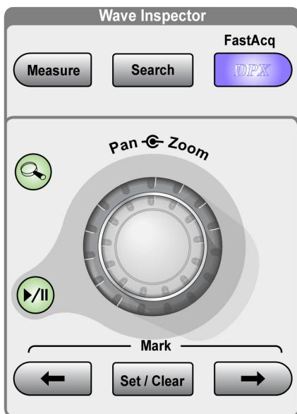
Use Measure to perform automated measurements, Search to search through an acquisition for user-defined events/criteria, or DPX/FastAcq to start or stop fast acquisitions.
