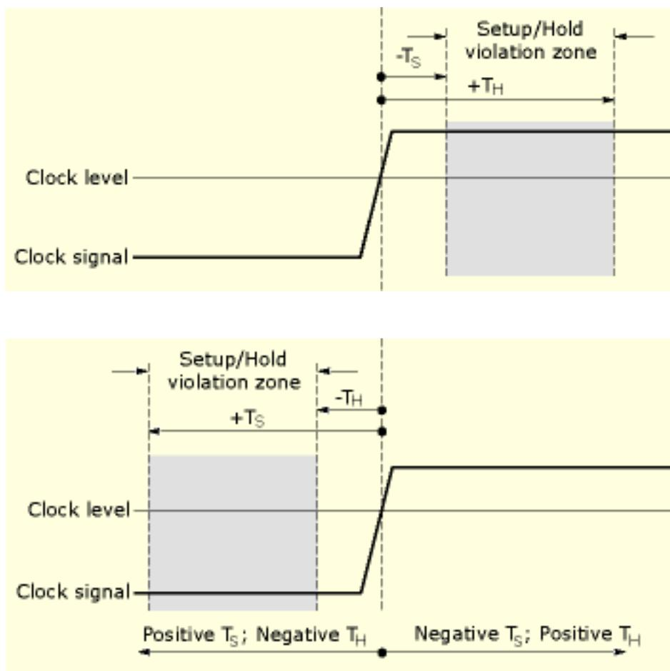
Setup/hold triggering uses the setup/hold violation zone to detect when data is unstable too near the time it is clocked. Each time trigger holdoff ends, the instrument monitors the data and clock sources. When a clock edge occurs, the instrument checks the data stream it is processing (from the data source) for transitions occurring within the setup/hold violation zone. If any occur, the instrument triggers with the trigger point located at the clock edge.
