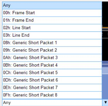
The Search For Short Packet window allows you set the Virtual Channel, Direction, Packet Data Format, and the [Packet Data Value \(see page 941\)](#).
