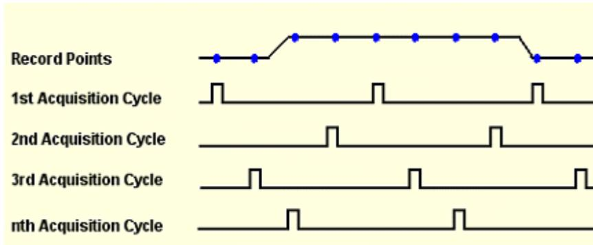
The sampling speeds and the number of channels you choose affect the mode the instrument uses to sample waveforms. The instrument always uses real-time sampling at slower time base settings; faster time settings force the instrument to switch from real-time sampling to equivalent-time sampling.
