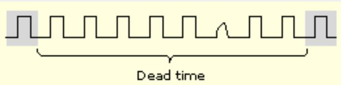
The instrument cannot acquire any new data until the previous data has been processed. If dead time is long, the instrument can miss acquiring infrequent events.
