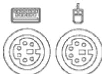
Use the PS-2 connectors to connect a PS-2 keyboard or a mouse to the instrument.
