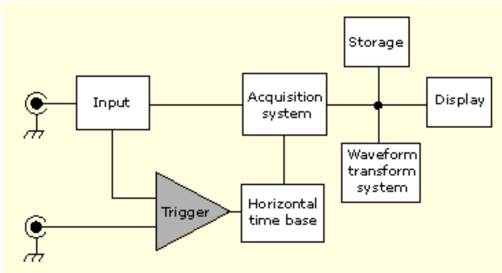
Triggers create meaningful waveforms from signal displays. This instrument has simple edge triggers as well as a variety of advanced triggers.
