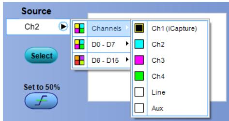
If your instrument has digital channels and, in the Vertical menu you selected an iCapture signal, trigger on a the iCapture channel by selecting the channel.
