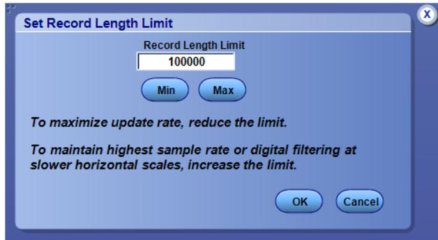
To increase the update rate, lower the record length limit. To enable higher sample rates or digital filtering at slower horizontal scales, increase the record length limit.
