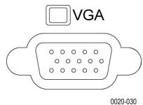
Use this VGA port to connect a monitor for extended desktop operation. For example, use the front panel to display the contents of the instrument, and use an additional monitor for Windows operation.
