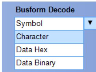
For the PCIe serial bus, you can display the decode of the bus in Symbol, Character Symbol, Character KCode, Data Hex, Data Binary, Descrambled Hex, and Descrambled Binary. Select the decode from the drop down list.
