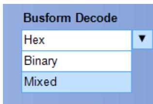
For the CAN serial bus, you can display the decode of the bus in Hex and Binary.
