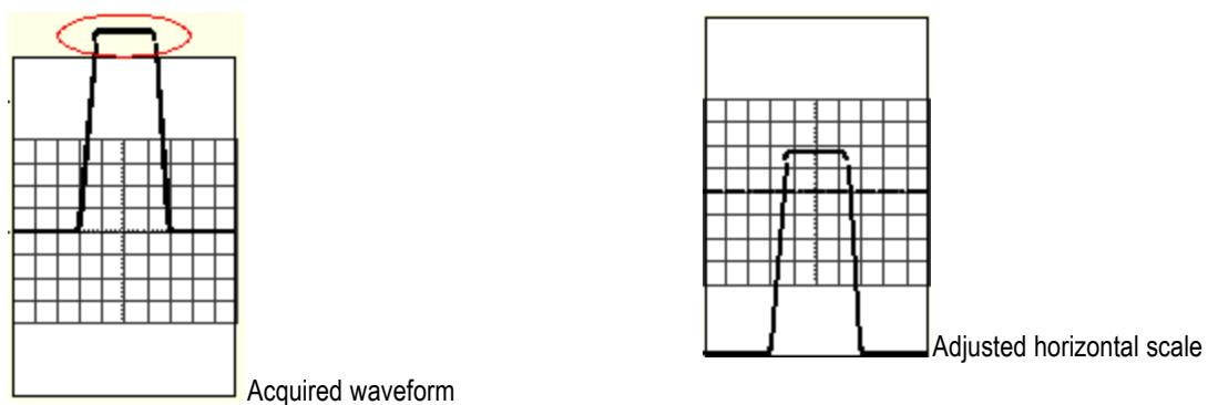
Set the horizontal scale, position, and resolution (record length) to include the acquired waveform record waveform attributes of interest with good sampling density on the waveform. These settings define the horizontal acquisition window, described in [Horizontal Acquisition Window Considerations \(see page 688\)](#).
