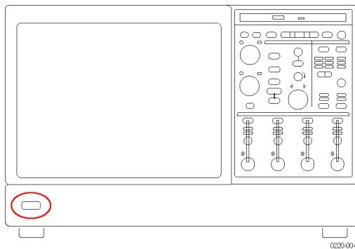
Before shutting down, it is recommended that you first exit the instrument application and any other active Windows applications to avoid error messages on shutdown or the next power on.
