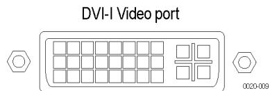
Use the DVI-I Video port (some instruments have a DVI-D Video port) to send the instrument display to a projector or to a flat-panel LCD monitor.
