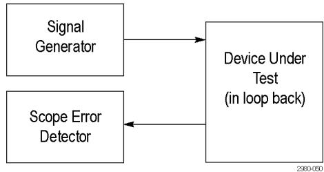
With the DUT inserted between the Signal Generator and the Serial Error Detector, all you need to do to get the Error Detector running is to press the Sync and Run buttons, because the Learn operation was completed in the previous step. If you do another Learn operation, you risk learning errors created by the DUT.
