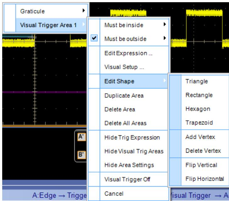
Select Edit Shape to change the shape and orientation of the visual trigger area. Selections include the following:
