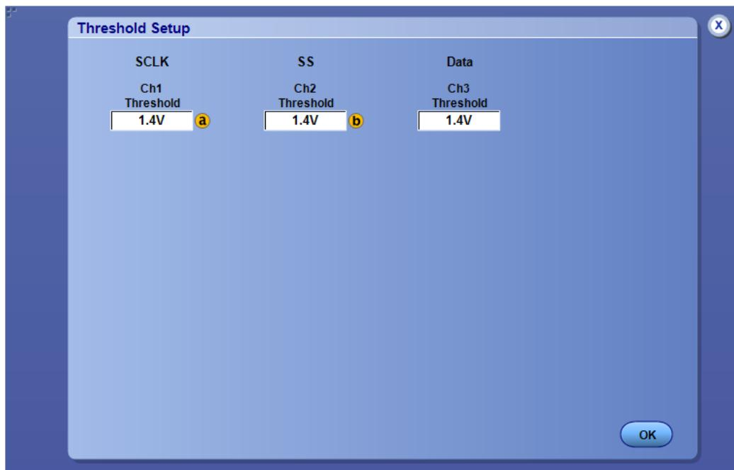
**TIP.** To quickly set the thresholds for all channels to the same voltage level, use the [Global Threshold \(see page 95\)](#) entry box to set the value, and click the Apply button.
