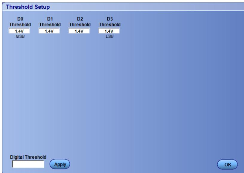
This is an example of the Threshold Setup dialog box for an I2C serial bus.
