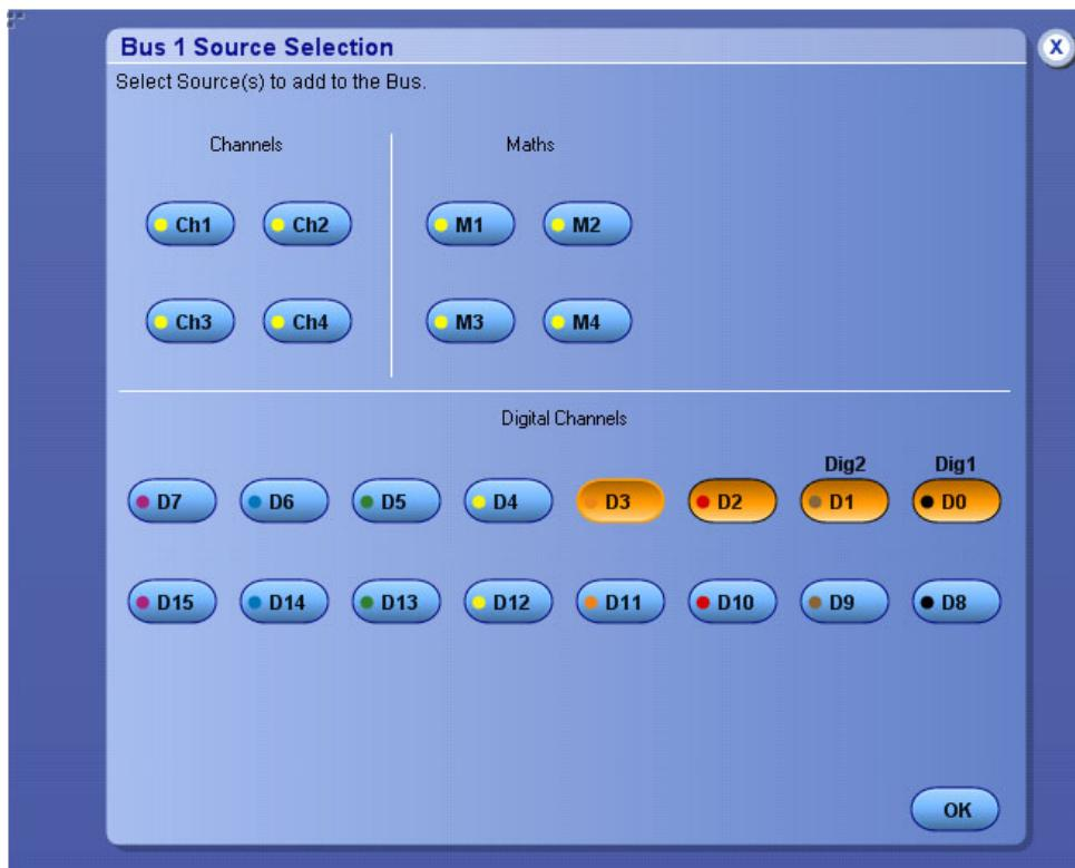
**NOTE.** You have the option to add user-defined labels for the analog, reference, bus, and digital sources. Digital sources are only available on MSO series instruments.
