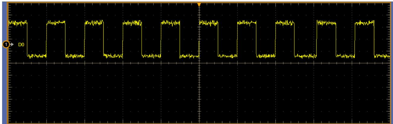
The following screen capture shows the same waveform acquired using edge trigger and visual trigger with two visual trigger areas controlling which triggered waveforms are displayed.
