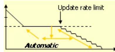
To set the Record Length Limit, click the Advanced button and enter the limit in the Set Record Length Limit dialog box. You can use the buttons or keypad. The instrument will keep the set record length near this limit to produce the best sequence of reduction in sample rate, as the time-per-division is increased.
