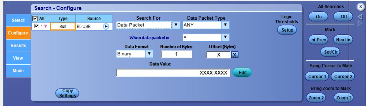
Select the Data Packet Type, When data packet is, Data Format, and Offset from the drop-down lists. Click Edit to enter the data value. Click Setup to adjust the logic thresholds.
