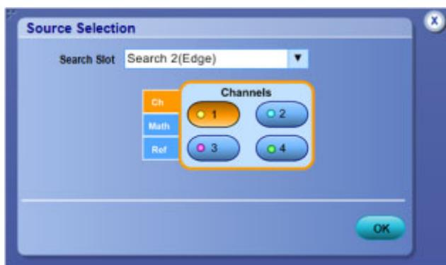
Use the dual Source Selection window to set the Clock and Data Source parameters for a Setup and Hold search.
