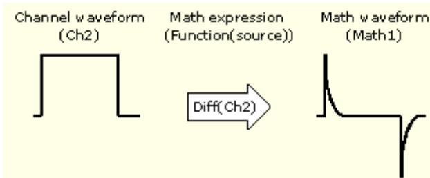
You create math waveforms to support the analysis of your channel and reference waveforms. By combining and transforming source waveforms and other data into math waveforms, you can derive the data view that your application requires. Create math waveforms that result from:
