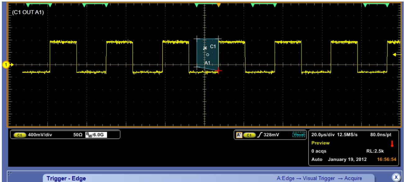
9. The results of the edge trigger and the visual trigger are also displayed in the search results.
