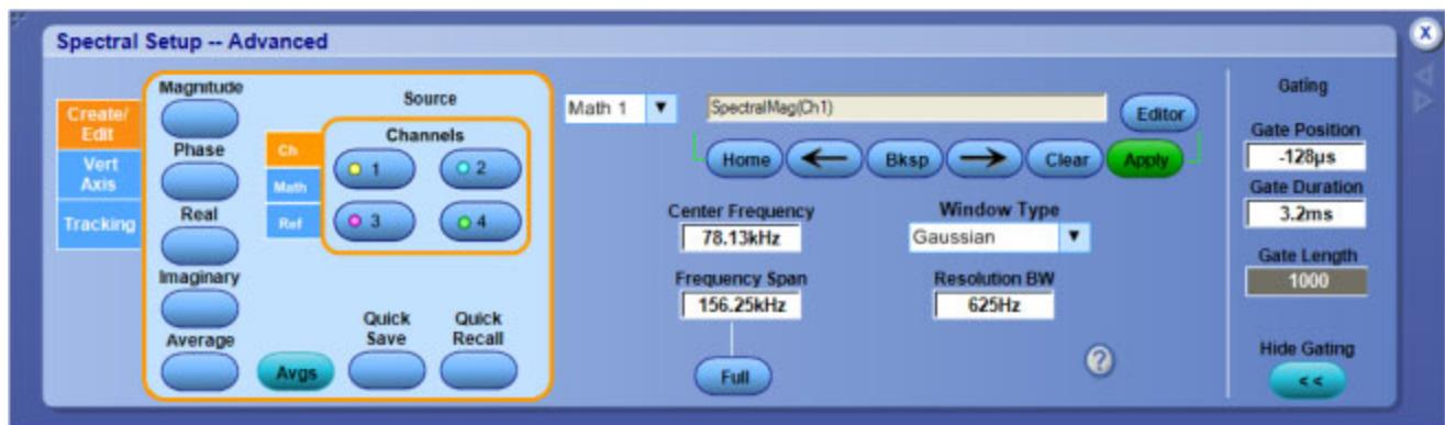
After you create the spectral waveform, use the controls on the right side of the control window to position and adjust the waveform so that you can view the data you are interested in.
