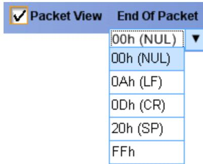
RS-232 decoding displays a stream of bytes. You can organize the stream into packets with an end-of-packet character.
