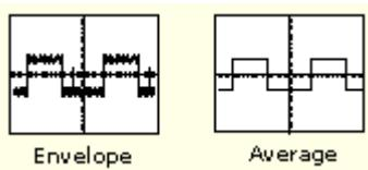
**Average.** This mode acquires and displays a waveform record that is the average result of several acquisitions. This mode reduces random noise. Use the multipurpose knobs to specify the number of waveforms that you want to average.
