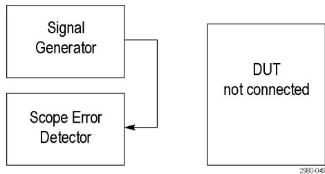
Having done the Learn operation, you can now insert the DUT in-between the Signal Generator and the Error Detector as shown.
