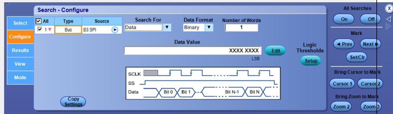
Select the Data Format from the drop-down list. Click Edit to enter the data value. Click Setup to adjust the logic thresholds.
