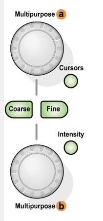
You can undo any mapping by right-clicking the multipurpose knob(s) and selecting Deassign Multipurpose Knobs, or from the Utilities menu, select the Deassign Multipurpose Knobs command. The mapping is deassigned until you perform that function again.
