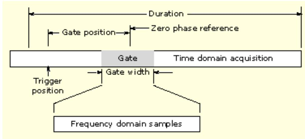
The gate must reside within the duration interval of the source waveform. If the source waveform duration is adjusted, and the gate position and width would result in the gate being outside of that duration, then the gate position or width is set within the limits.
