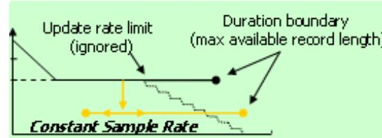
**TIP.** You can use the front panel Horizontal Resolution knob to change the sample rate in Constant Sample Mode.
