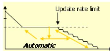
**Constant Sample Rate.** Use this mode to set the Sample Rate and Scale; the record length is a dependent variable. For  $\geq 4$  GHz instrument models, the default sample rate supports bandwidth filter operation. The maximum record length for your instrument depends on instrument model and record length option.
