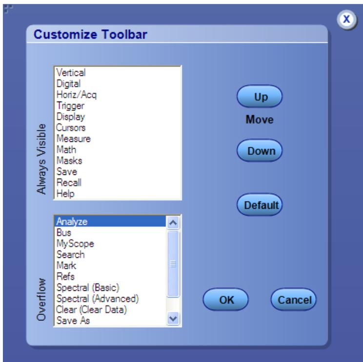
To access some of the less common controls, click the [Menu Bar Mode \(see page 33\)](#). To do this, click the Menu button (with the arrow) in the upper-right corner of the screen and select Customize to display the Customize Toolbar dialog box.
