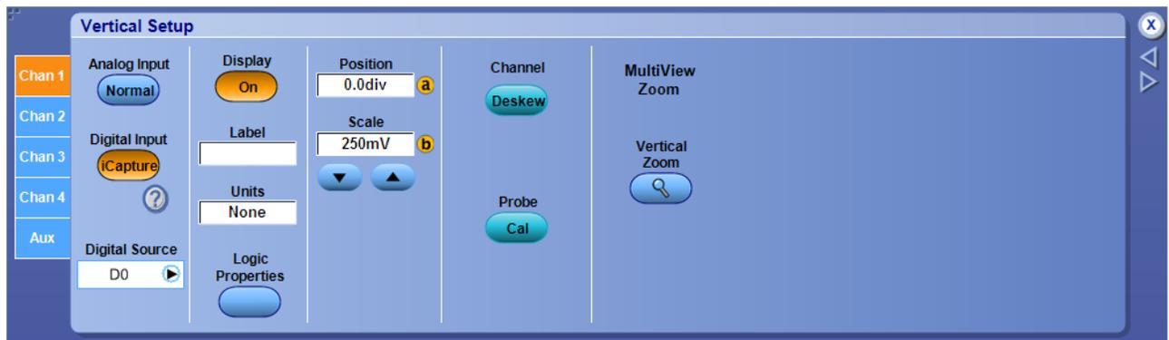
**NOTE.** Right-click on the digital source readout in the waveform window to reroute from one analog channel to any of the other three analog channels. For example, right-click on D0 captured on Ch1 and select **iCapture on Ch2** to reroute the source D0 to Ch2.
