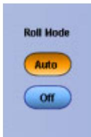
Roll mode lets you see acquired data without waiting for the acquisition of a complete waveform record. It gives you immediate feedback. For slow time base settings, Roll mode provides a rolling display similar to a strip-chart recorder.
