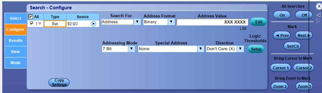
Select the Address Format, Addressing Mode, special Address, and Direction from the drop-down lists. Click Edit to enter the address value. Click Setup to adjust the logic thresholds.
