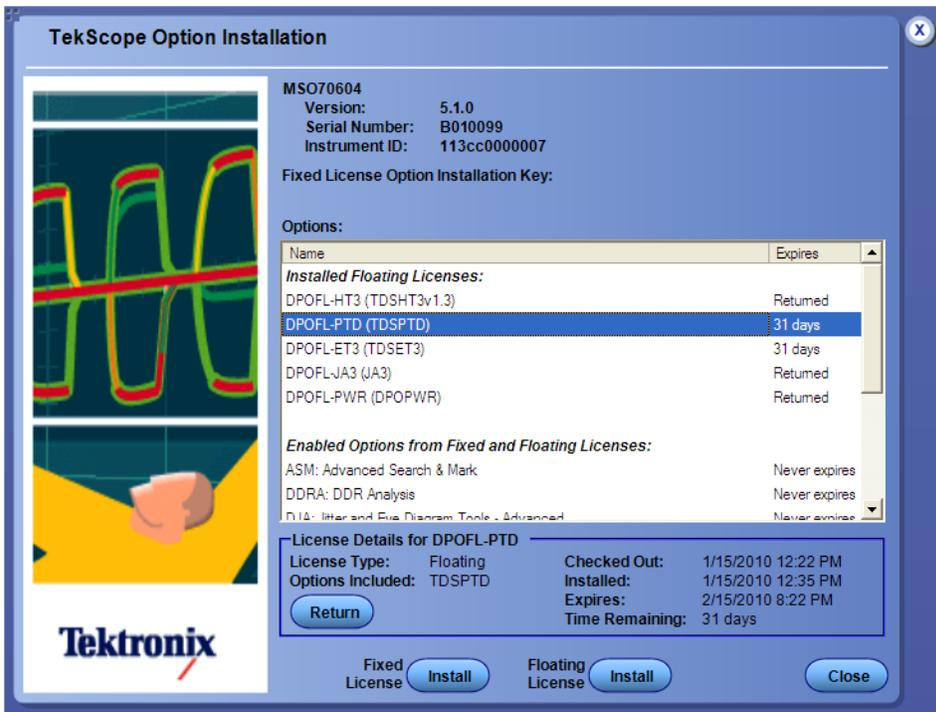
3. Select the Option (for example DPOFL-PTD (TDSPTD)) in the Tekscope Option Installation dialog box and click the Return button (when the license is still valid) or click Exit Key button (when the license has expired).
