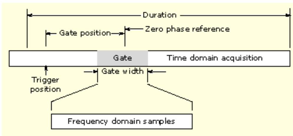
The gate must reside within the duration interval of the source waveform. If the source waveform duration is adjusted, and the gate position and width would result in the gate being outside of that duration, then the gate position or width is set within the limits.
