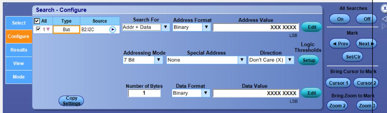
Select the Address Format, Addressing Mode, special Address, Direction, and Data Format from the drop-down lists. Click Edit to enter the address and data values. Click Setup to adjust the logic thresholds.
