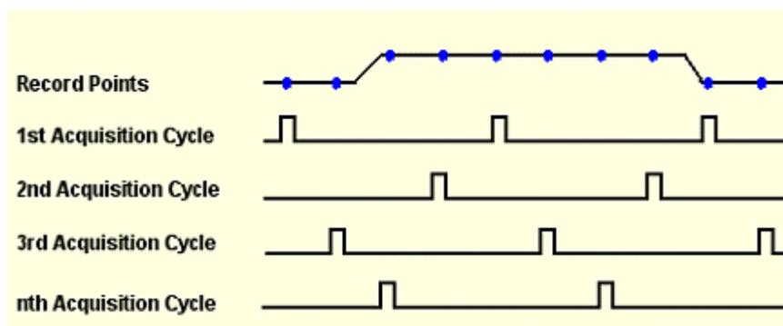
The sampling speeds and the number of channels you choose affect the mode the instrument uses to sample waveforms. The instrument always uses real-time sampling at slower time base settings; faster time settings force the instrument to switch from real-time sampling to equivalent-time sampling.
