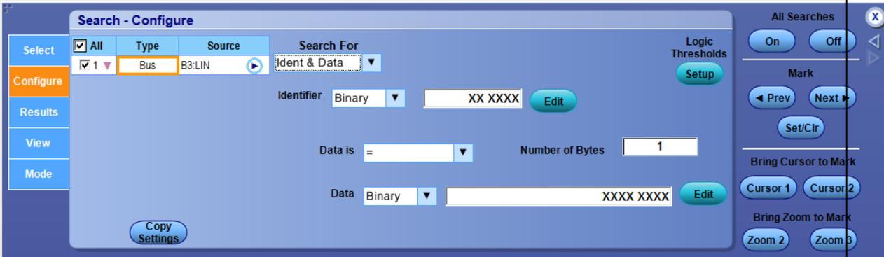
The screenshot shows the 'Search - Configure' dialog box. The 'Search For' dropdown is now set to 'Ident & Data'. The 'Identifier' field remains 'Binary' with 'XX XXXX'. Below it, 'Data is' is set to '=' and 'Number of Bytes' is '1'. The 'Data' field is set to 'Binary' and contains 'XXXX XXXX'. An 'Edit' button is next to the field. A 'Copy Settings' button is at the bottom left. The right-hand side controls are the same as in the previous screenshot.
