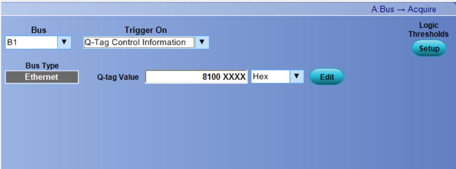
The screenshot shows a configuration window titled "A:Bus → Acquire". It features a "Bus" dropdown menu set to "B1" and a "Trigger On" dropdown menu set to "Q-Tag Control Information". To the right, there is a "Logic Thresholds" section with a "Setup" button. Below the "Trigger On" menu, the "Bus Type" is set to "Ethernet". There is one row of input fields: "Q-tag Value" containing the text "8100 XXXX" and a "Hex" dropdown menu. An "Edit" button is located to the right of the input field.
