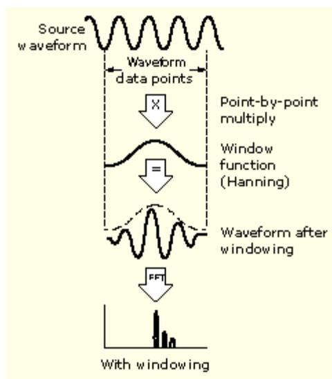
The window functions affect the ability to resolve frequency in the output spectrum and can affect the accuracy of the magnitude and phase measurements. The previous figure shows how the time domain record is processed.
