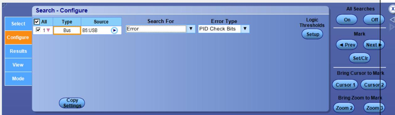
Select the Error Type from the drop-down list. Click Setup to adjust the logic thresholds.
