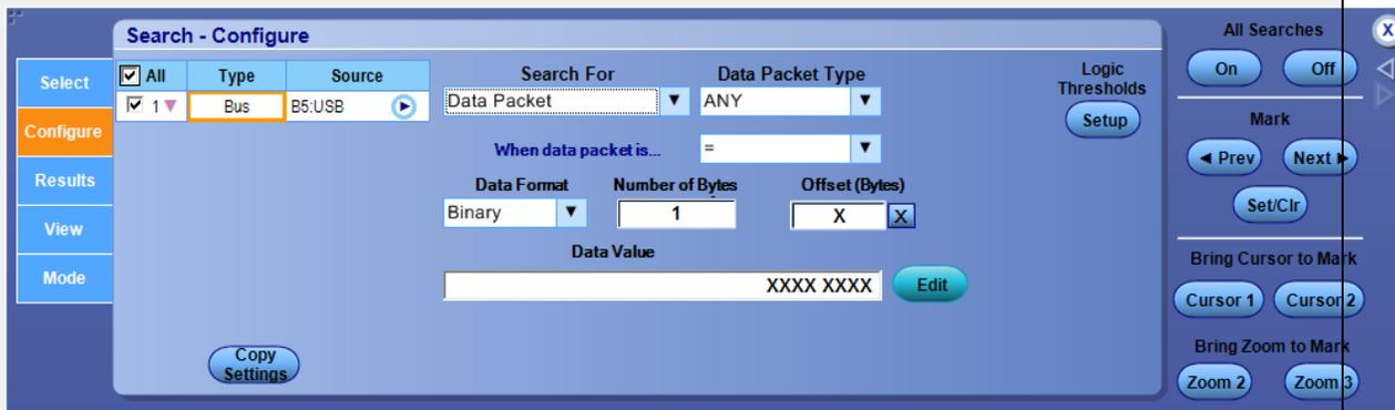
Select the Data Packet Type, When data packet is, Data Format, and Offset from the drop-down lists. Click Edit to enter the data value. Click Setup to adjust the logic thresholds.
