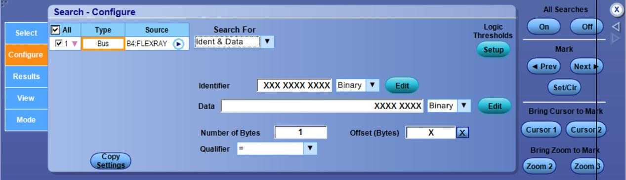
Select the Identifier from the drop-down list. Click Edit to enter the data values. Click Logic Thresholds to adjust the logic thresholds.
