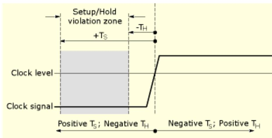
Setup/hold triggering uses the setup/hold violation zone to detect when data is unstable too near the time it is clocked. Each time trigger holdoff ends, the instrument monitors the data and clock sources. When a clock edge occurs, the instrument checks the data stream it is processing (from the data source) for transitions occurring within the setup/hold violation zone. If any occur, the instrument triggers with the trigger point located at the clock edge.
