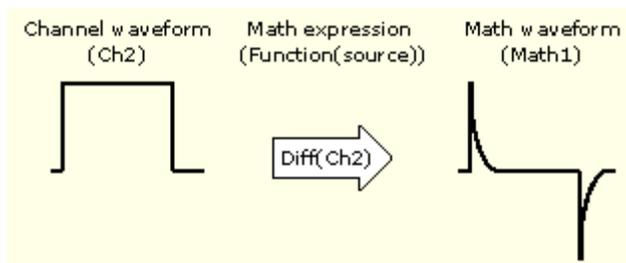
You create math waveforms to support the analysis of your channel and reference waveforms. By combining and transforming source waveforms and other data into math waveforms, you can derive the data view that your application requires. Create math waveforms that result from:
