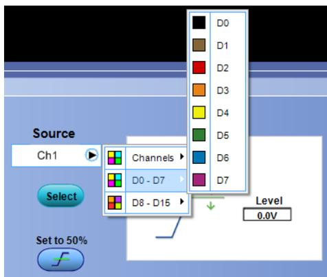
If your instrument has digital channels, trigger on a digital channel by selecting a digital channel.
