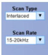
The Scan Rate enables you to trigger on nonbroadcast video signals that have unique scan rates. Select the scan rate range that includes your signal: 15-20 kHz, 20-25 kHz, 25-35 kHz, 35-50 kHz, or 50-65 kHz.
