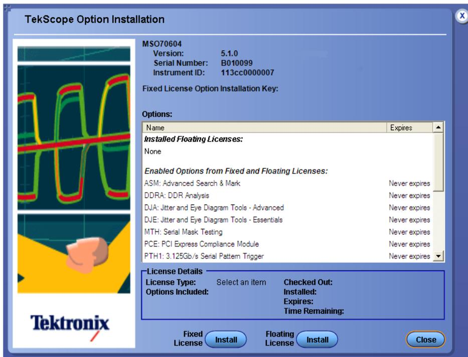
2. Enter the option installation key (provided by Tektronix) in the Options dialog box.
