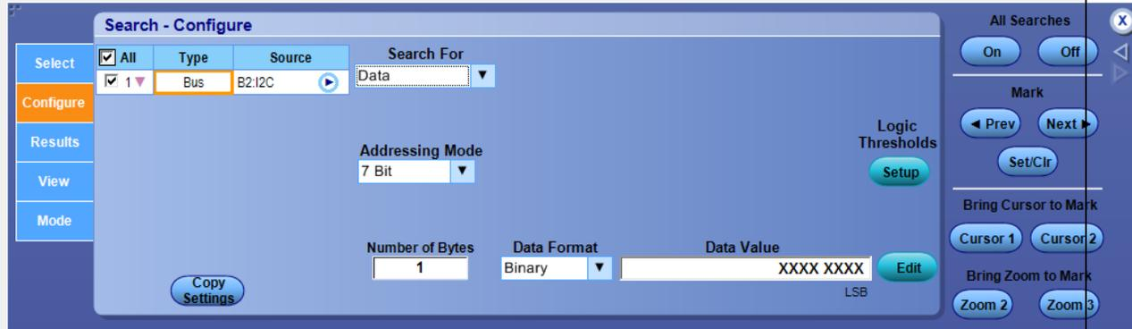
Select the Addressing Mode and Data Format from the drop-down lists. Click Edit to enter the data value. Click Setup to adjust the logic thresholds.
