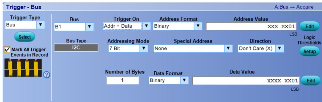
In DPO7000C and MSO70000C/DX Series instruments, when you trigger on an Address for I2C serial bus, there are some predefined patterns termed as Special Addresses. Use this information to debug your serial bus. The following table lists the predefined patterns along with their names.
