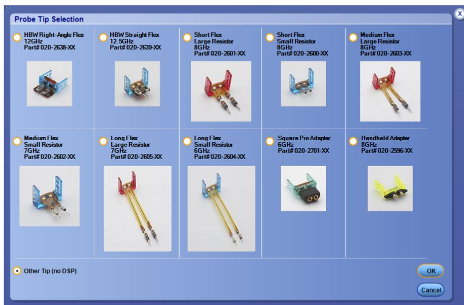
Here is an example of Probe Tip for Tektronix Trimode probe.
