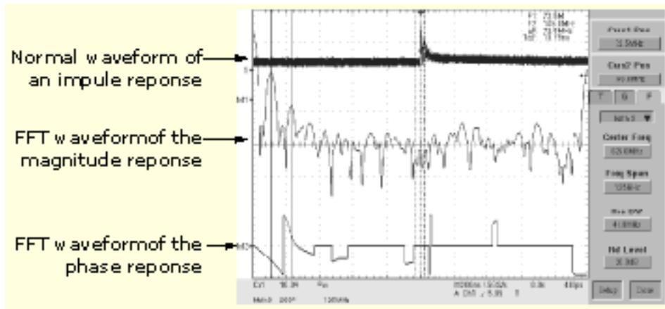
This instrument supports mathematical combination and functional transformations of waveforms it acquires. The next figure shows this concept:
