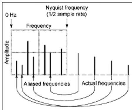
If you have a variable-frequency signal source, another way to observe aliasing is to adjust the frequency slowly while watching the spectral display. If some of the harmonics are aliased, you will see the harmonics decreasing in frequency when they should be increasing or vice versa.
