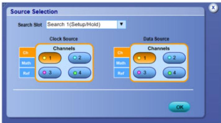
Use the Logic Source Selection window to set the threshold parameters for a Pattern or State logic search.
