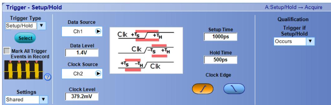
The following Trigger Setup/Hold screen appears on MSO/DPO5000B Series instruments:
