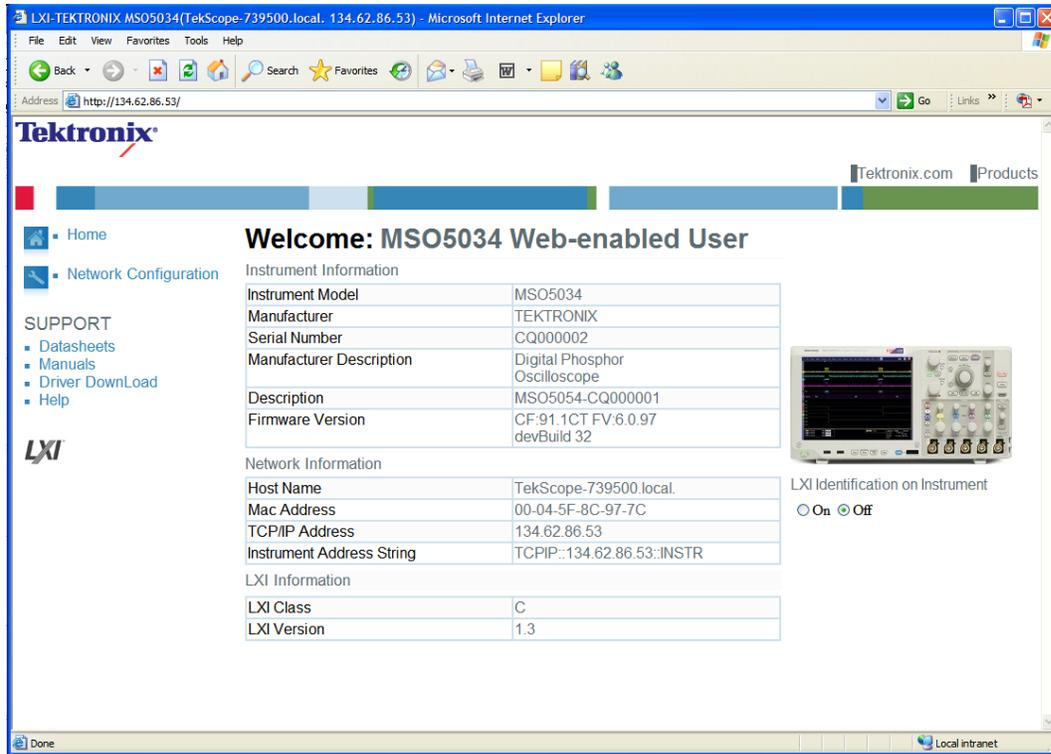
To display network configuration information, click on Network Configuration. The Web page displays the network configuration, and allows you to submit changes to some of the instrument configuration. Click on the Help SUPPORT link to see help on the configuration information.
