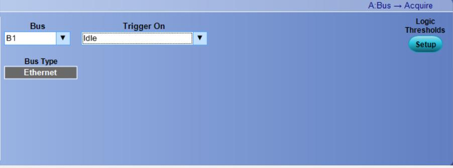
The screenshot shows a configuration window titled "A:Bus → Acquire". It has a "Bus" dropdown set to "B1" and a "Trigger On" dropdown set to "Idle". Below this is a "Bus Type" section with a button labeled "Ethernet". In the top right corner, there are "Logic Thresholds" and "Setup" buttons.
