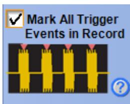
6. The instrument searches for and marks all similar events that meet the trigger requirements. The results of the search are shown as marked events on screen, and they can also be viewed in the Results tab of the Mark Table.
