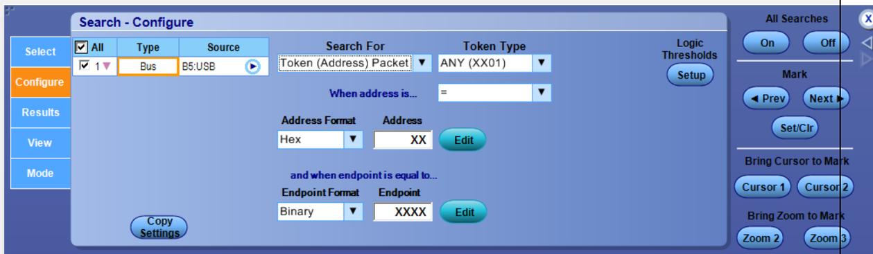
Select the Token Type, Address Format, When address is, and Endpoint Format from the drop-down lists. Click Edit to enter the address and endpoint values. Click Setup to adjust the logic thresholds.
