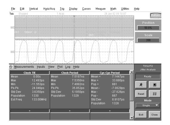
Figure 6: Jitter analysis demonstrations
