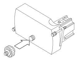
Figure 3: Storing the adapter
