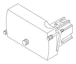
Figure 1: O/E Electrical Out-to-CH1 input adapter (013-0327-xx)
