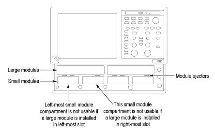
Figure 1: Module compartments
