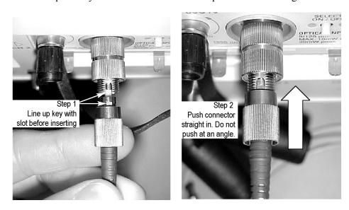
Figure 2: Connecting optical cables correctly
