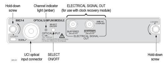
Figure 3: 80C14 optical module front panel
