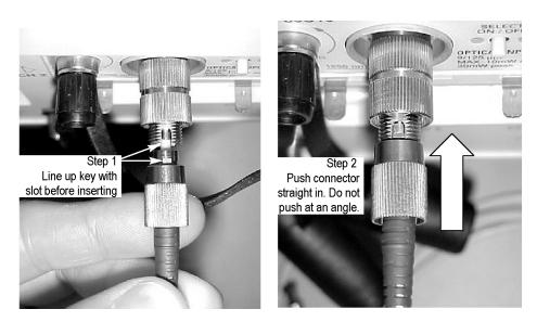
Figure 2: Connecting optical cables correctly
