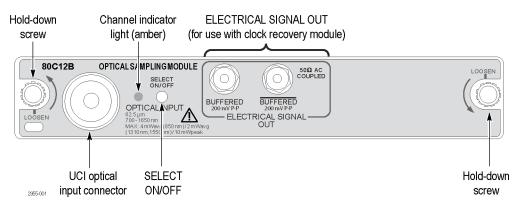
Figure 3: 80C12B optical module front panel
