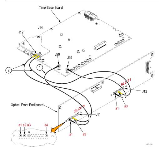
Figure 5-9: Optical front end cables
