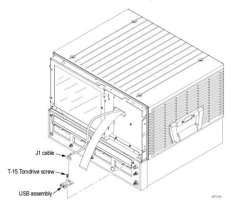
Figure 4-8: USB assembly removal
