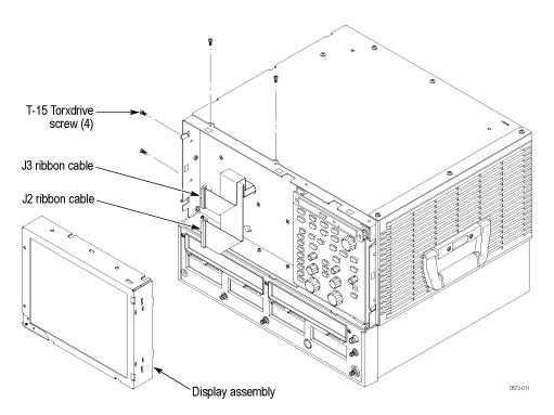
Figure 4-5: Display assembly removal
