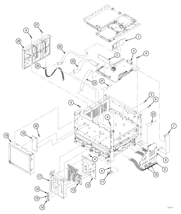
Figure 5-3: Front panel and processors
