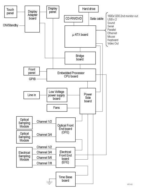
Figure 2-1: DSA8300 block diagram
