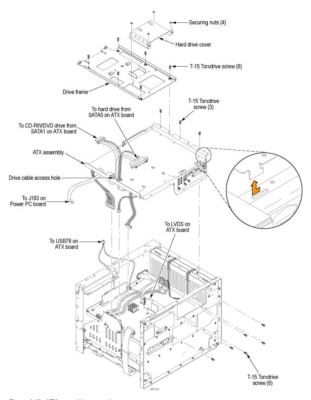
Figure 4-13: ATX assembly removal
