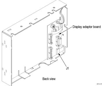
Figure 4-7: Display adaptor board replacement
