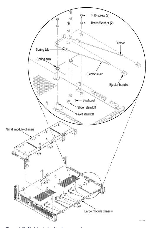
Figure 4-19: Module ejector handles removal
