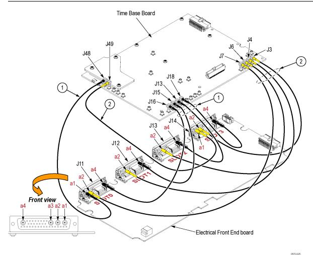
Figure 5-8: Electrical front end cables
