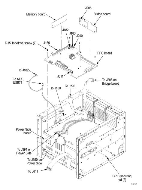
Figure 4-14: Power PC board removal
