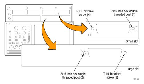
Figure 4-17: T-10 screws and threaded posts
