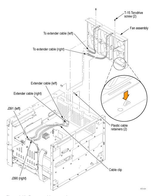
Figure 4-15: Fan assembly removal
