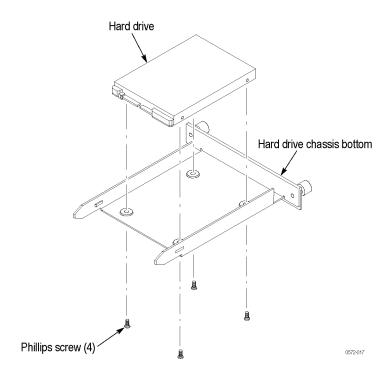
Figure 4-9: Hard disk drive removal
