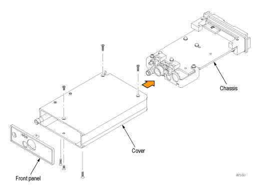
Figure 4-21: Sample of electrical module hardware removal
