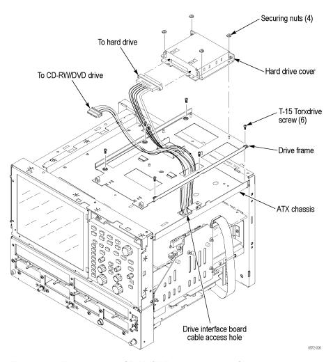
Figure 4-12: Hard drive and CD-RW/DVD drive mounting frame removal
