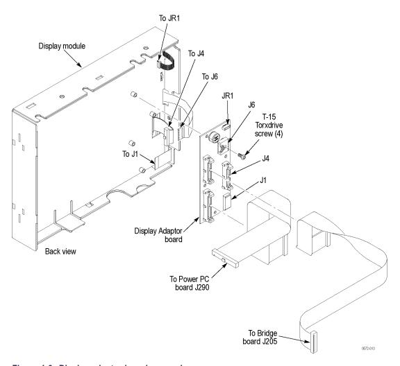
Figure 4-6: Display adaptor board removal
