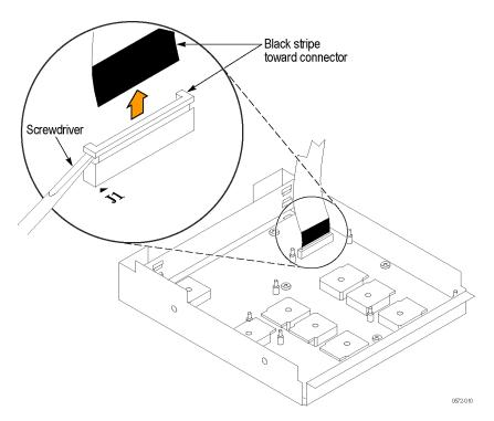
Figure 4-4: J1 flex cable connector removal
