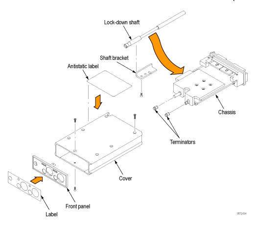
Figure 4-22: 80A00 and 82A00 series parts removal (80A01 shown)
