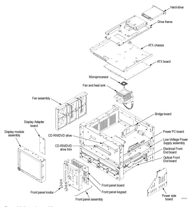
Figure 4-3: Internal assemblies
