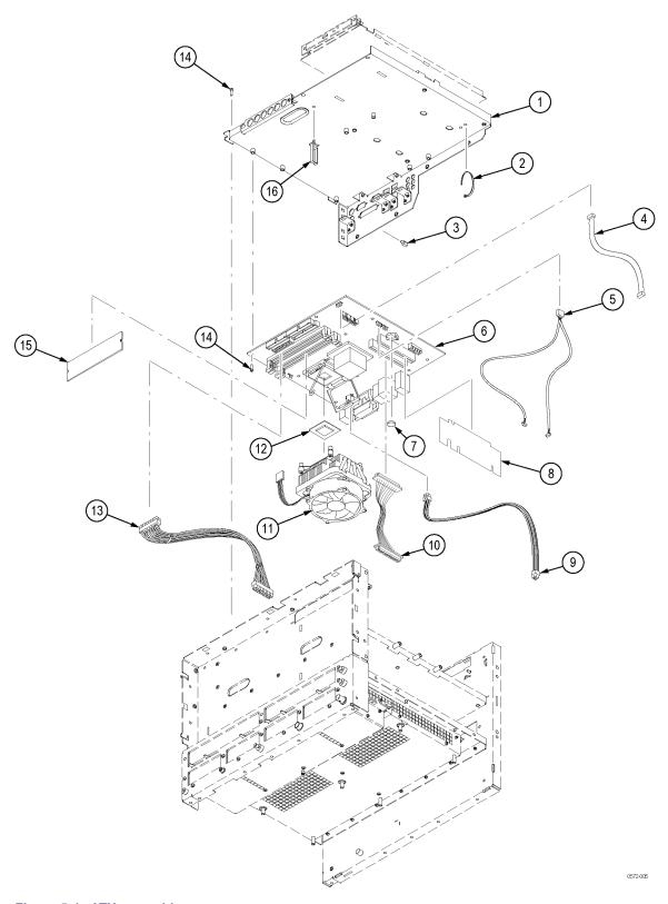
Figure 5-4: ATX assembly
