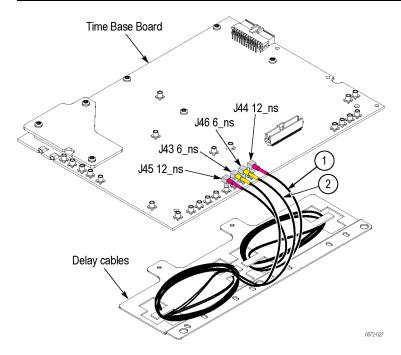
Figure 5-7: Time base delay cables
