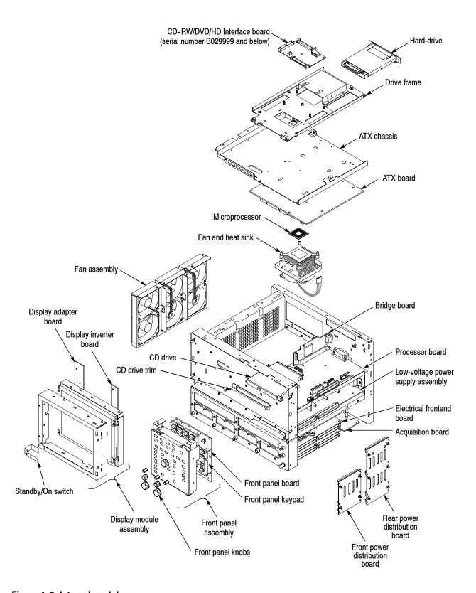
Figure 4-8: Internal modules
