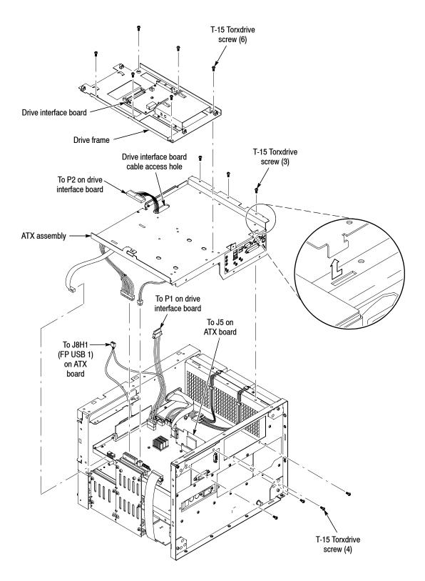
Figure 4-28: ATX assembly removal (serial number B029999 and below)
