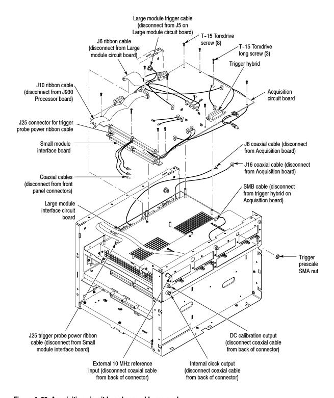
Figure 4-39: Acquisition circuit board assembly removal
