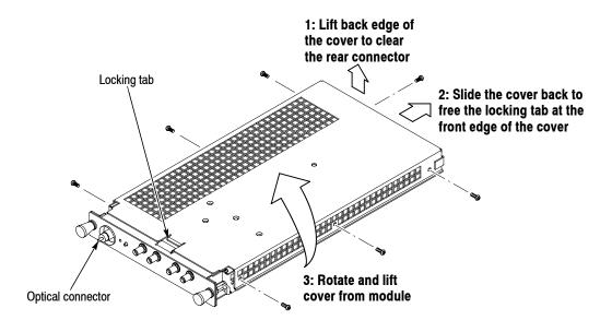
Figure 4-47: Optical module cover removal
