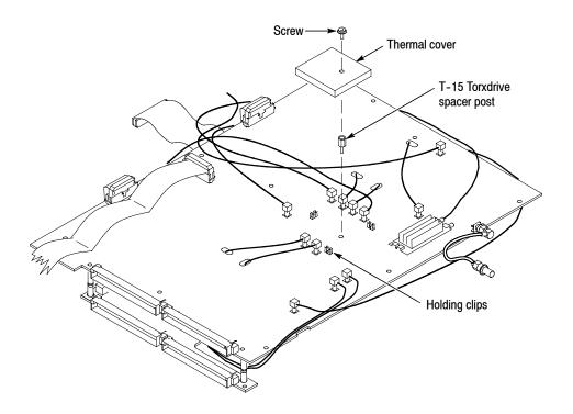
Figure 4-38: Thermal cover removal
