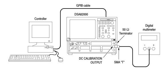
Figure 3-1: Adjustment setup using the DMM
