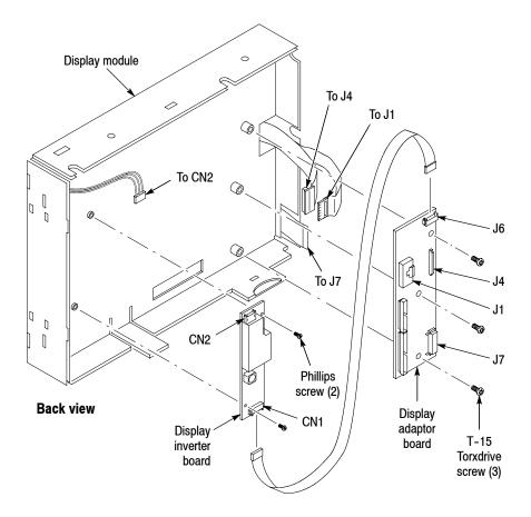
Figure 4-15: Display adaptor board removal
