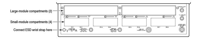
Figure 1-1: Compartments for sampling modules
