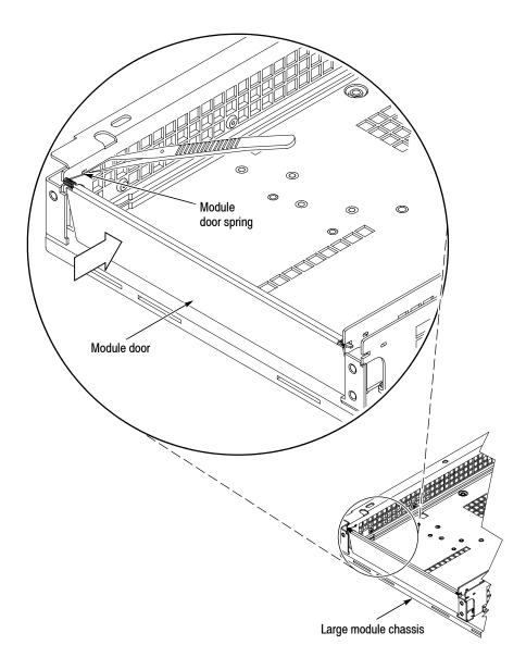
Figure 4-42: Module door spring removal
