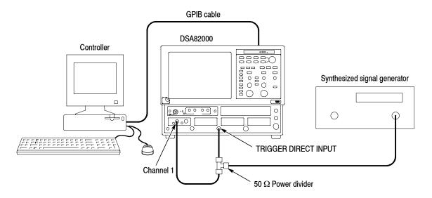
Figure 3-2: Adjustment setup using the signal generator
