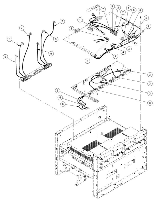
Figure 6-9: Coaxial cables
