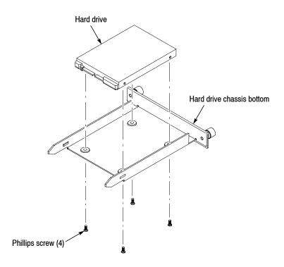
Figure 4-21: Removing the hard disk drive from the cartridge (serial number B030000 and above)
