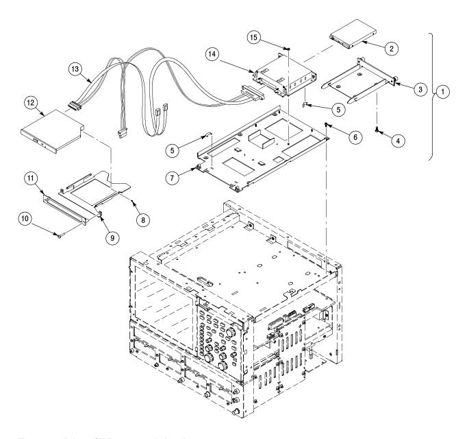
Figure 6-2: Drives (SN B030000 and above)
