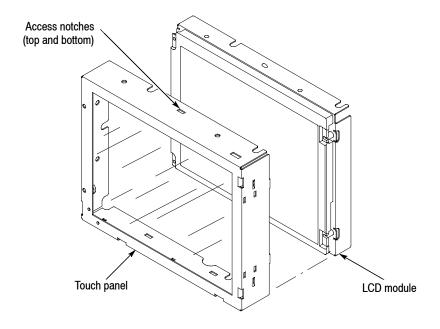
Figure 4-14: Touch panel and LCD assembly removal
