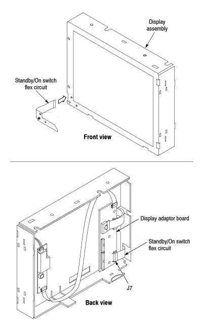
Figure 4-17: Standby/On switch flex circuit removal
