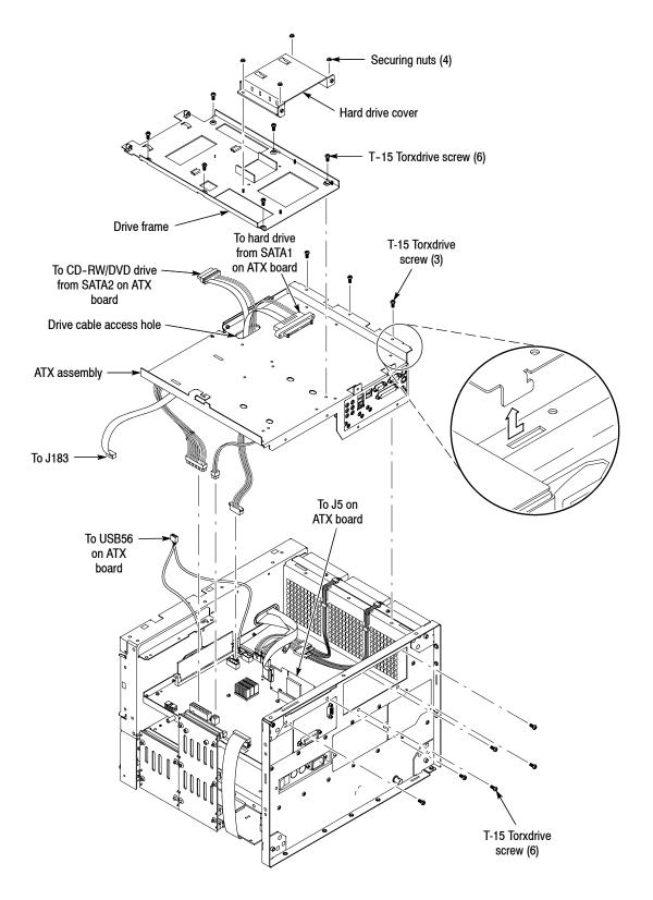
Figure 4-29: ATX assembly removal (serial number B030000 and above)
