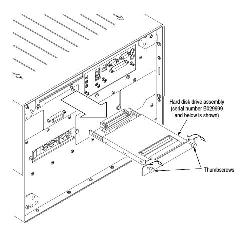
Figure 4-19: Hard drive disk removal
