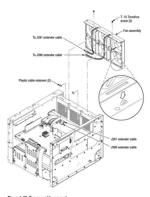
Figure 4-35: Fan assembly removal
