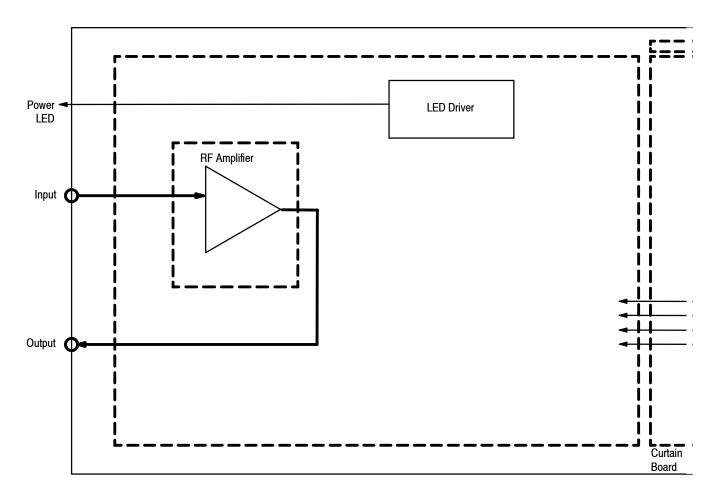
Figure 5-3: 80A01 block diagram
