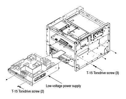
Figure 4-36: Low-voltage power supply removal
