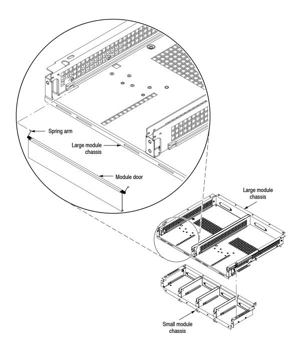
Figure 4-43: Module slot door removal
