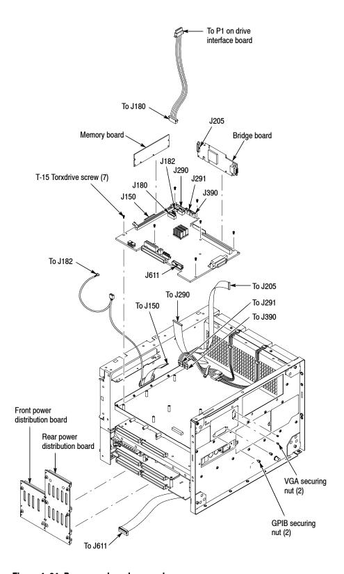
Figure 4-34: Processor board removal
