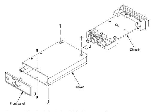
Figure 4-46: Sample of electrical module hardware removal
