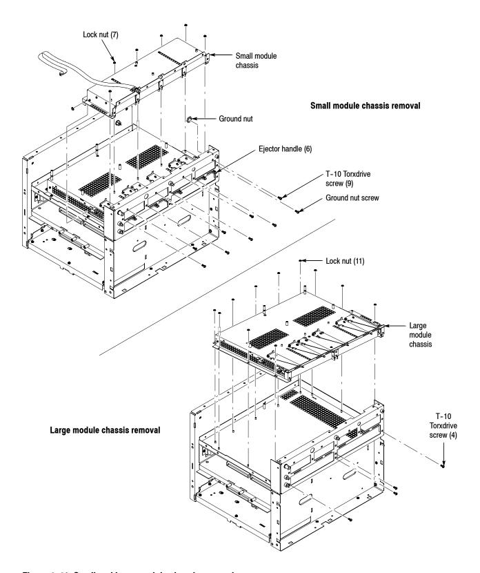
Figure 4-41: Small and large module chassis removal
