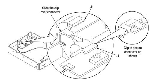
Figure 4-16: Connector clip assembly
