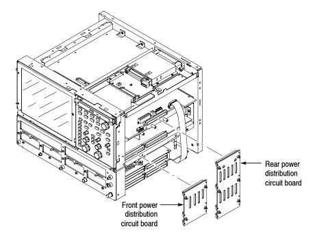
Figure 4-33: Front and rear power distribution board removal
