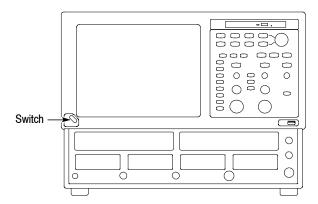
Figure 1-4: On/Standby switch location
