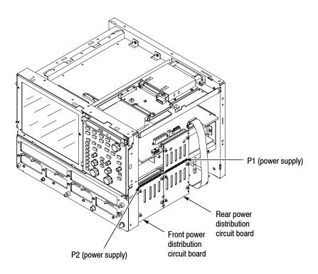
Figure 4-51: Connectors P1 and P2
