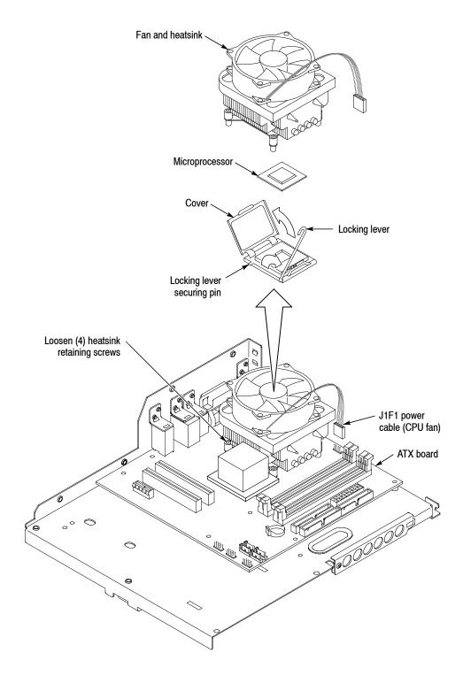
Figure 4-32: Microprocessor removal
