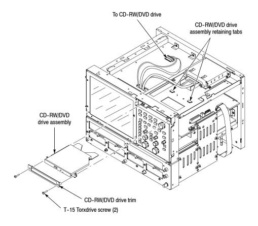
Figure 4-23: CD-RW/DVD disk drive removal (serial numbers B030000 and aove)
