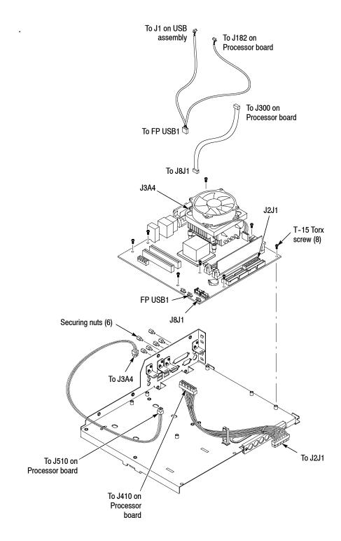
Figure 4-30: ATX board removal (serial number B029999 and below)
