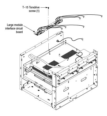
Figure 4-40: Large module interface circuit board removal
