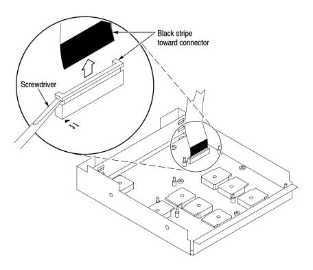
Figure 4-11: J1 flex cable connector removal
