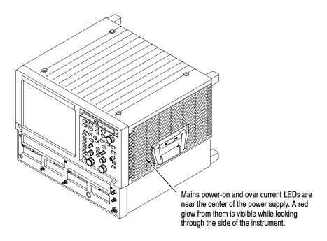
Figure 4-49: Location of power-on and over current LEDs
