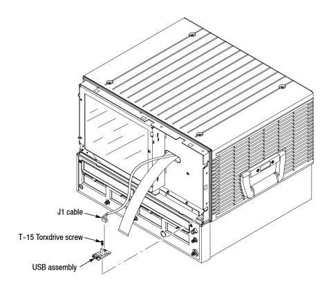
Figure 4-18: USB assembly removal
