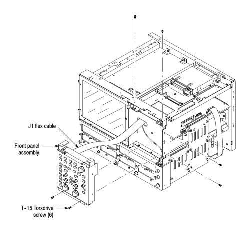
Figure 4-10: Front panel assembly removal
