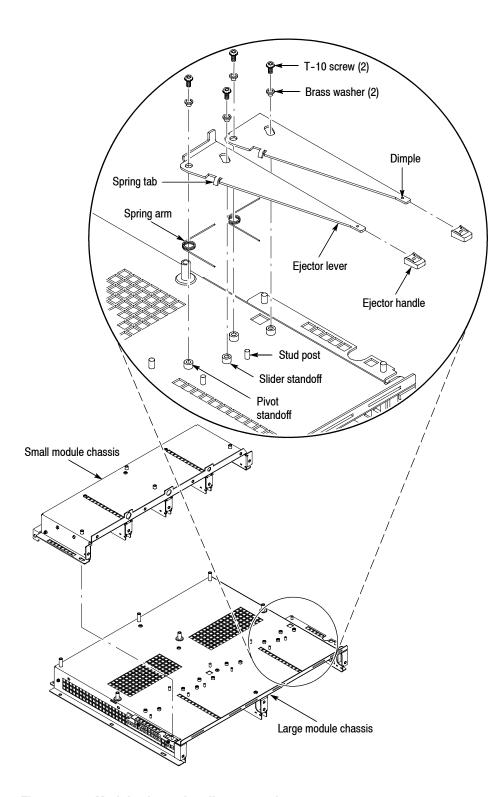
Figure 4-44: Module ejector handles removal
