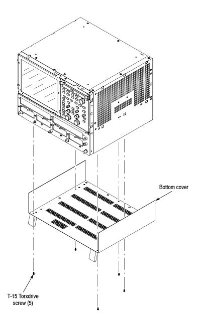
Figure 4-4: Bottom cover removal
