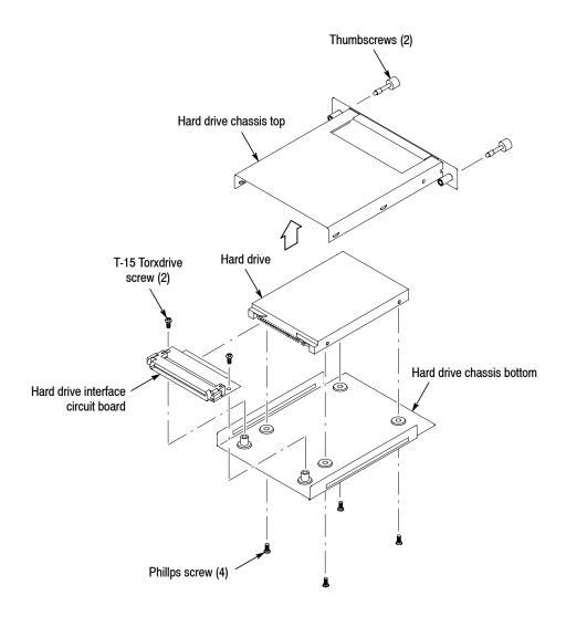
Figure 4-20: Removing the hard disk drive from the cartridge (serial number B029999 and below)
