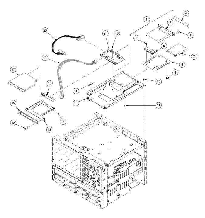
Figure 6-3: Drives (SN B029999 and below)
