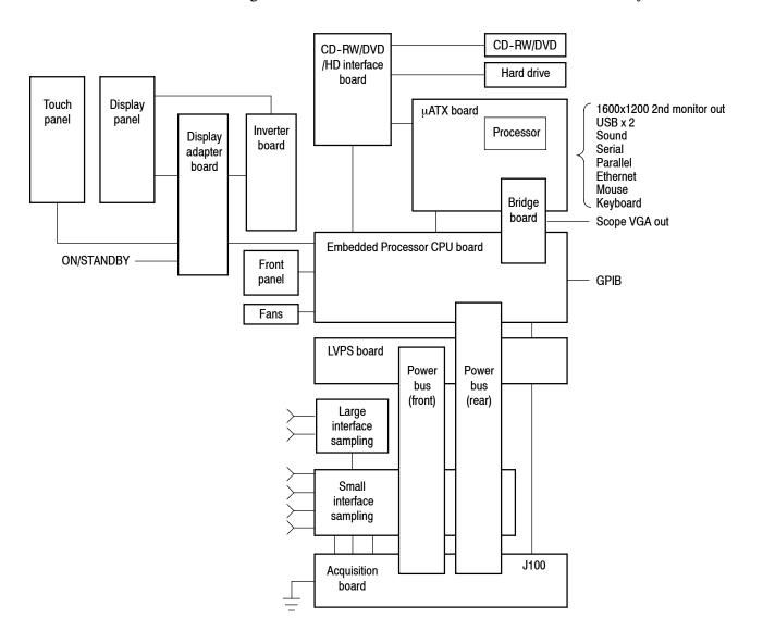
Figure 5-1: Block diagram for the DSA8200
