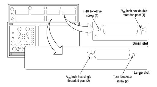
Figure 4-37: T-10 screws and threaded posts
