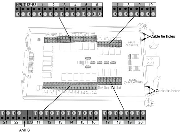
4. Route wire along the wire path and secure with cable tie as shown. The next figure also shows connections to channels 1 and 2.
