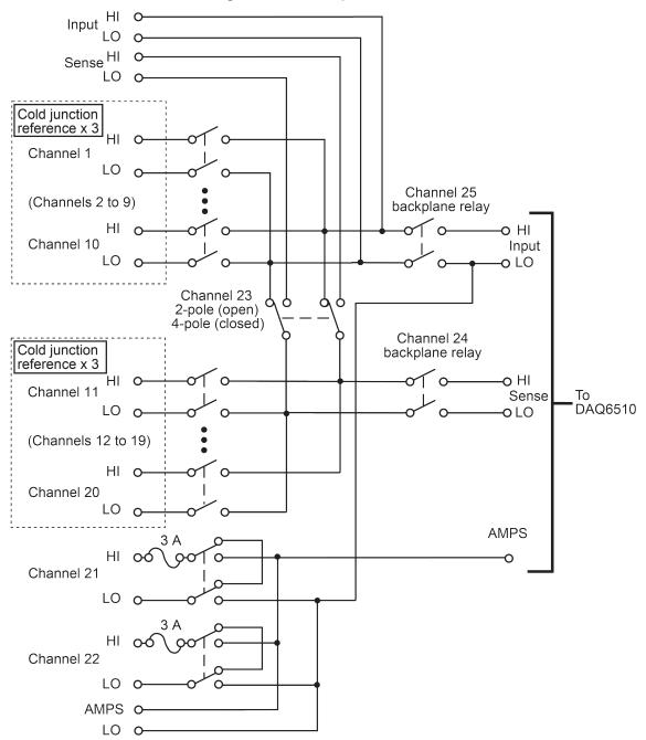
Figure 5: 7700 simplified schematic
