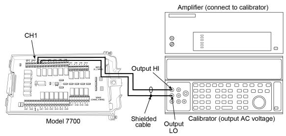
Figure 7: Connections for AC volts verification
