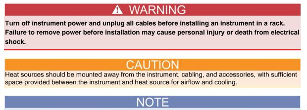
To prevent damaging heat build-up and ensure specified performance, make sure there is adequate ventilation and air flow around the instrument to ensure proper cooling. Do not cover the ventilation holes on the top, sides, or bottom of the instrument.
