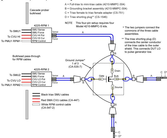
Figure 19: Test setup for four-terminal C-V testing
