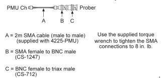
Figure 16: Basic four-pin prober setup for PMU
