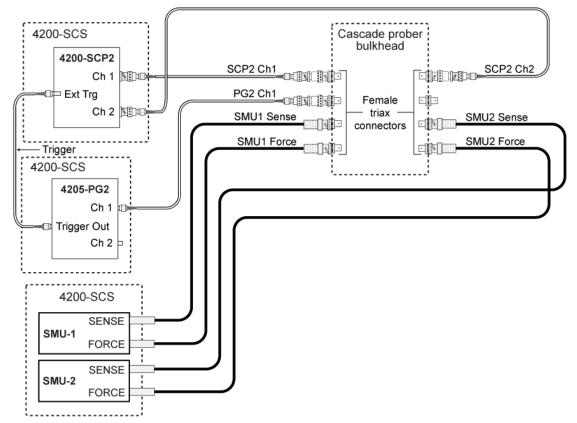
Figure 5: Cables and adapters used for instrumentation connections
