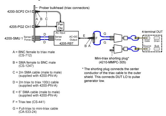
Figure 13: Connections to the drain and bulk
