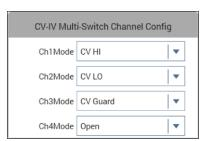
If using 2-wire sense, connect a single triaxial cable to the force output connectors of channels 1, 2, and 3 of the 4200A-CVIV to the device under test. If using 4-wire sense, connect two triaxial cables to the force and sense output connectors of each channel and terminate them together at the device under test. See the next figure for an example of the internal switch configurations and device connections.
