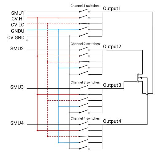
Figure 48: 4200A-CVIV connections to a 4-terminal MOSFET device for C-V characterization
