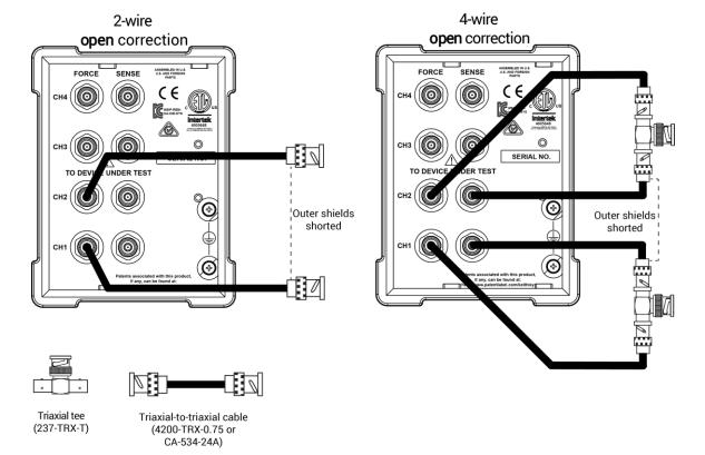
Figure 28: Connections for open connection compensation
