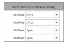
If using 2-wire sense, connect a single triaxial cable to the force output connector of channels 1 and 2 of the 4200A-CVIV to the device under test. If using 4-wire sense, connect two triaxial cables to the force and sense output connectors of each channel and terminate them together at the device under test. See the next figure for an example of the internal switch configurations and device connections.
