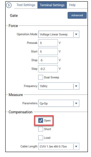
Figure 36: Enabling open compensation for the test
