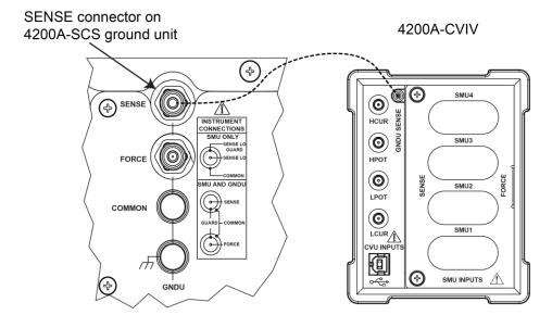
Figure 20: 4200A-CVIV GNDU switching configuration connection
