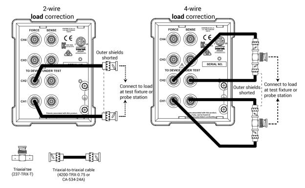
Figure 30: Connections for load connection compensation
