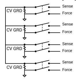
Figure 19: 4200A-CVIV CV GRD switching configuration
