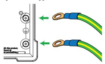
Figure 8: Connecting ground cables to the 4200A-CVIV
