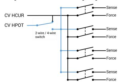
Figure 17: 4200A-CVIV CV HI switching configuration
