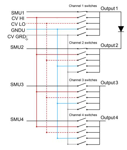
Figure 38: 4200A-CVIV connections to a 2-terminal device for I-V characterization
