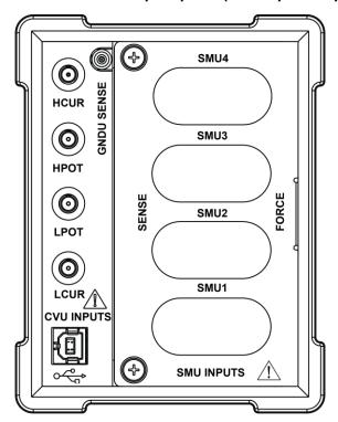
Figure 3: 4200A-CVIV inputs panel (SMU inputs empty)
