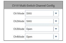
If using 2-wire sense, connect a single triaxial cable to the force output connectors of channels 1 and 2 of the 4200A-CVIV to the device under test. If using 4-wire sense, connect two triaxial cables to the force and sense output connectors of each channel and terminate them together at the device under test. See the next figure for an example of the internal switch configurations and device connections.
