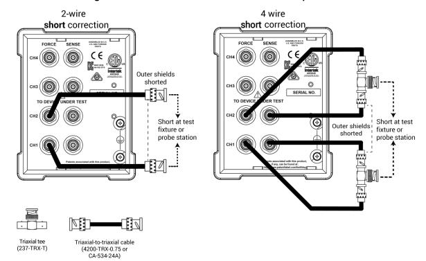
Figure 29: Connections for short connection compensation
