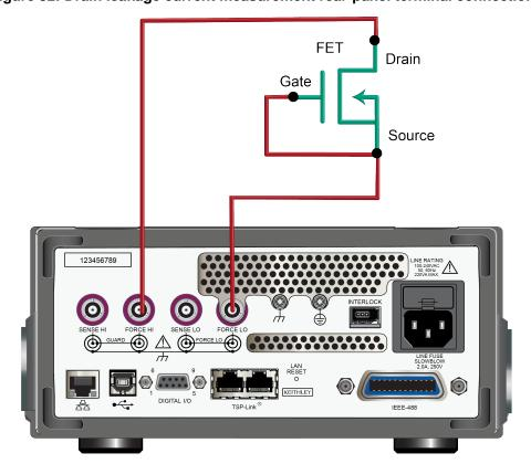
Figure 32: Drain leakage current measurement rear-panel terminal connections
