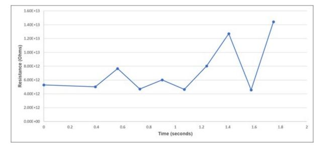
Figure 27: Insulation resistance test results
