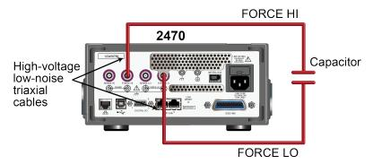
Figure 23: Rear-panel connections insulation resistance test
