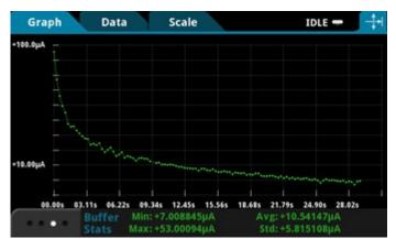
Figure 24: Front panel graph of leakage current measurement
