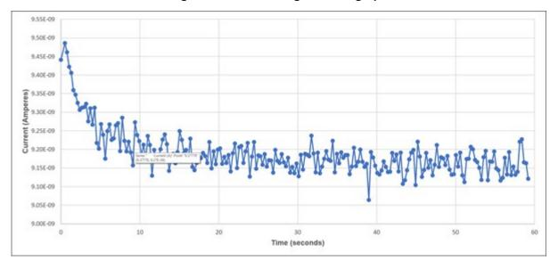
Figure 35: Drain leakage current graph
