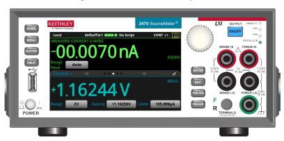
Figure 2: Model 2470 front panel
