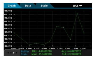
Figure 26: Insulation resistance graph
