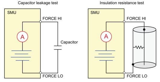
The following figures show the rear-terminal connections to the device under test (DUT) for these applications. If capacitor leakage measurements are noisy, you may need to use the high capacitance mode or add a low leakage forward-biased diode in series with the capacitor.
