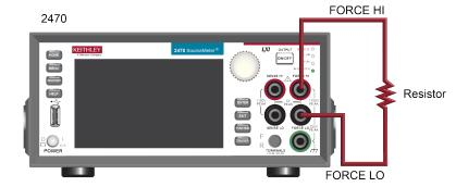
Figure 19: 2470 2-wire front-panel connections
