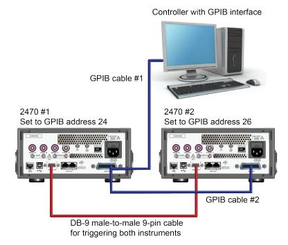
Figure 29: GPIB and DB-9 connections for the SCPI programming example
