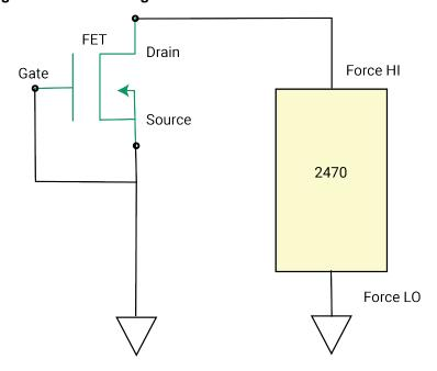
Figure 31: Drain leakage current measurement device connections
