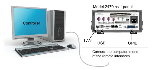
Figure 28: Model 2470 remote interface connections
