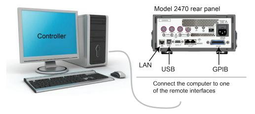
Figure 20: Model 2470 remote interface connections
