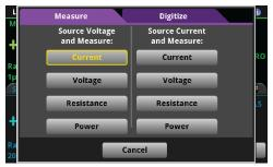
The instrument saves many of the commands with the source or measure function that was active when you set them. For example, if you set the measure function to current and you set a value for NPLCs, the instrument saves the NPLC value for that measure function. When you change the measure function to voltage, the NPLC value changes to the value that was last set for the voltage measure function.
