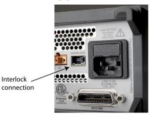
The interlock is intended for use through a normally open switch, which may be installed on the lid of a test fixture, on the enclosure of a semiconductor prober or device handler, or on the door or doors of a test equipment rack. The switch must be closed to enable the Model 2461 to produce voltages greater than  $\pm$  42 V.
