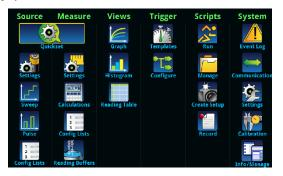
From this screen, you can select source, measure, graphing, trigger, scripting, and system setup menus. These menus allow you to choose options to set up your instrument to meet the needs of your applications.
