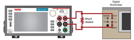
Figure 5: Front-panel connections for the 4 A to 10 A ranges
