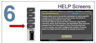
On the front panel, press the **HELP** key. The SMU has a context-sensitive help system to speed up your learning curve. When an icon or touchscreen button has focus (icon or button is highlighted with a yellow box), that feature or function has context-sensitive help. If there is no specific focus when you press the **HELP** key, overview information for the screen you are viewing displays.
