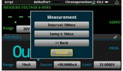
Change the measurement interval time to 500ms
