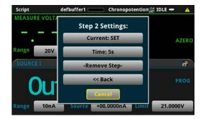
Add a second step to discharge the battery
