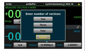
After the open circuit voltage is measured, the parameters of the potential sweep must be defined: Number of vertices, voltage magnitude, and reference voltage.
