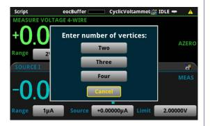
After the open circuit voltage is measured, the parameters of the potential sweep must be defined: Number of vertices, voltage magnitude, and reference voltage.
