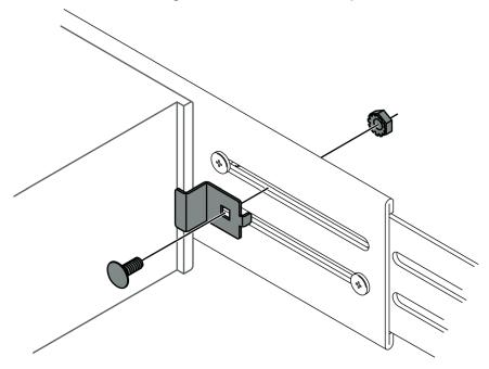
Figure 18: Install the unit clip
