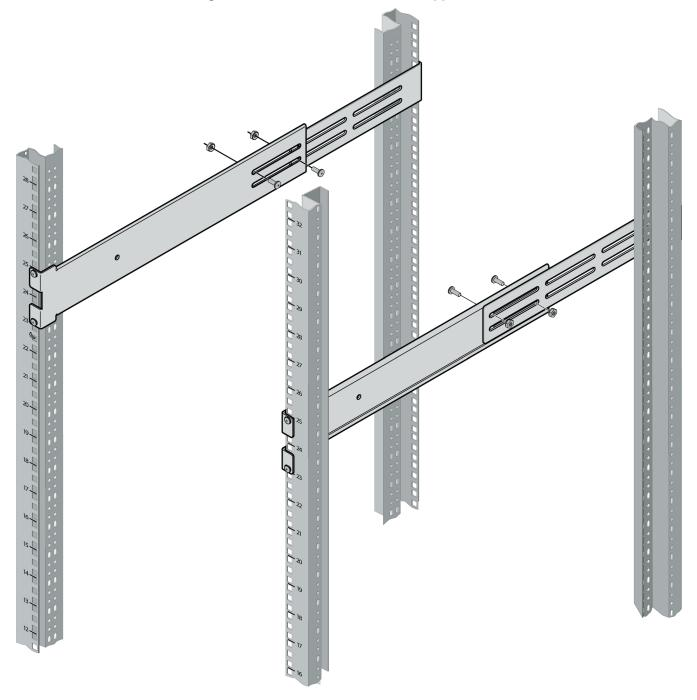
7. Install the U-bracket as shown in the following figure.
