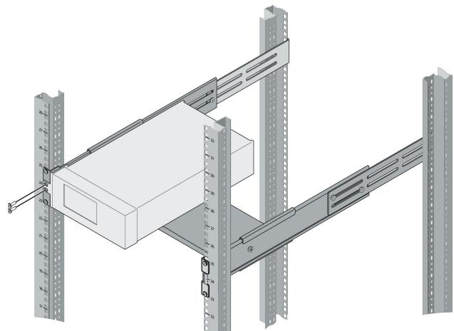
4. Secure the rear of the instrument to the support shelf with the unit clip, carriage bolt, and nut as shown in the following figure.
