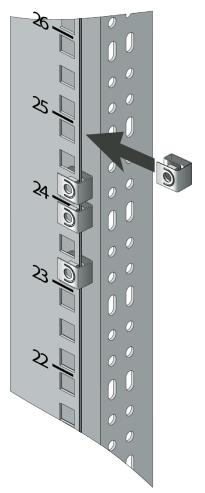
3. Install two cage nuts on each of the rear rails as shown in the following figure as shown in the following figure.
