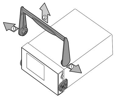
3. Remove the screws and the handle mounts from the instrument as shown in the following figure.
