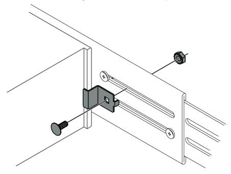
Figure 20: Install the unit clip
