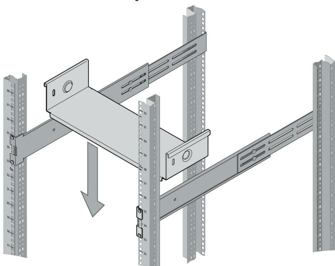
Figure 8: Install the U-bracket
